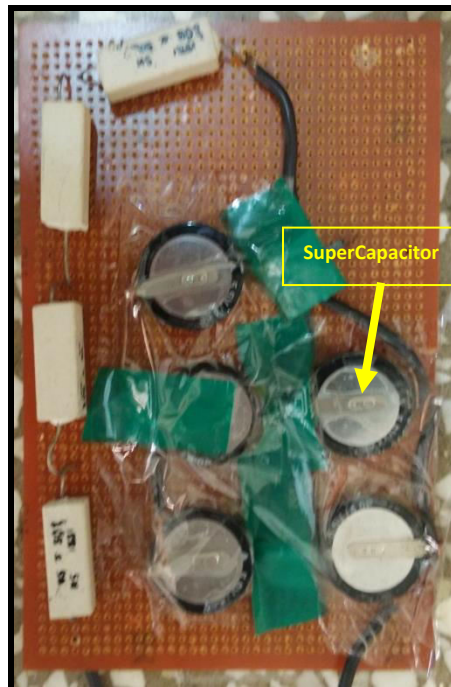
Photograph 6 SC Bank Sheet with Resistor & SUPER Capacitor.
