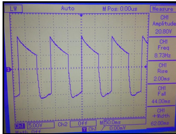
Photograph 17 Discharging of the R-C Bank Sheet parallel to Battery Bank
