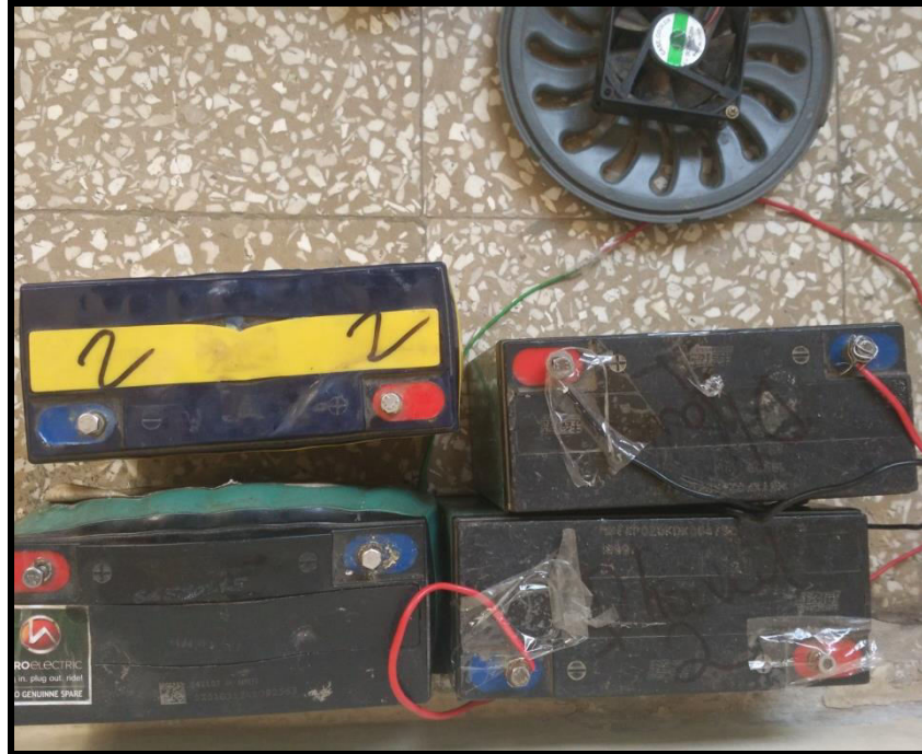
Photograph 7 Battery Bank of 48 V used for EV Testing.
