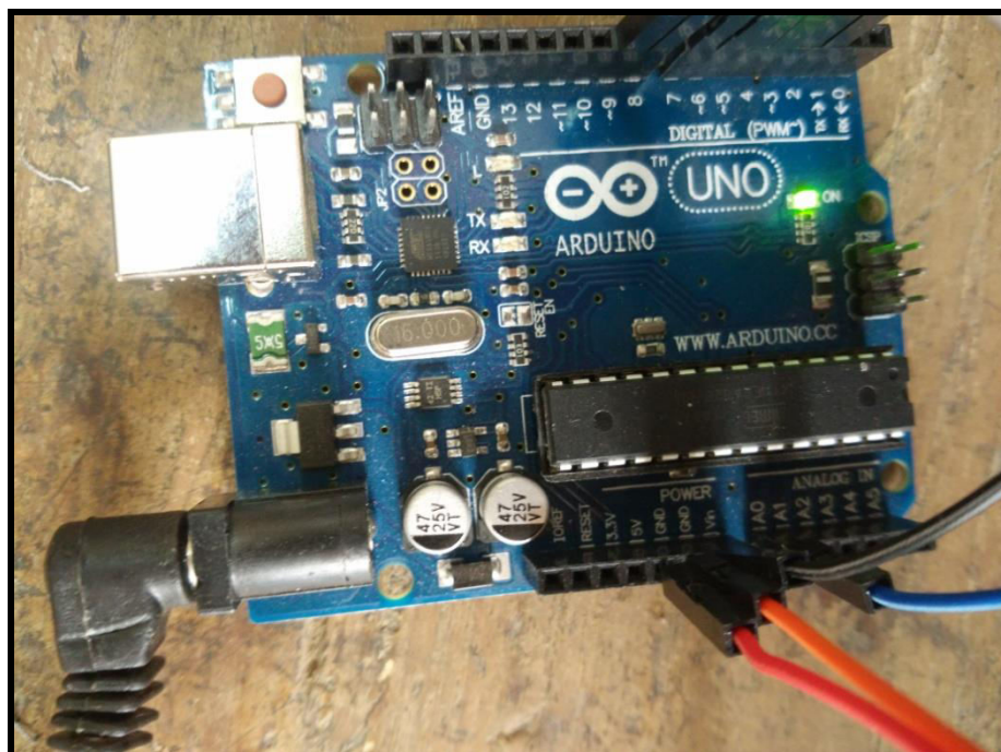
Photograph 2 Controller ARDUINO used for DST Programming
