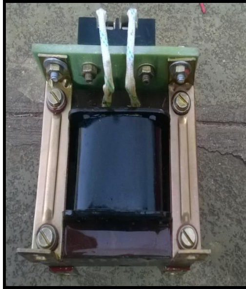
Photograph 23 The Inductor Designed.
