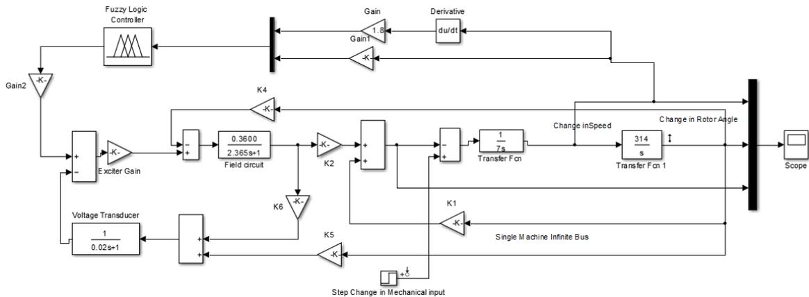
Fig. 4.16 Simulink model for 5% change in mechanical torque input With FPSS
