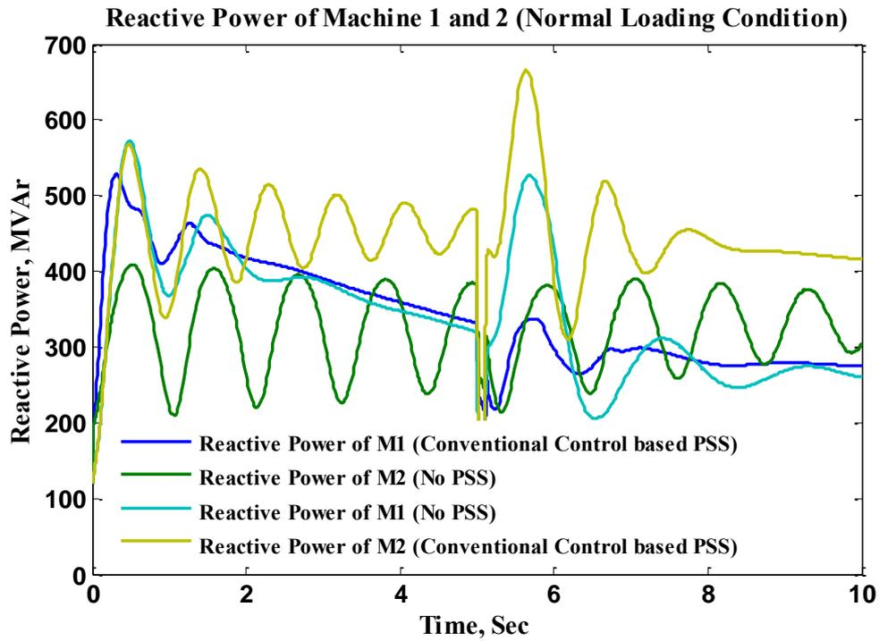
Fig. 4. 14 Reactive power performance of PSS installed in multimachine system for normal loading condition
