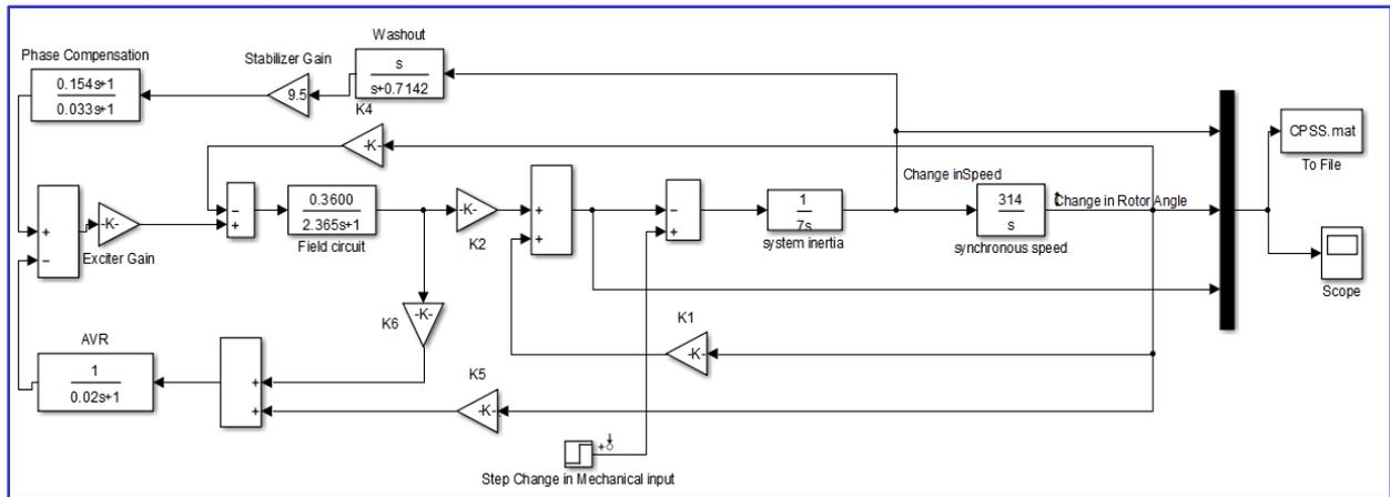
Fig. 4. 1 Simulink model for 5% change in mechanical torque input With CPSS
