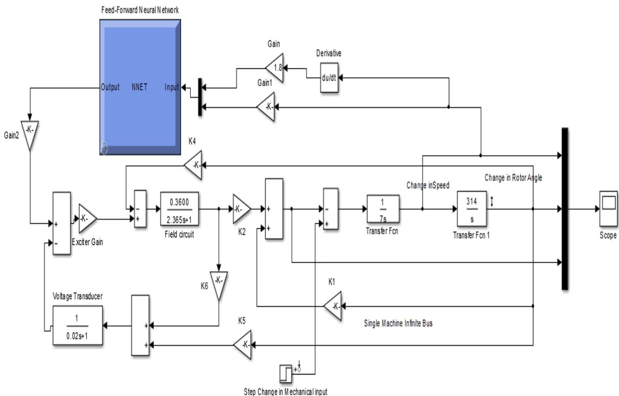
Fig. 4.18 Simulink model for 5% change in mechanical torque input With ANNPSS
