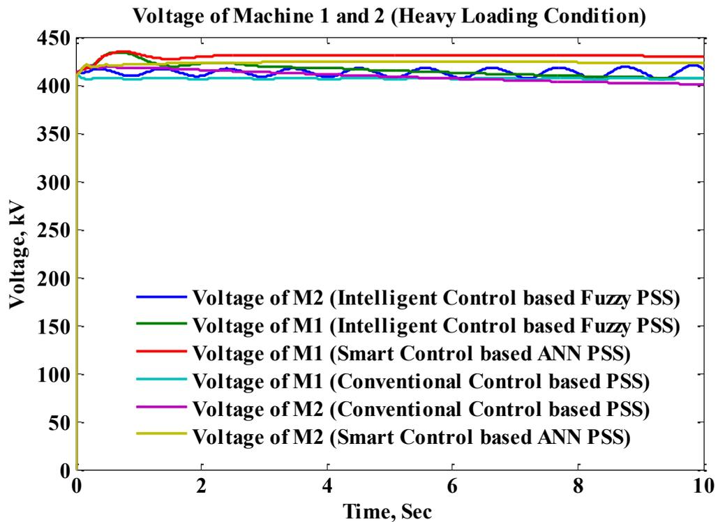
Fig. 4.25 Voltage comparisons for multimachine system (Heavy Loading Condition)
