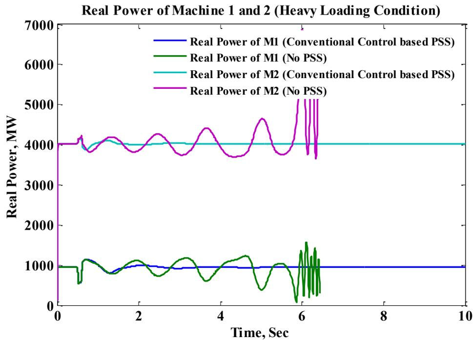
Fig. 4. 12 Real power performance of PSS installed in multimachine system for heavy loading condition
