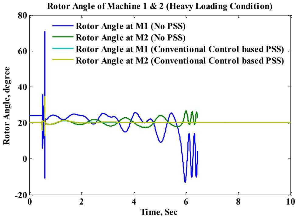
Fig. 4. 6 Rotor Angle Performance of PSS installed in multimachine system for heavy loading condition
