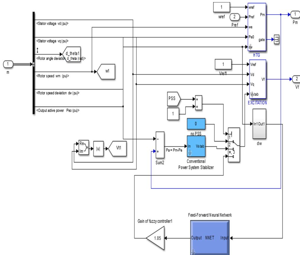
Fig. 4.19 Simulink model for Multimachine system with ANN PSS
