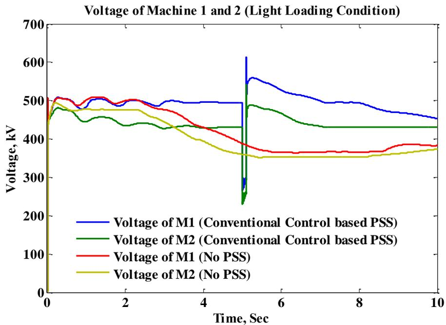
Fig. 4.7 Voltage performance of PSS installed in multimachine system for light loading condition
