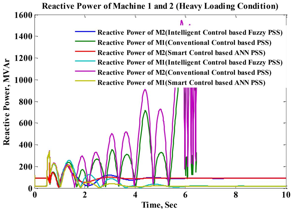
Fig. 4.31 Reactive power comparisons for multimachine system (Heavy Loading Condition)
