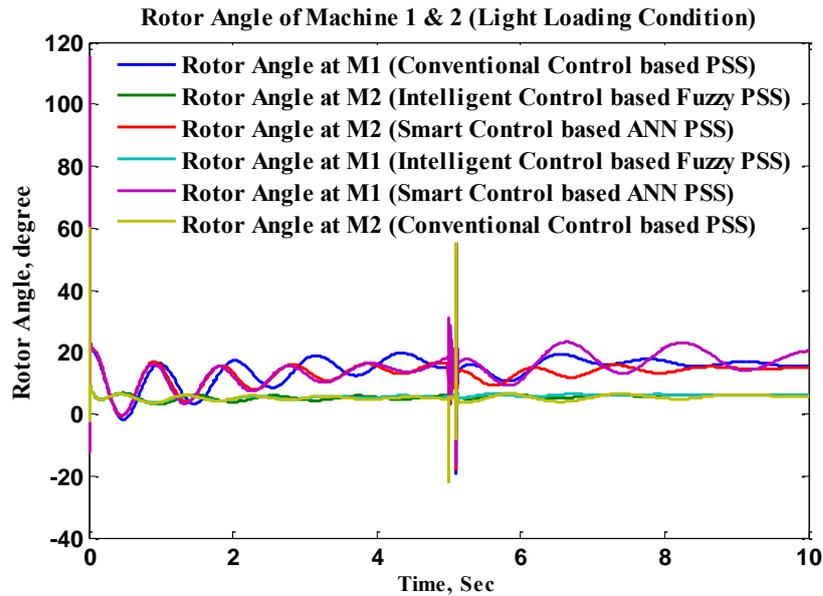
Fig. 4.20 Rotor angle comparisons for multimachine system (Light Loading Condition)
