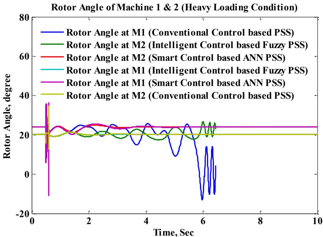
Fig. 4.22 Rotor angle comparisons for multimachine system (Heavy Loading Condition)
