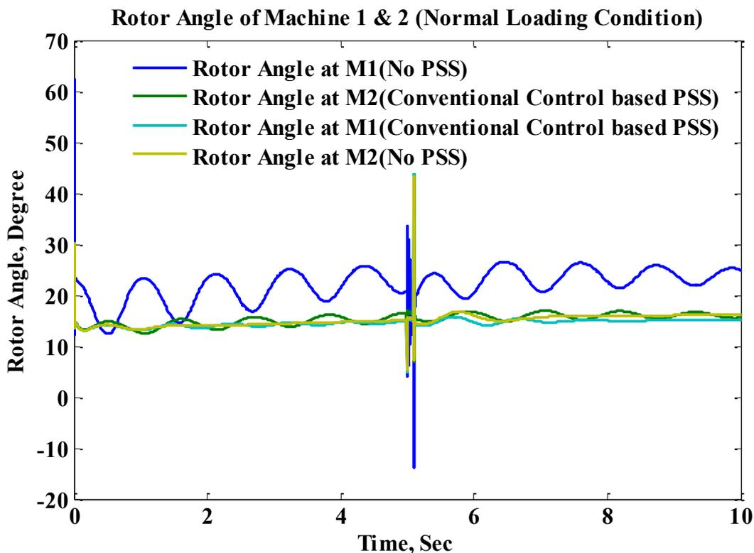
Fig. 4. 5 Rotor Angle Performance of PSS installed in multimachine system for normal loading condition
