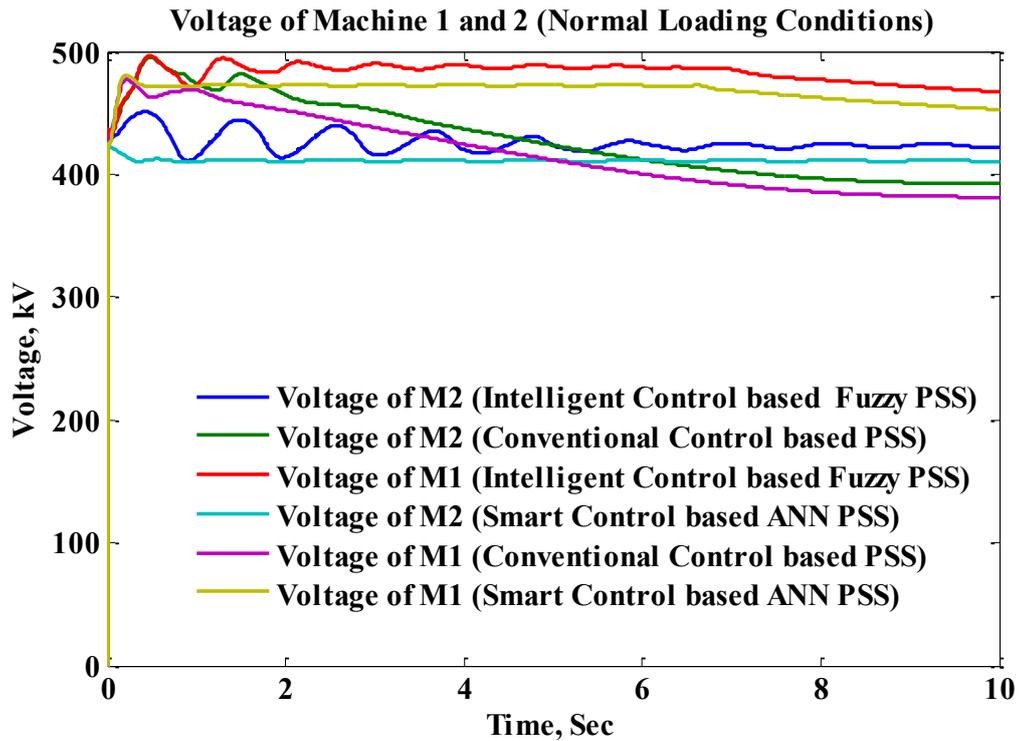
Fig. 4.24 Voltage comparisons for multimachine system (Normal Loading Condition)
