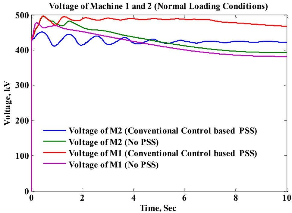
Fig. 4.8 Voltage performance of PSS installed in multimachine system for normal loading condition
