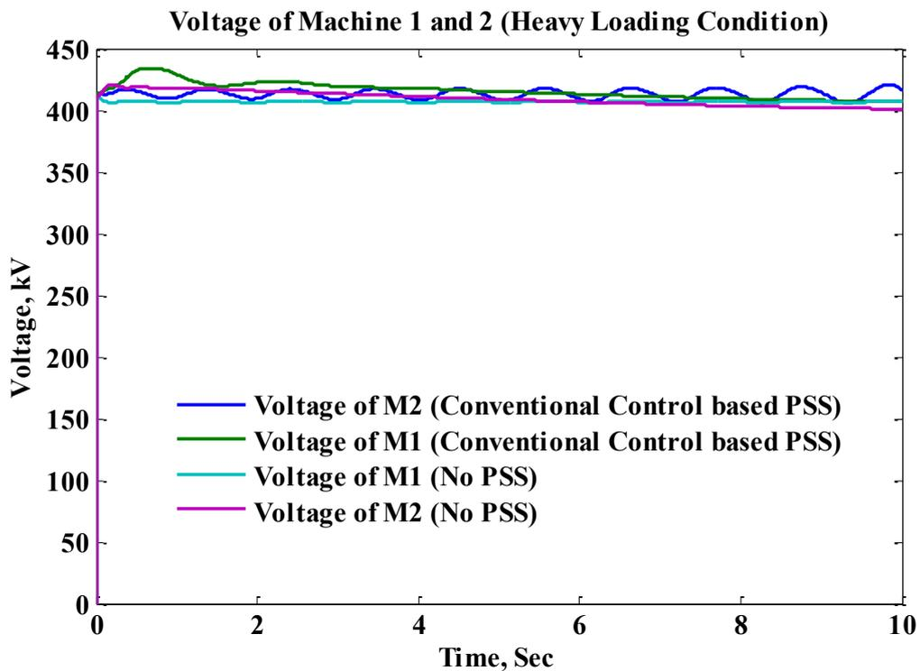
Fig. 4.9 Voltage performance of PSS installed in multimachine system for heavy loading condition
