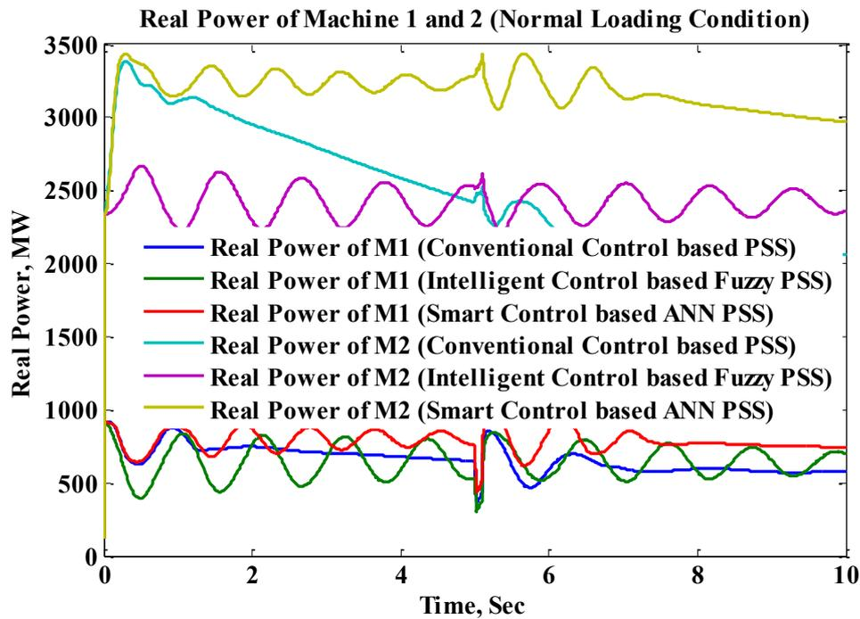
Fig. 4.27 Real power comparisons for multimachine system (Normal Loading Condition)
