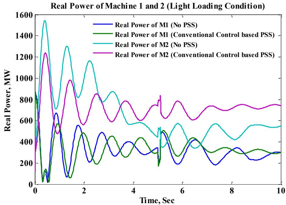
Fig. 4.10 Real power performance of PSS installed in multimachine system for light loading condition
