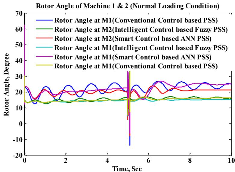
Fig. 4.21 Rotor angle comparisons for multimachine system (Normal Loading Condition)
