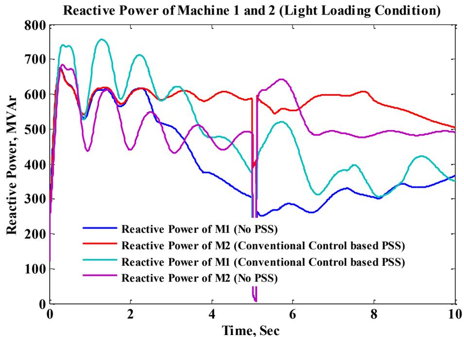
Fig. 4. 13 Reactive power performance of PSS installed in multimachine system for light loading condition
