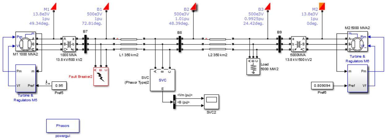
Fig. 4. 2 Simulink model Multimachine system with CPSS
