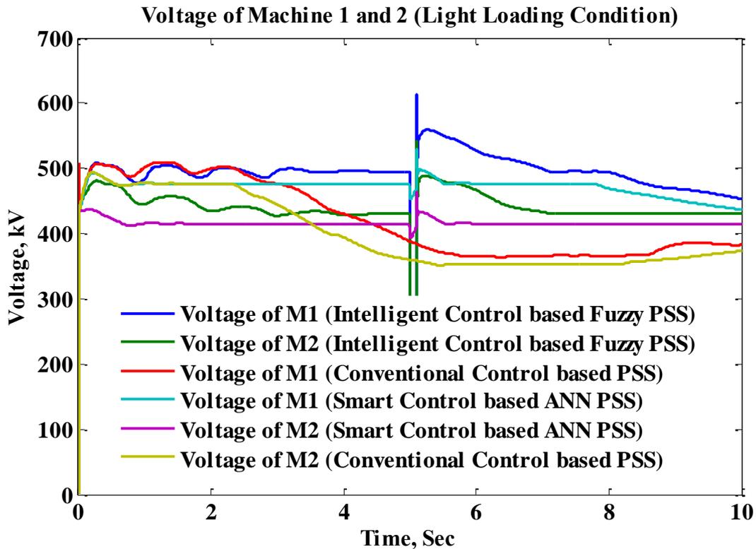
Fig. 4.23 Voltage comparisons for multimachine system (Light Loading Condition)
