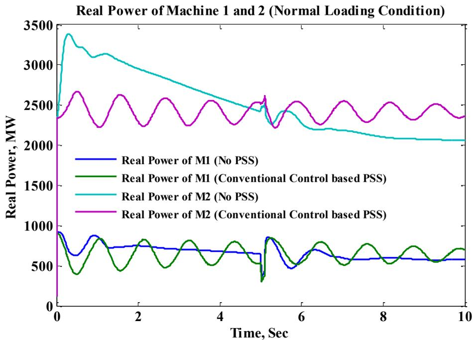
Fig. 4.11 Real power performance of PSS installed in multimachine system for normal loading condition
