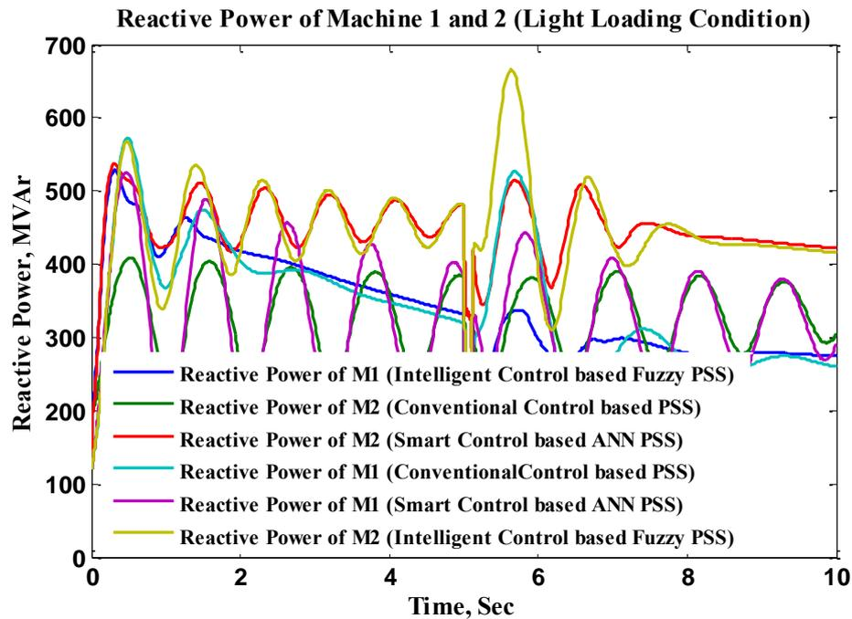
Fig. 4.29 Reactive power comparisons for multimachine system (Light Loading Condition)
