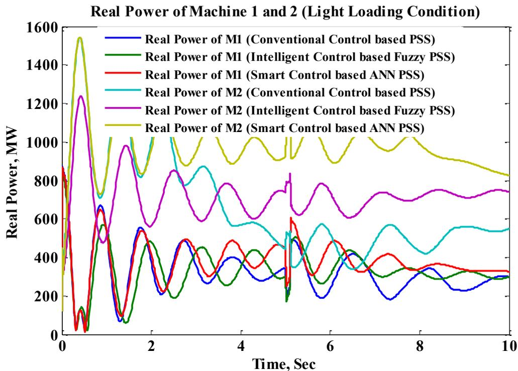
Fig. 4.26 Real power comparisons for multimachine system (Light Loading Condition)
