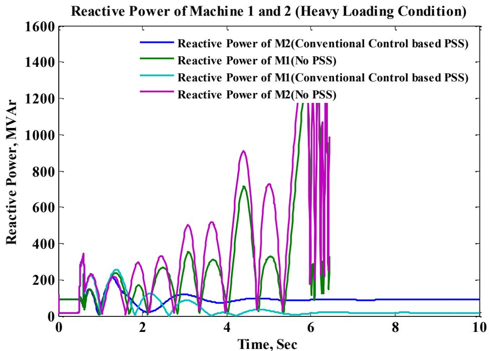
Fig. 4. 15 Reactive power performance of PSS installed in multimachine system for heavy loading condition
