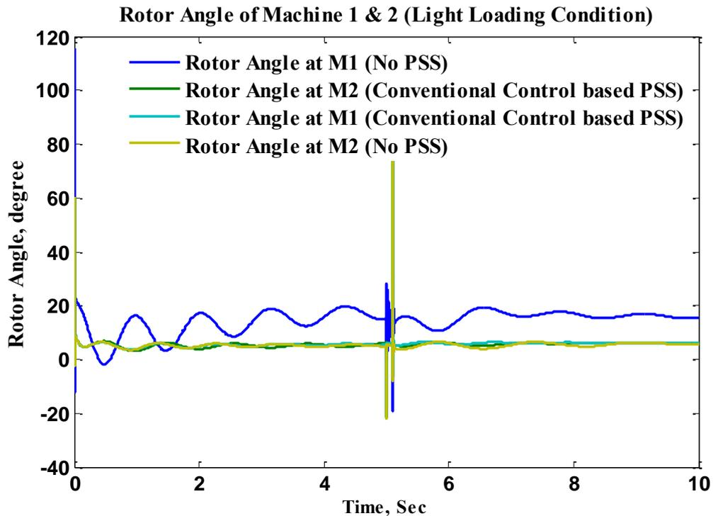
Fig. 4. 4 Rotor Angle Performance of PSS installed in multimachine system for light loading condition
