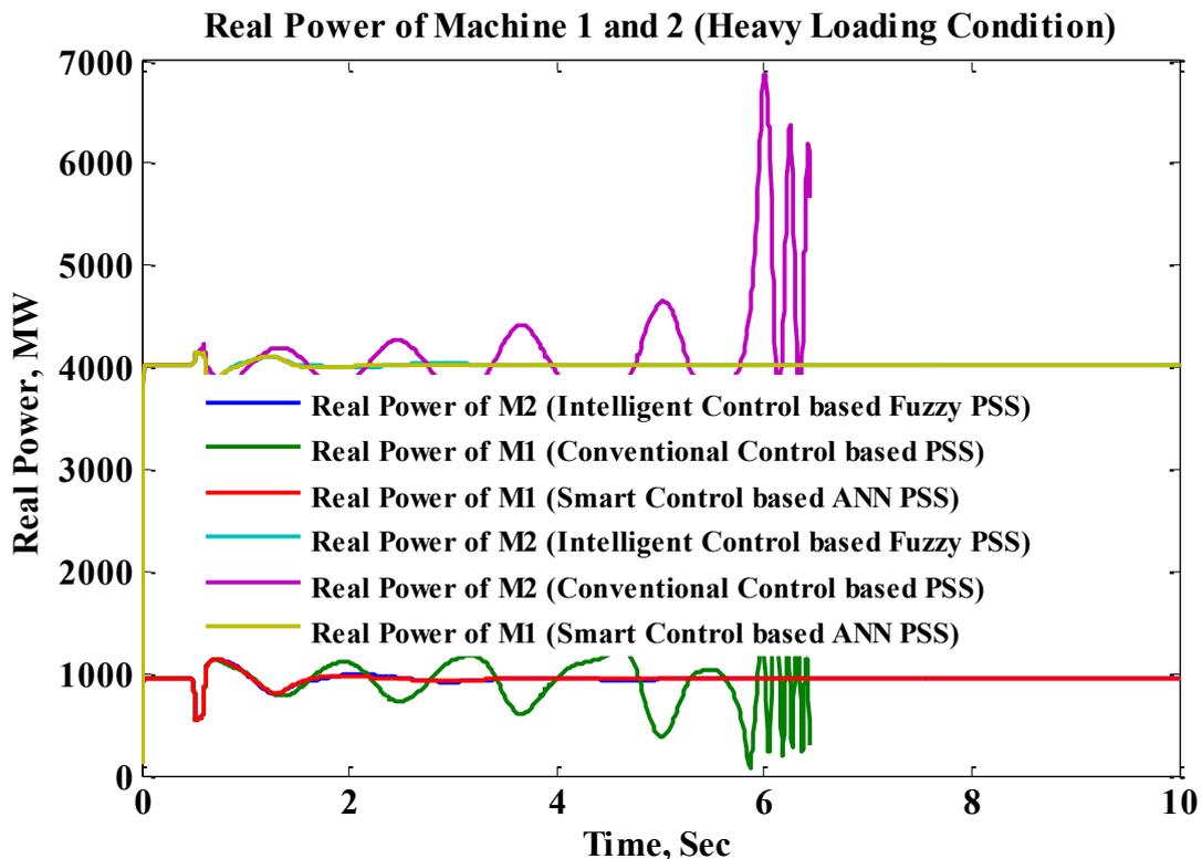
Fig. 4.28 Real power comparisons for multimachine system (Heavy Loading Condition)
