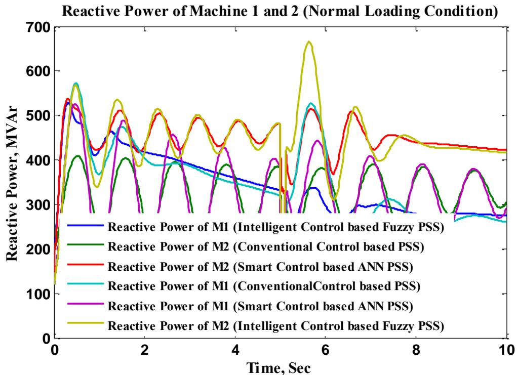
Fig. 4.30 Reactive power comparisons for multimachine system (Normal Loading Condition)
