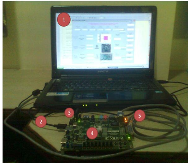
Figure B. 6: FPGA Setup: 1)CPU Core2Duo with Software tools installed, 2)USB cable, 3)Power cable, 4)Atlys board, 5)Gigabit Ethernet crossover cable
