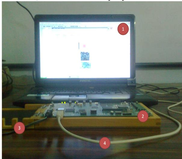
Figure B. 4: DSP Setup: 1)CPU Core2Duo with Software tools installed, 2)TMS320C6713 DSK, 3)Power Cable and 4)USB Cable
