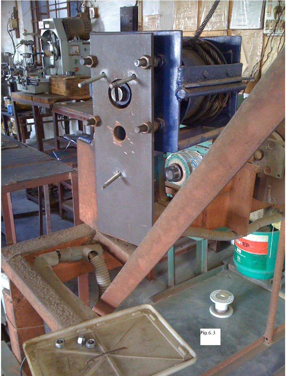
Figure 6.3 Experimental setup for loading the motor.
