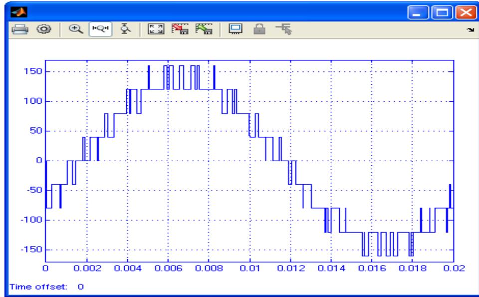
**Fig. 5.20 One phase output from three phase HMLI PD modulation technique**
