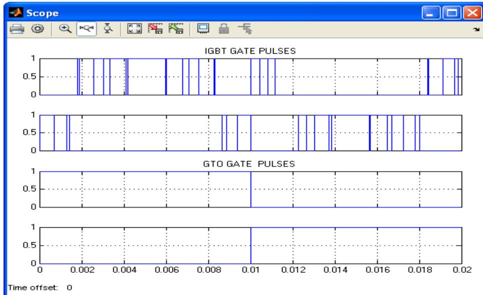
**Fig. 4.22 Control signals for asymmetric hybrid multilevel inverter**
