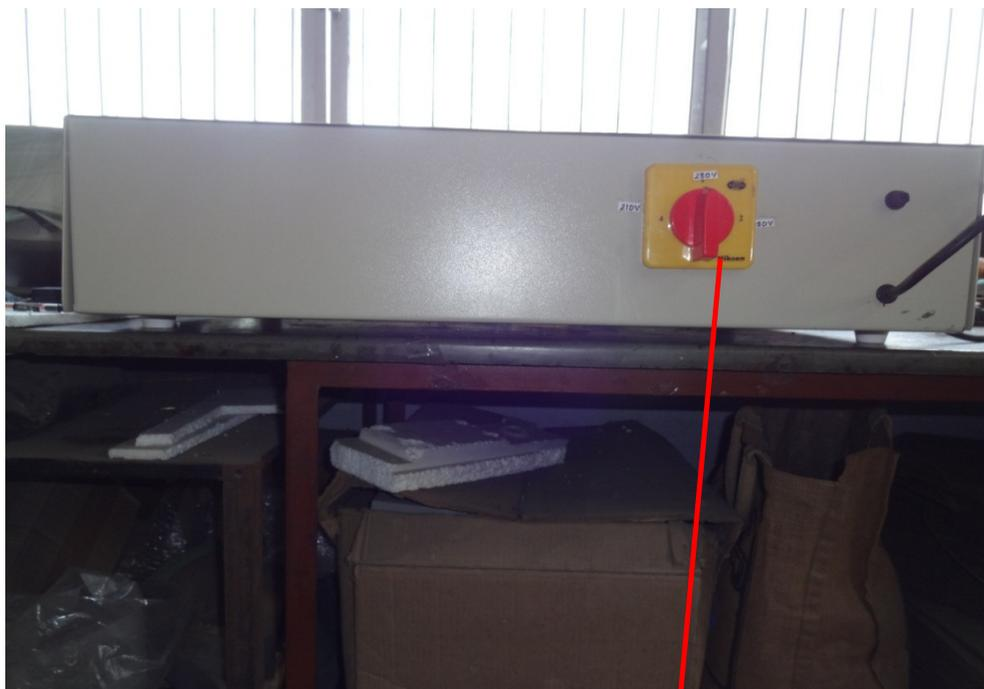
**Fig. B.8 Primary voltage selector**
