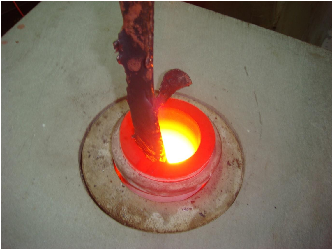
Figure B-18 Insertion of long copper piece to show effect of load inductance changes
