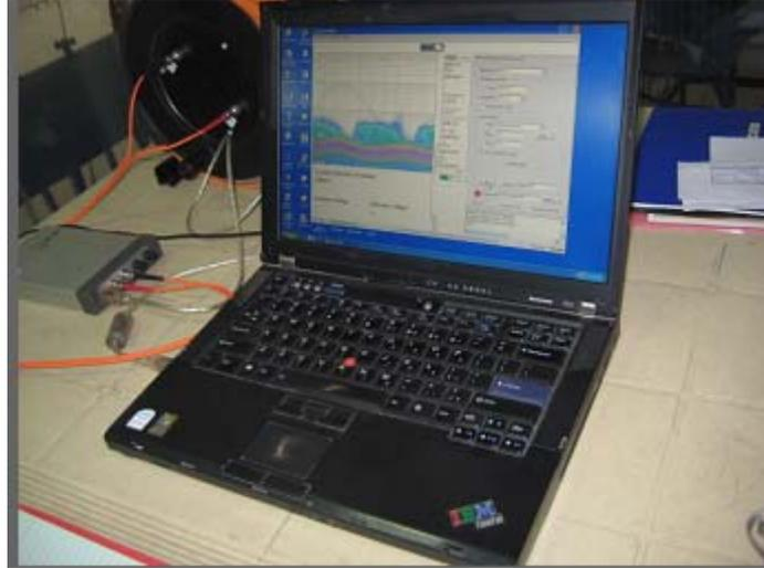
Figure-5.2 Data acquisition Setup for PD Measurement
