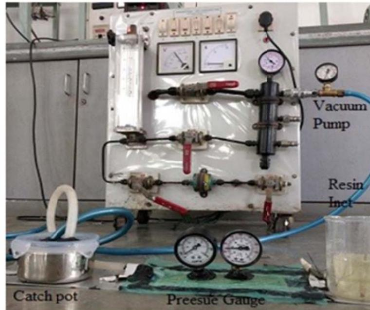
**Figure 2.5** Actual experimental setup for the vacuum infusion process.(Gajjar et al., 2020)
