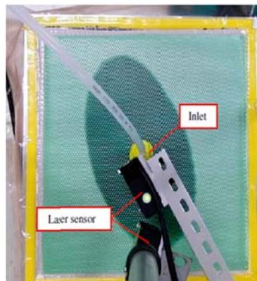
**Figure 2.3** Top view of resin infusion behaviour. (Yokozeki et al., 2014)
