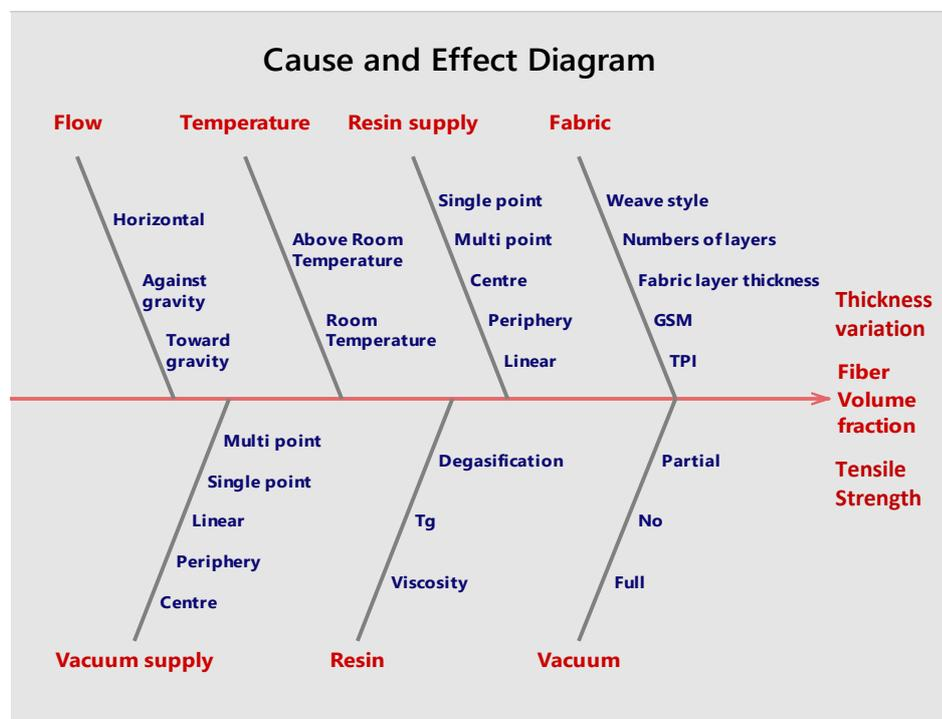
**Figure 2.6** Cause and Effect diagram for parameters affecting VARTM process
