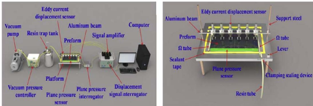
**Figure 2.4** Schematic diagram of an integrated experimental setup for testing in-plane permeability adopted in the study. (Changchun et al., 2015)
