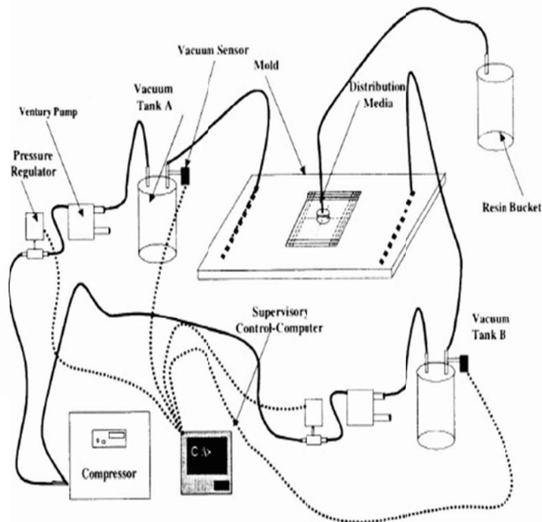
**Figure 2.1.** Schematic of VARTM Control system incorporating computer control pressure and vacuum in-situ vacuum sensing for two individual vents. (Heider et.al., 1999)
