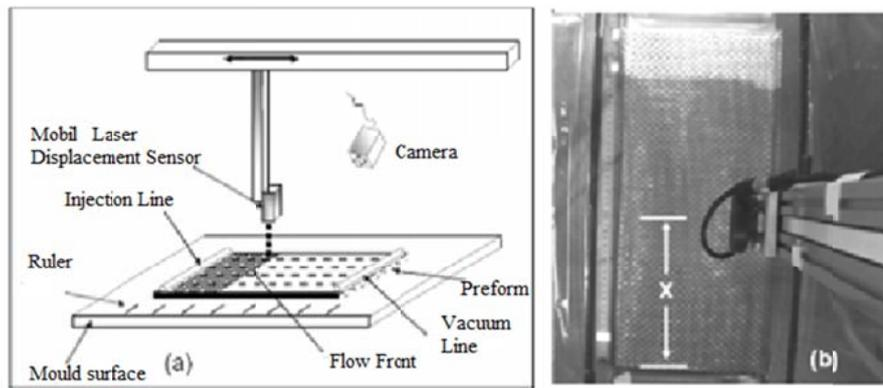
**Figure 2.2** a) The Schematic of the laser scanner to increase during infusion b) the laser scanner above the mold. (Lawrence et al., 2007)
