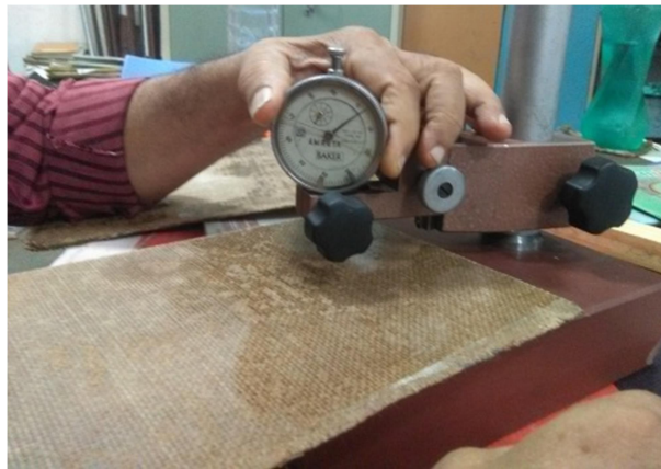
Figure 5.6 Measuring laminate thickness with mechanical comparator
