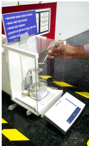
Figure 5.10 Composite density measurements
