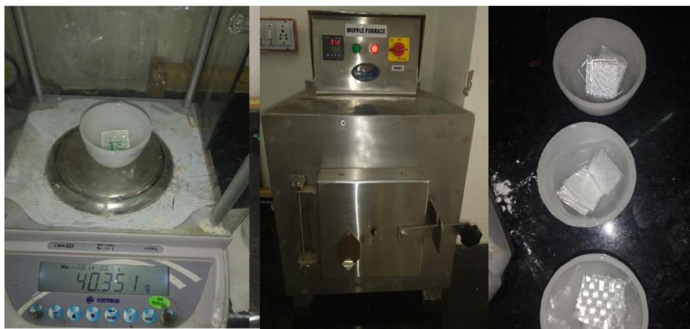
Figure 5.8 Weight fractions measurement by LOI method for glass fabric. a) Weighing of glass laminate b) putting in muffle furnace c) weighing fabric after keeping in furnace for 2 hours at 565 \pm 28^\circ \text{C}
