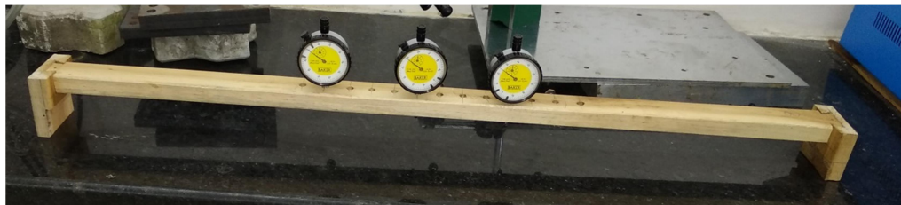
Figure 5.1 Fixture to measure thickness variations during the flow
