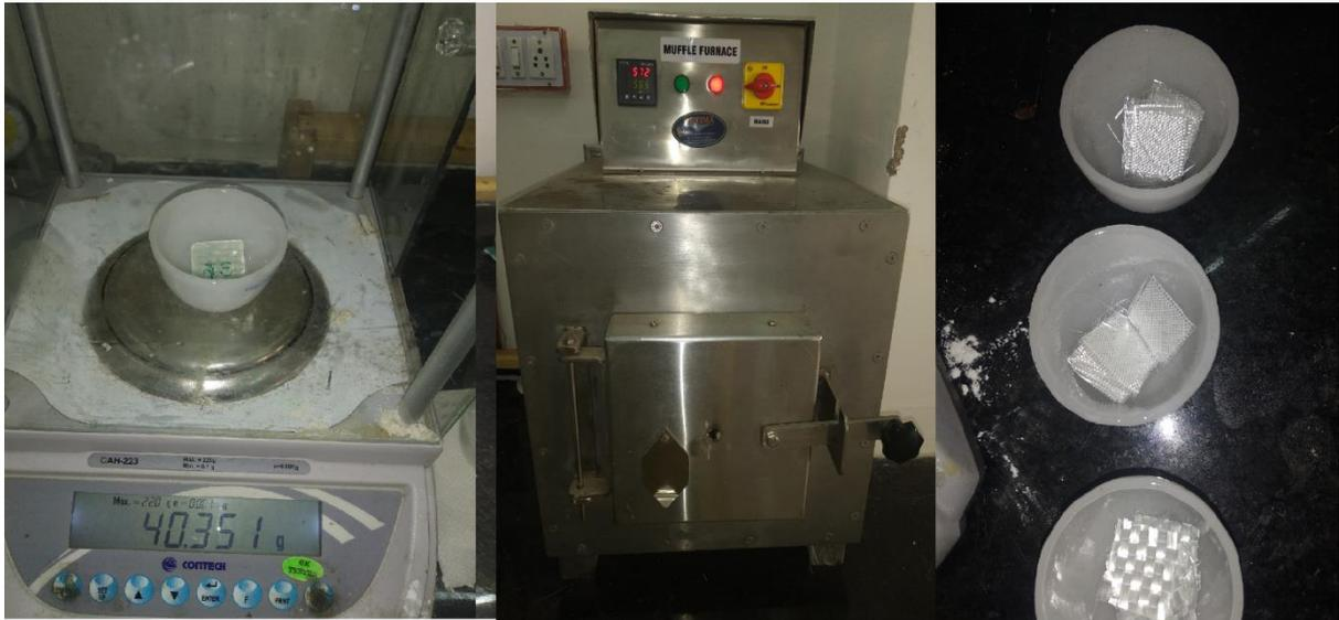
Figure 18 Weight fraction by LOI method for glass fabric. a) Weighing of glass laminate b) putting in muffle furnace 3) weighing fabric after keep in furnace for 2 hours at  $565 \pm 28^\circ \text{C}$
