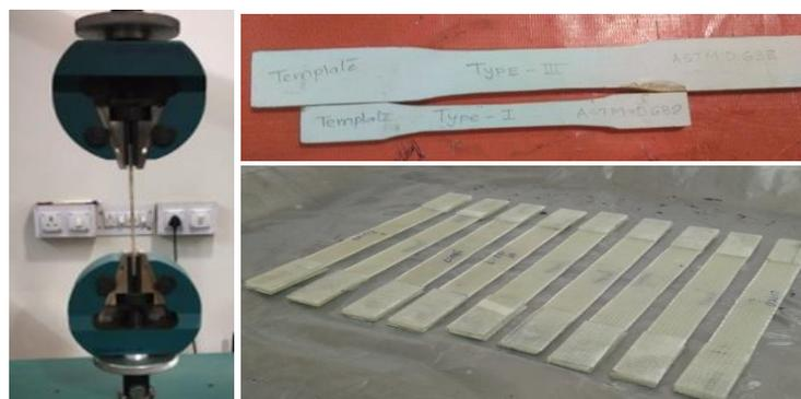
Figure 14 Tensile testing specimen & fixture details
