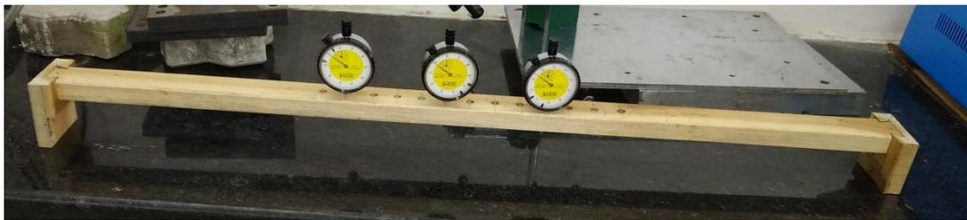
Figure 11 Fixture to measuring thickness variations during the flow
