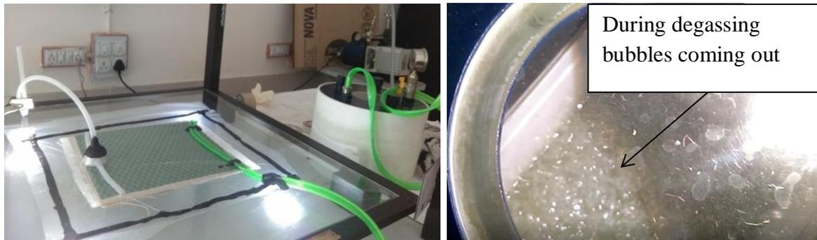
Figure 8 Experimental setup with degassing
