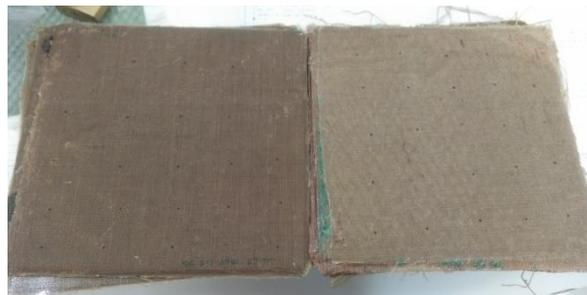
Figure 28 Color of laminate with and without degassing
