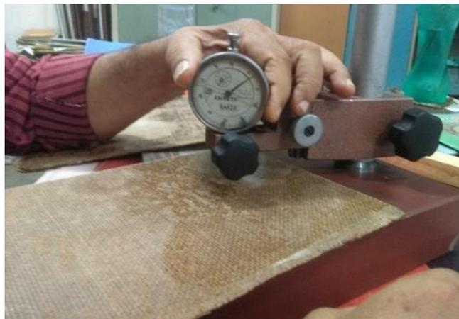
Figure 16 Measuring laminate with mechanical comparator
