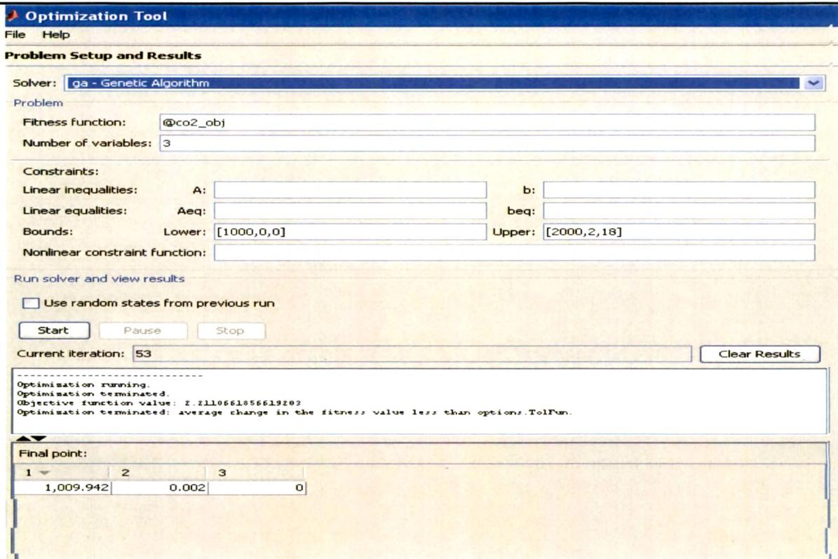
Fig. 4.21 MATLAB Screen to Show Single Objective Optimization of CO<sub>2</sub>
