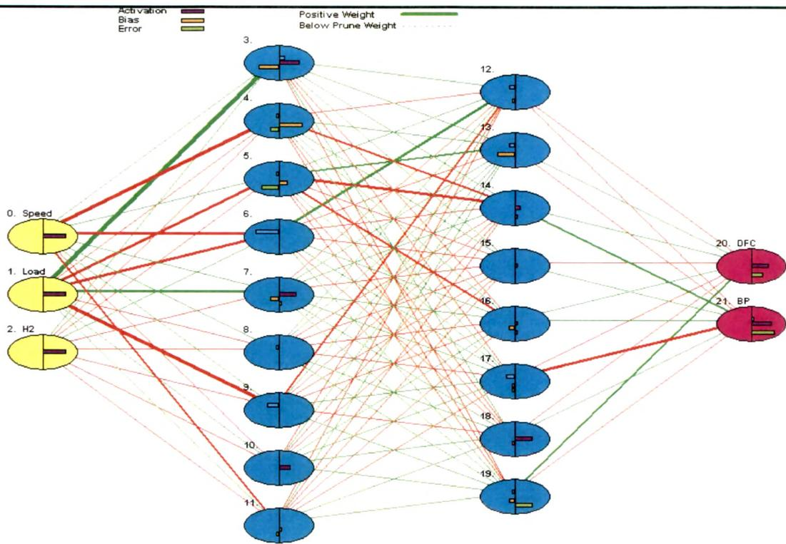
Fig. 4.6 ANN Model of Engine Performance with Architecture 3,10,9,2
