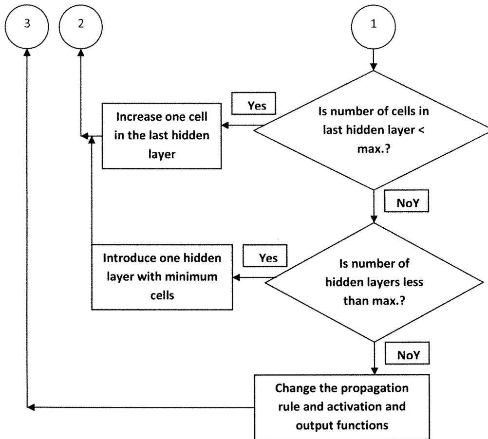
Fig. 4.3 Flow Chart for Neural Network Modeling Approach
