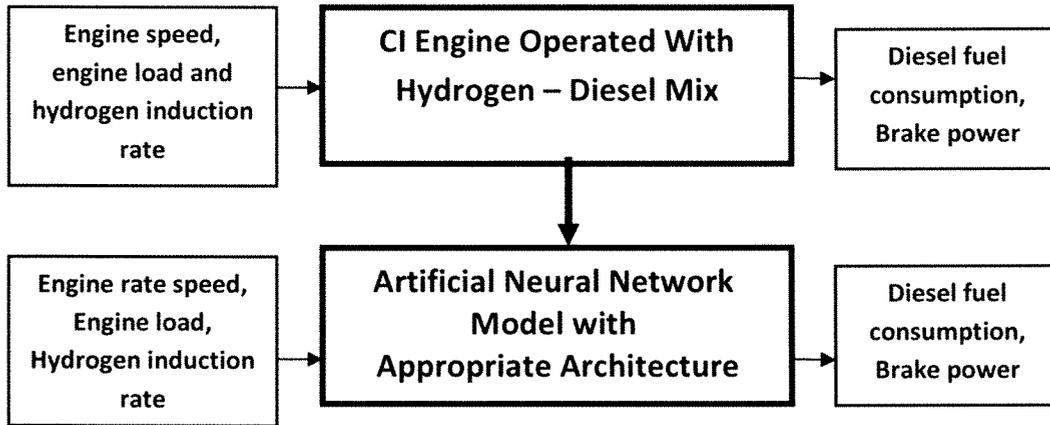
**Fig. 4.4 Layout of Artificial Neural Network Model for Engine Performance**
