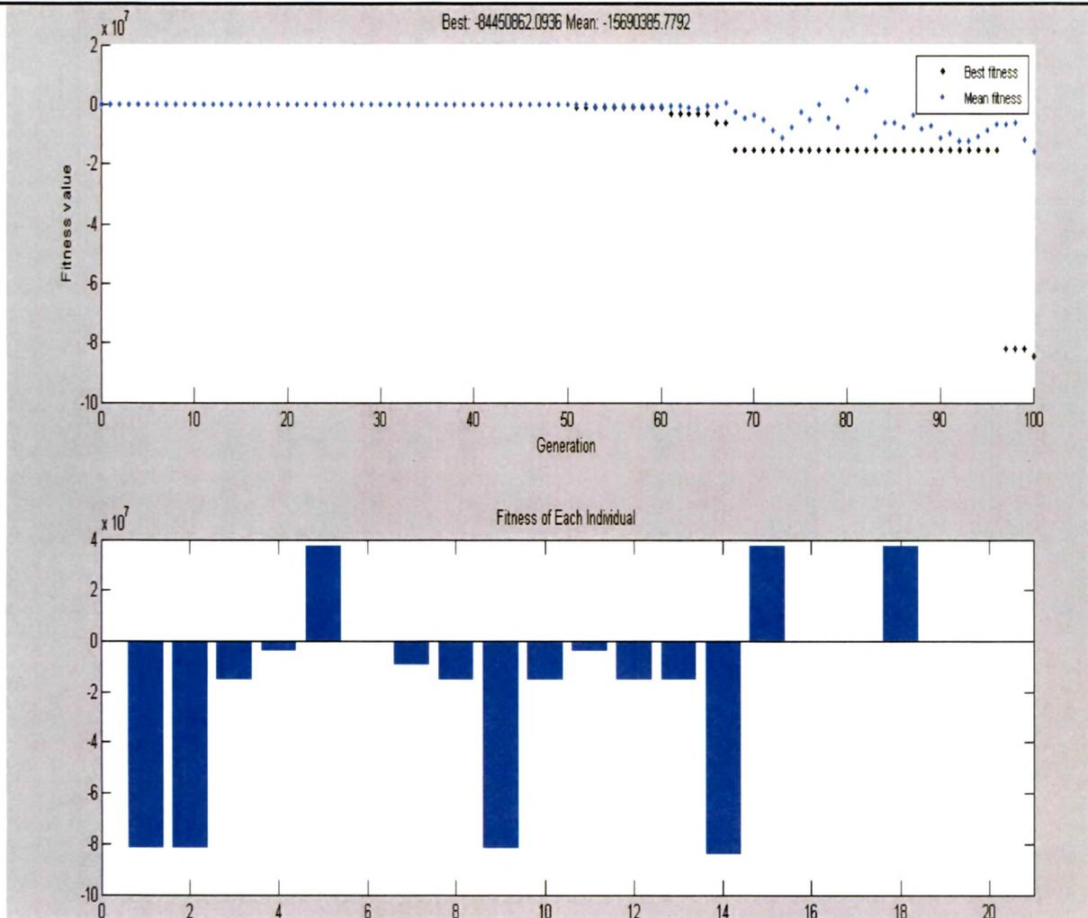
*Fig. 4-14 Variation of Fitness Value with Generation Growth for Single Objective Optimization of Brake Power*
