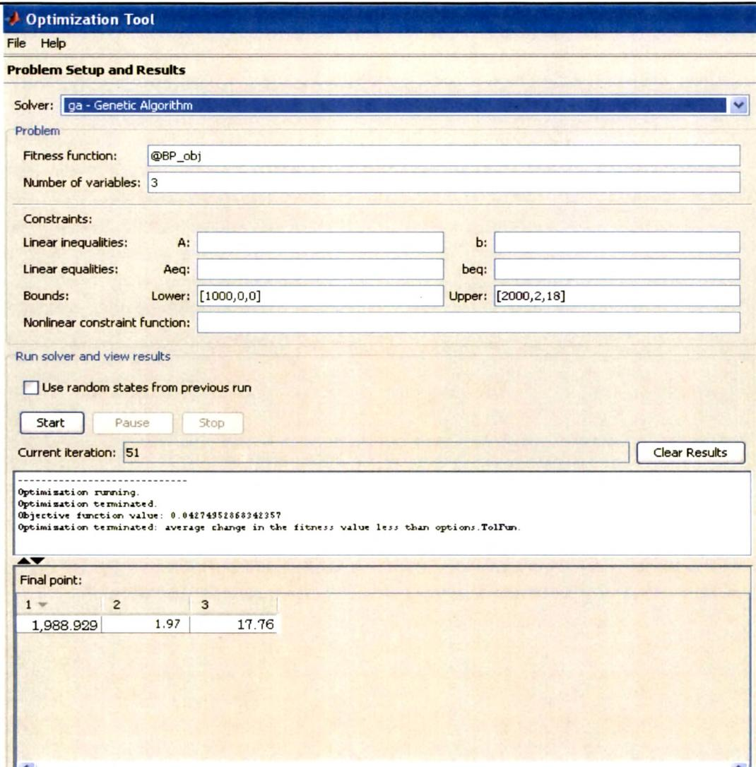
Fig. 4.15 MATLAB Screen to Show Single Objective Optimization of Brake Power
