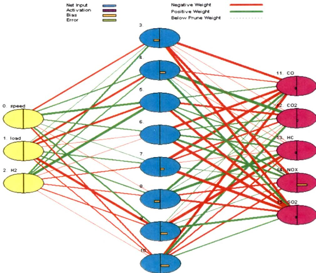
*Fig. 4-10 ANN Model of Engine Gas Emission Constituents with Architecture 3,10,5*
