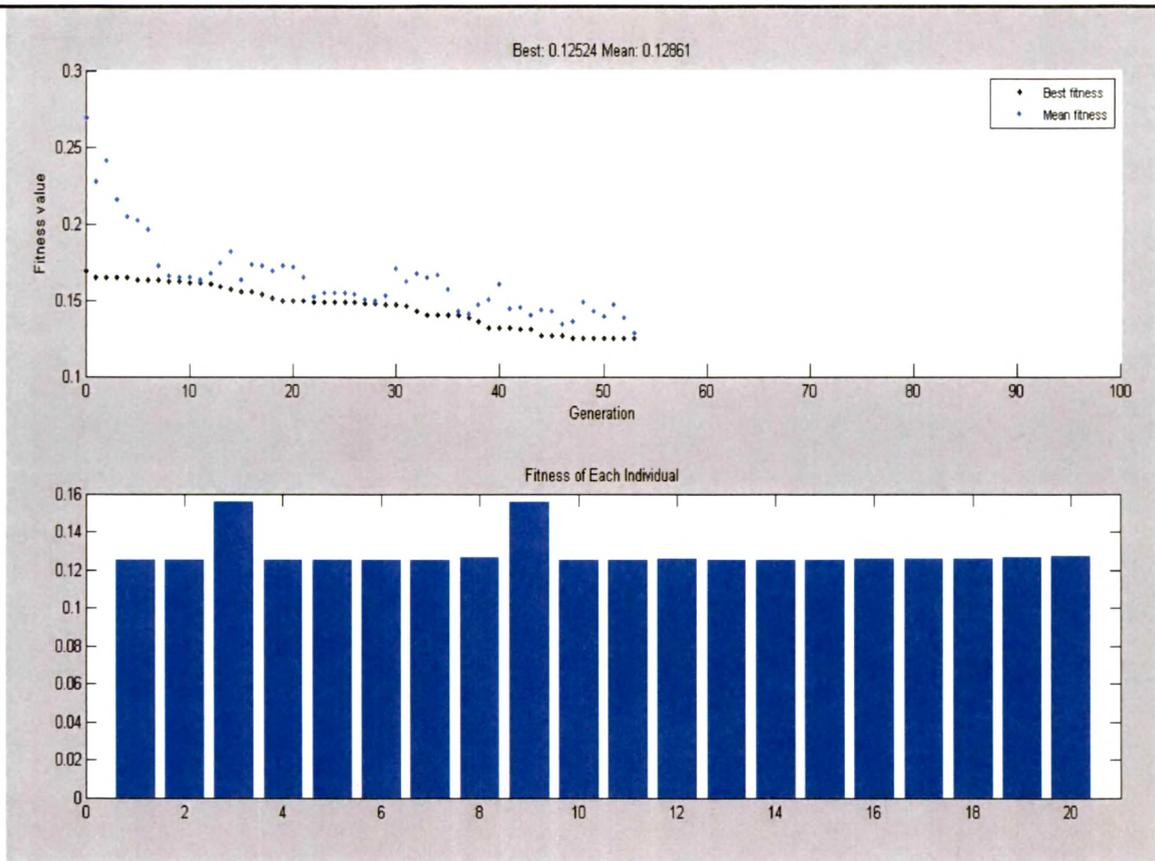
**Fig. 4.16** Variation of Fitness Value with Generation Growth for Single Objective Optimization of Diesel Fuel Consumption
