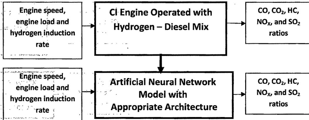
**Fig. 4.8 Schematic of Artificial Neural Network Model for CI Engine Gas Emission Constituents**
