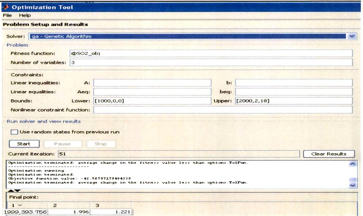
Fig. 4.25 MATLAB Screen to Show Single Objective Optimization of SO<sub>2</sub>
