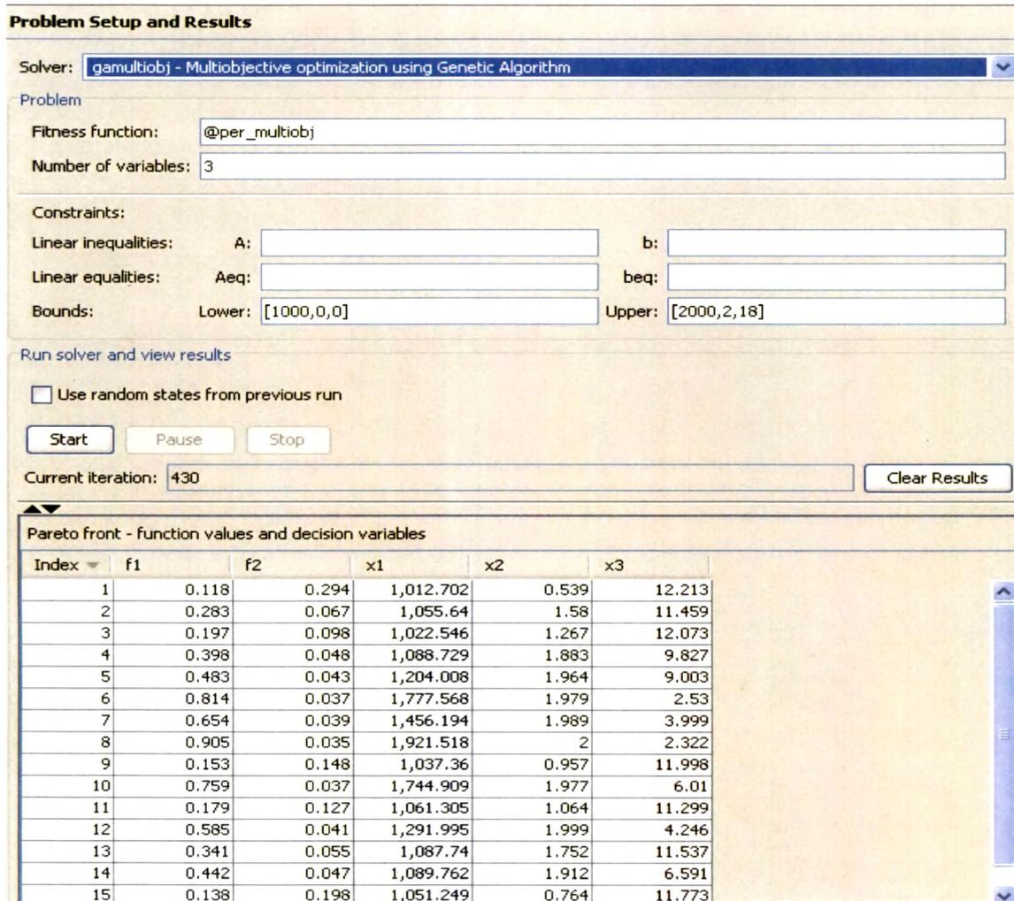
**Fig. 4.30 Display Screen of MATLAB Program for Multi Objective Optimization of Maximum Brake Power and Minimum Diesel Fuel Consumption**
