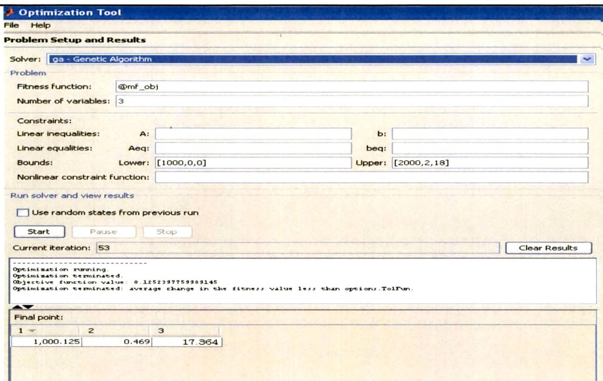
Fig. 4.17 MATLAB Screen to Show Single Objective Optimization of Diesel Fuel Consumption
