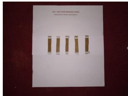
Figure 4.12 Specimens of In-Process Curing Jute-Vinyl Ester Composite as per ASTM D790 for Flexural Test
