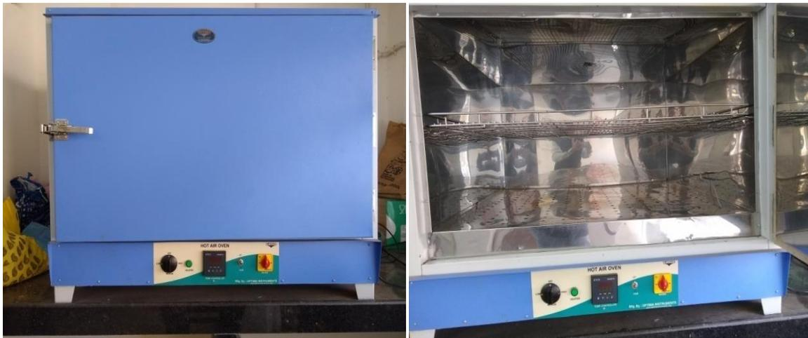
Figure 4.1 Developed Hot Air Oven for Post-Process Curing
