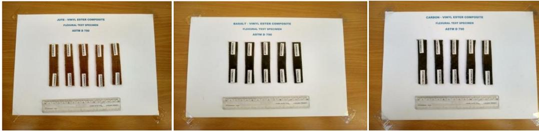
Figure 4.11 Post Cured Specimens of Jute, Basalt and Carbon Fibers with Vinyl Ester as per ASTM D790 for Flexural Test
