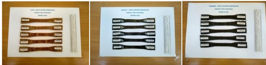
Figure 4.8 Post Cured Specimens of Jute, Basalt and Carbon Fibers with Vinyl Ester as per ASTM D638 for Tensile Tests
