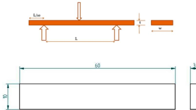
Figure 4.5 Specimen Dimensions as per ASTM D790 for Flexural Test
