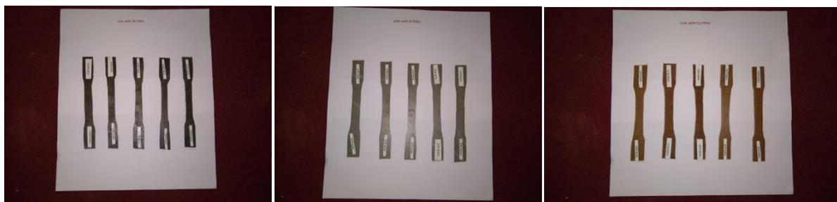
Figure 4.10 (a) Specimens with SiC Filler (b) Specimens with AL Filler (c) Specimens with Cu Filler
