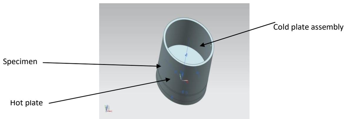
Figure 4.18: Assembly of a Hot Plate and Cold Plate
