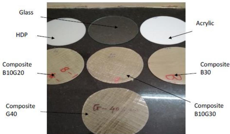
Figure 4.21 Specimens Prepared for Thermal Conductivity Measurement (as per ASTM C1530) of Different Combination of Bamboo and Glass Fibers
