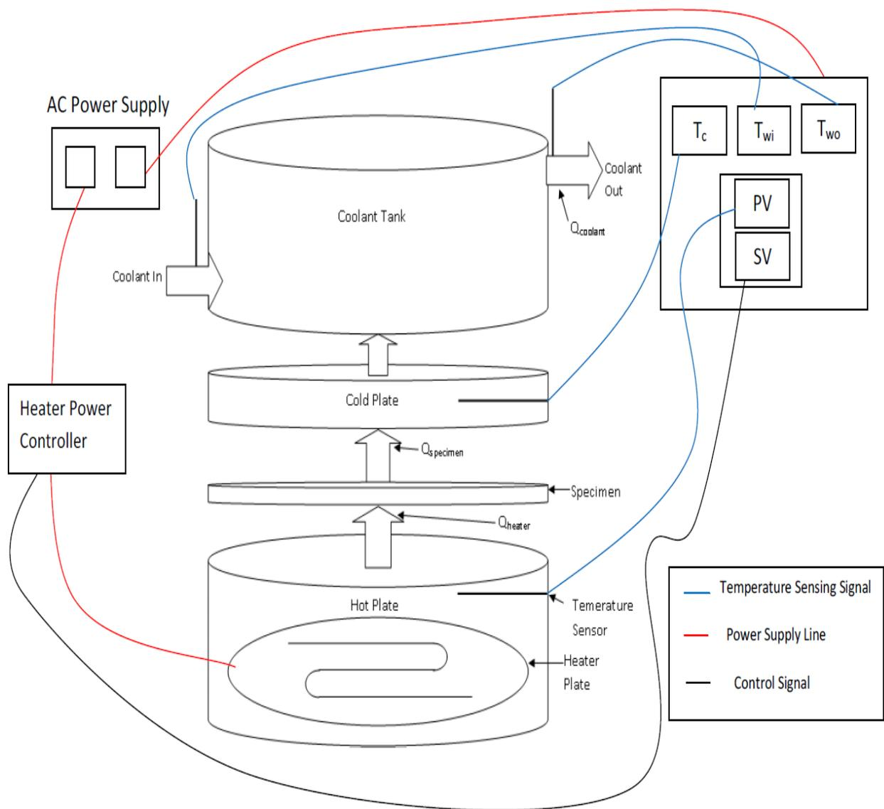
Figure 4.19: Schematic Diagram of the Developed Experimental Setup for Measuring Thermal Conductivity
