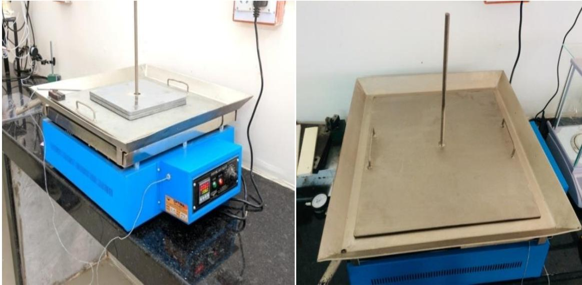
Figure 4.2 Developed Punch and Mould Assembly with Hot Plate for In-Process Curing
