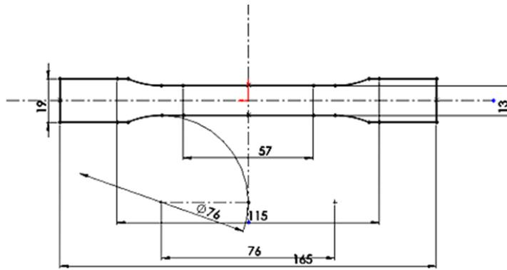
Figure 4.3 Specimen Dimension as per ASTM D638 for Tensile Test
