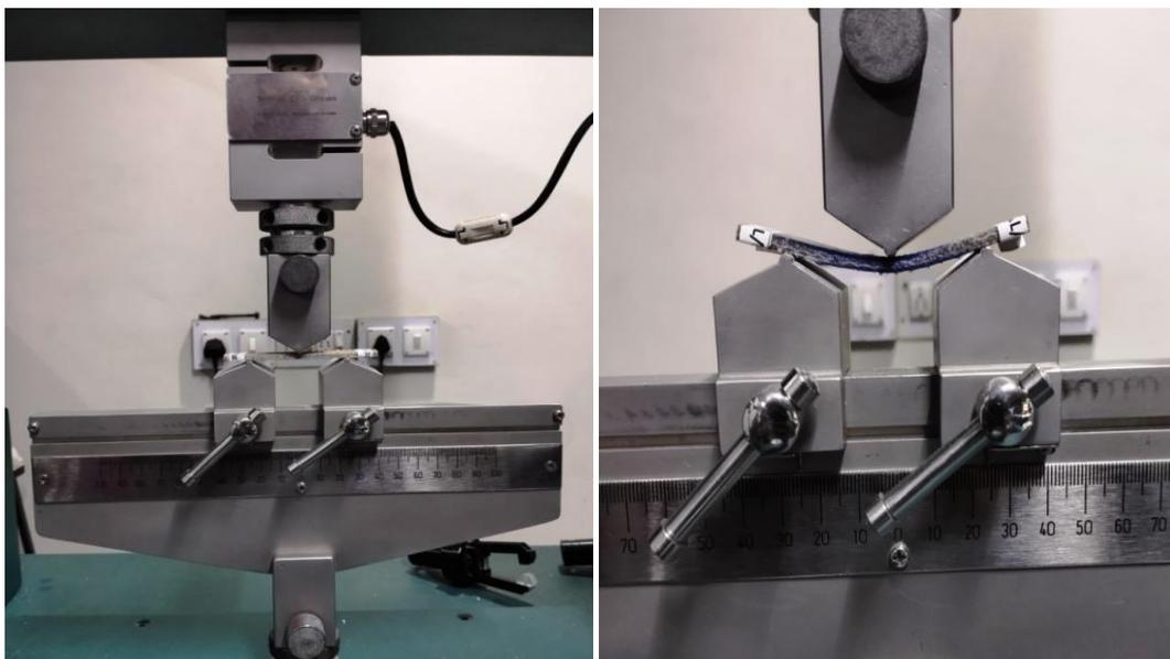
Figure 4.6 Flexural Testing in Universal Testing Machine
