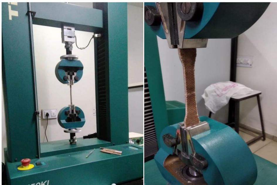
Figure 4.4 Tensile Testing in The Universal Testing Machine (UTM) (Model: TINIUS OLSEN/LSeries H50KL)
