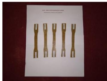
Figure 4.9 Specimens of In-Process Curing of Jute Vinyl ester Composite for a Tensile Test as per ASTM D638 Standards
