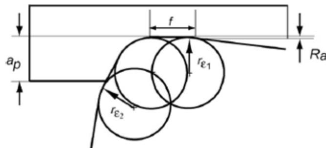
Fig. 2.15 Wiper insert design:  $r_{e1}$  and  $r_{e2}$  are the radii of wiper curvature [45]
