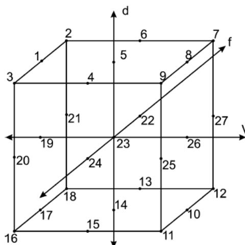
Fig. 2.25 Central composite design for three factors [61]
