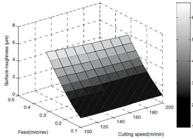
Fig. 2.16 (a) Effective rake angle =  $6^{\circ}$ , nose radius = 0.4 mm [47]
