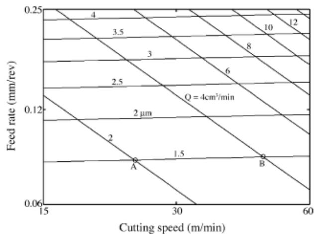
Fig.2.11 Response contours of surface roughness and metal removal Q [36]
