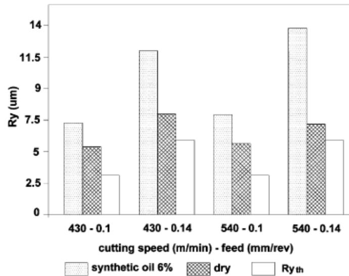
Fig. 2.1 Surface roughness ( $R_y$ ) for all the conditions tested ( $r_e = 0.4\text{mm}$ ) [24]
