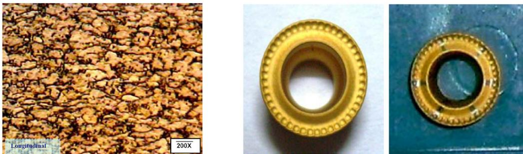
Fig. 2.29 Microstructure of Ti-6Al-4V [69] Fig. 2.30 CVD coated carbide insert [69]
