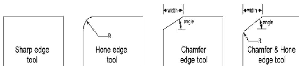
Fig. 2.17 Type of edge preparations used in CBN and ceramic cutting tools [49]
