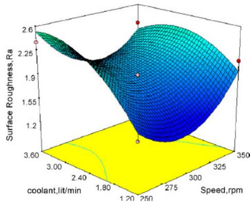
Fig. 2.19 3D surface graph for the surface roughness at feed = 50mm/min as speed and coolant varies [50]
