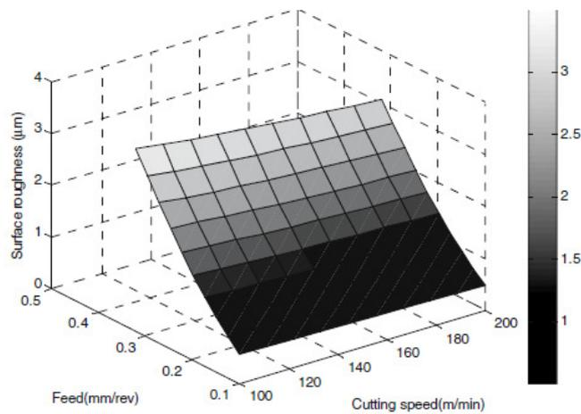
Fig. 2.16 (c) Effective rake angle =  $6^{\circ}$ , nose radius = 1.2 mm [47]
