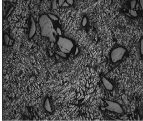
Fig. 2.21 Microstructure of the Al-SiC (20 p) MMC [54]
