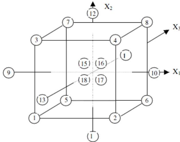
Fig. 2.10 Central composite design for three factors [35]
