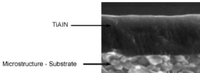
Fig. 2.23 Coating layer of Insert 2 [55]
