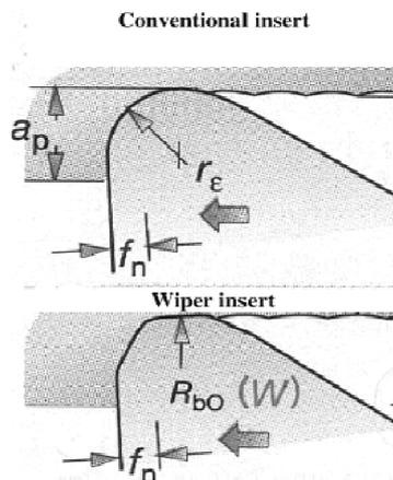
Fig. 2.27 Comparison of inserts with conventional and wiper (multi-radii) geometry [67]
