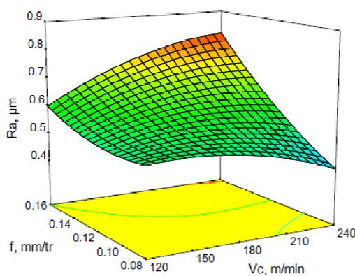
Fig. 2.31 Effect of cutting speed and feed [70]
