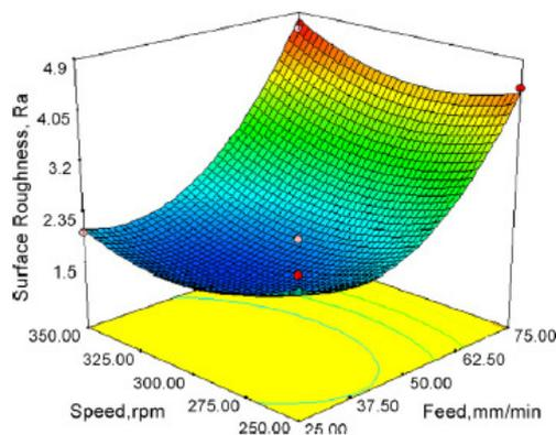
Fig. 2.18 3D surface graph for the surface roughness at Coolant = 2.4 l/min, as speed and feed varies [50]
