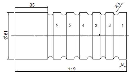
Fig. 2.28 Pre prepared work pieces in AISI 1045 used in turning tests [67]
