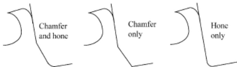
Fig. 2.9 Cutting with various edge geometry CBN tools [34]
