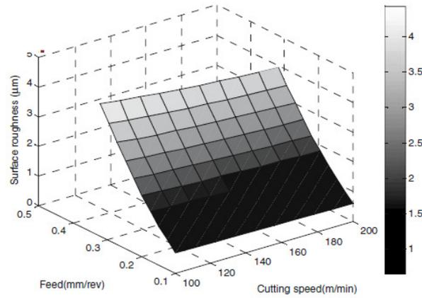
Fig. 2.16 (b) Effective rake angle =  $6^{\circ}$ , nose radius = 0.8 mm [47]
