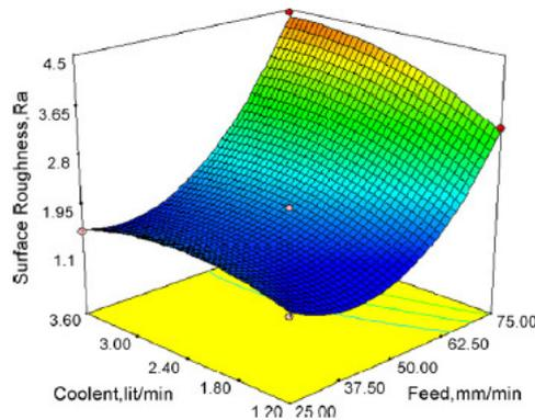
Fig. 2.20 3D surface graph for the surface roughness at speed = 300 rpm as coolant and feed varies [50]
