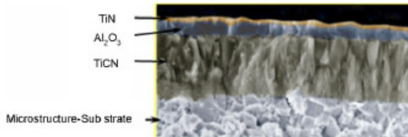
Fig. 2.22 Coating layers of Insert 1 [55]
