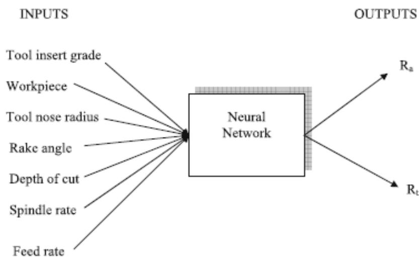
Fig. 2.12 Inputs and outputs of the network [39]
