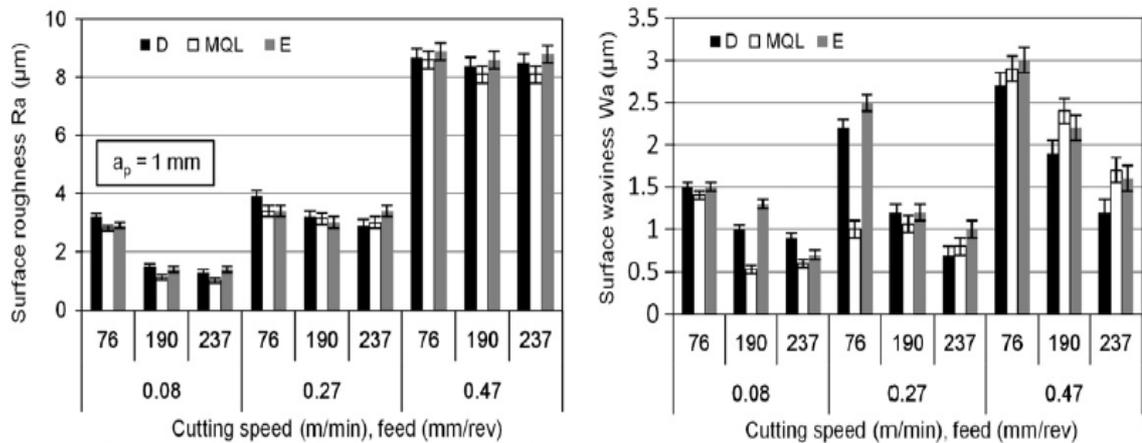
Fig. 5.6 Surface roughness and waviness depending on cooling and lubrication conditions and cutting parameters [66]
