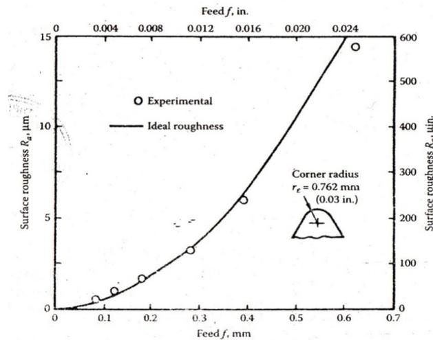
Fig. 5.4 Comp. of experimental results with an idealized model of surface roughness
