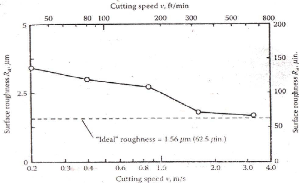
Fig. 5.5 Effect of cutting speed on the surface roughness for turning M.S.
