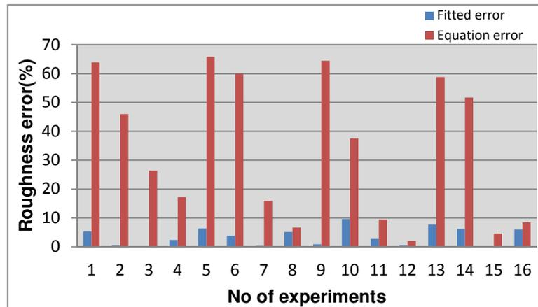
Fig. 5.13 Relative error of the fitted values vs. Computed values (AISI 410 steel and Aluminium)
