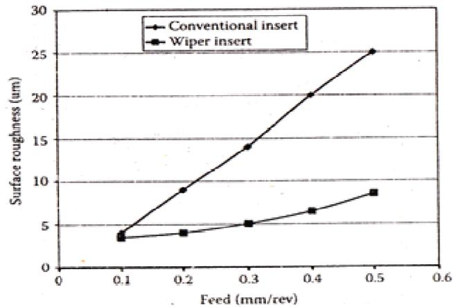
Fig. 5.9 Effect of feed on the effectiveness of a wiper inserts [38]
