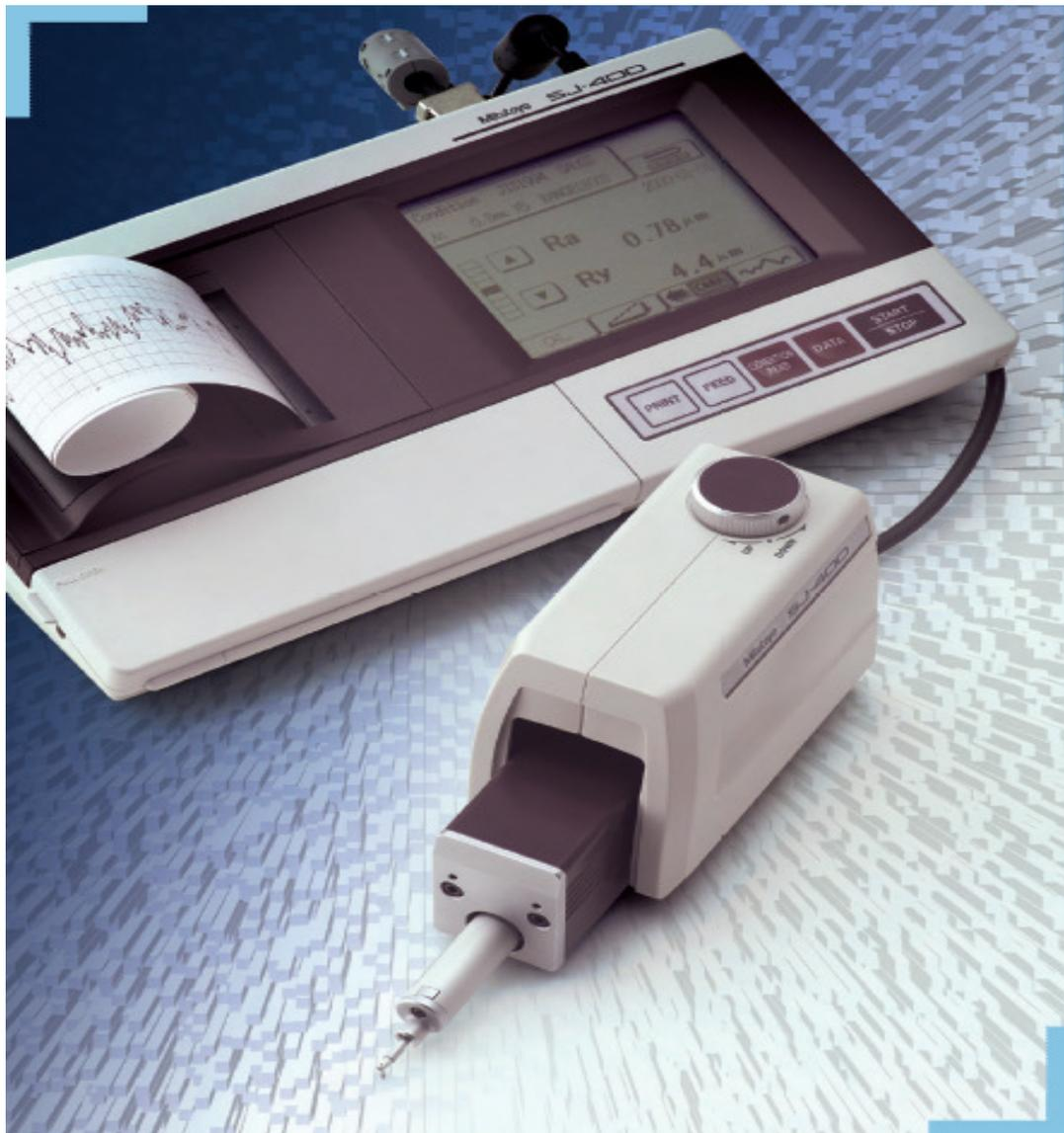
Fig. 5.7 Surface roughness tester SJ-400
