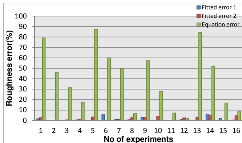
Fig. 5.14 Comparison of the fitted values and the estimated values (AISI 1040 steel and Aluminium)
