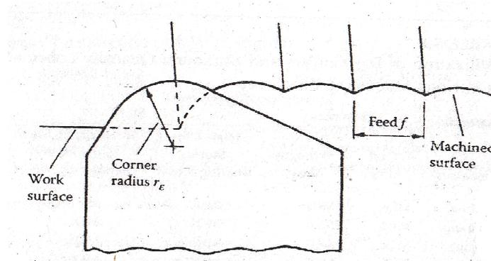
Fig. 5.3 Idealized model of surface roughness for round corner tool [38]
