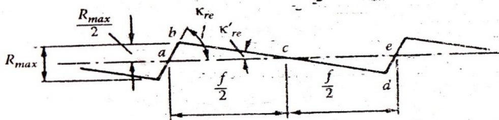
Fig. 5.1(b) Cross section through surface irregularities [38]
