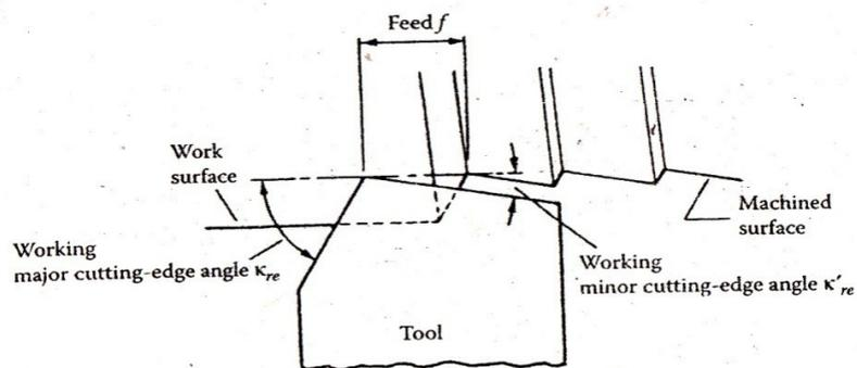
Fig. 5.1(a) Idealized model of surface roughness with sharp corner cutting tool [38]
