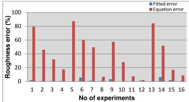
Fig. 5.12 Relative error of the fitted values vs. Computed values (AISI 1040 steel and Aluminium)
