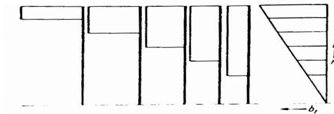
Figure: 3.3 possible shapes of impellers at 20% inlet acceleration
