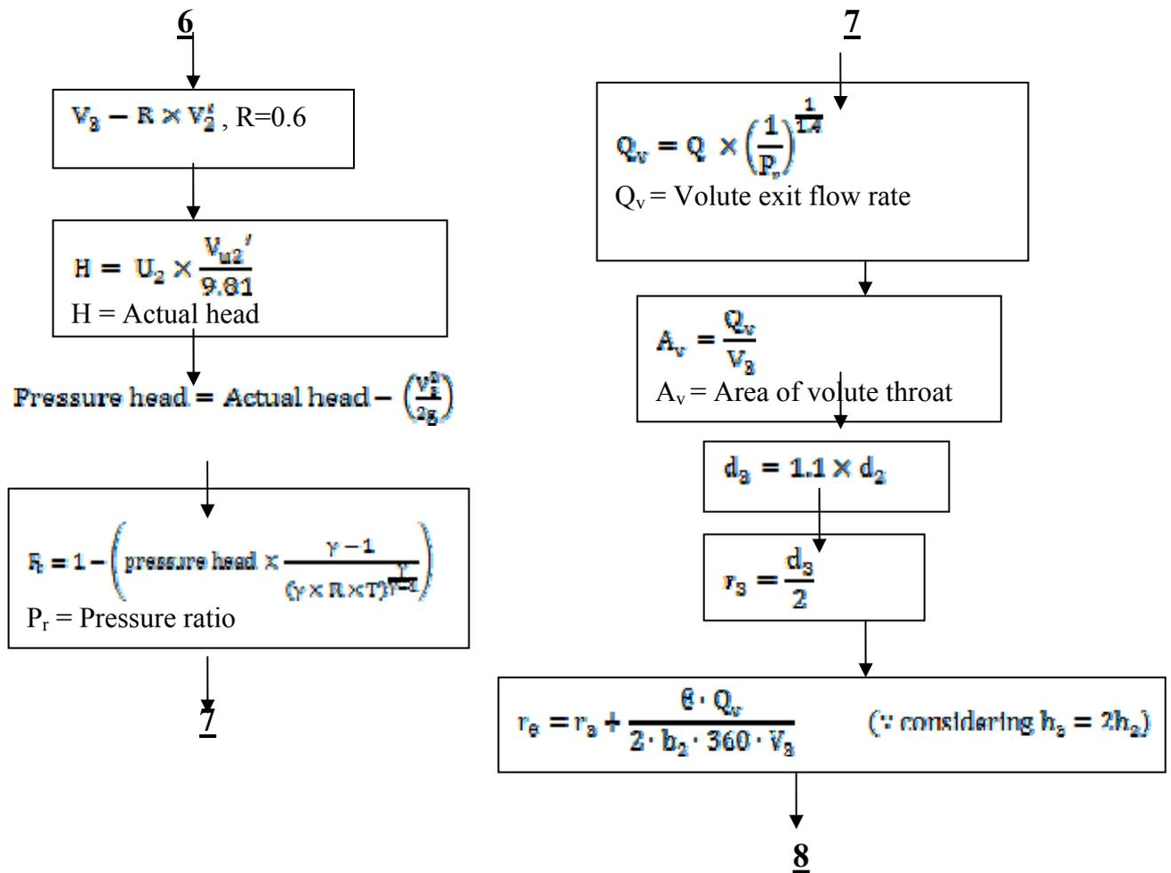
Volute widths  $b_3$  are typically taken equal to  $2b_2$  or  $1.25b_2$ . The volute widths do not affect performance appreciably. Rather, smaller volute width yields bigger volutes. [9] Thus, in present work, volute width  $b_3 = 2b_2$  is preferred in order to achieve a smaller design.
