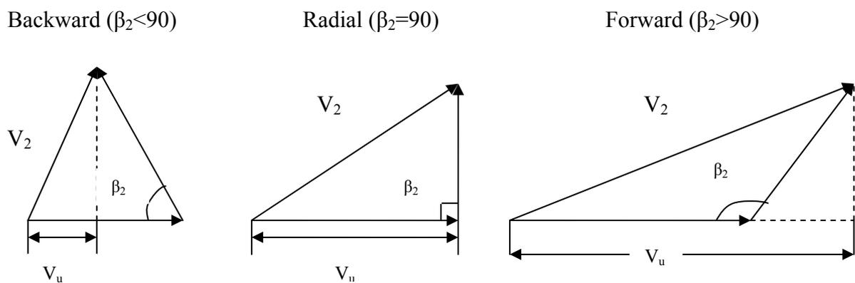
Figure: 3.6 Outlet velocity triangles
