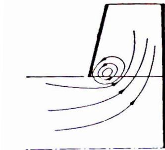
Figure: 3.2 Back flow at inlet of impeller due to large inlet breadth  $b_1$
