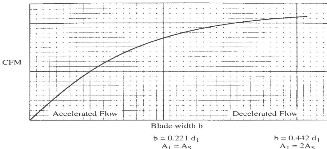
Figure: 3.4 Significance of impeller eye area and blade inlet area
