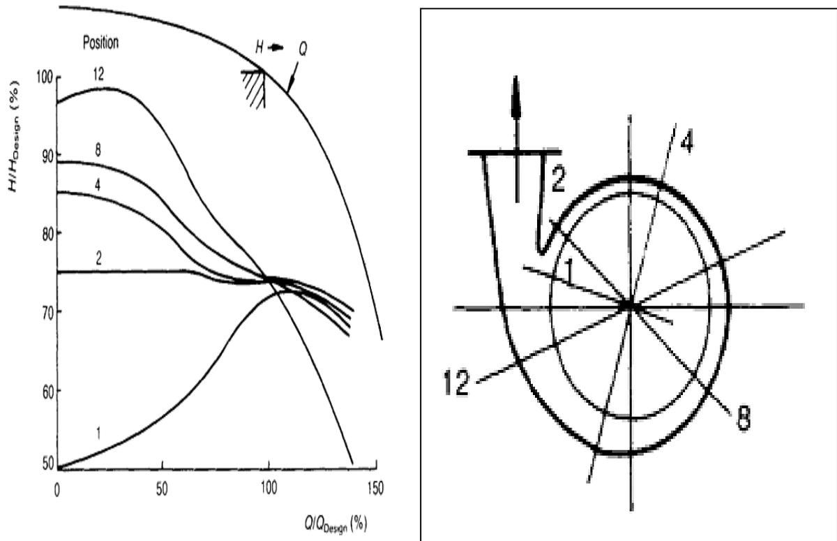
Figure: 3.8 Variation of pressure round an impeller.
