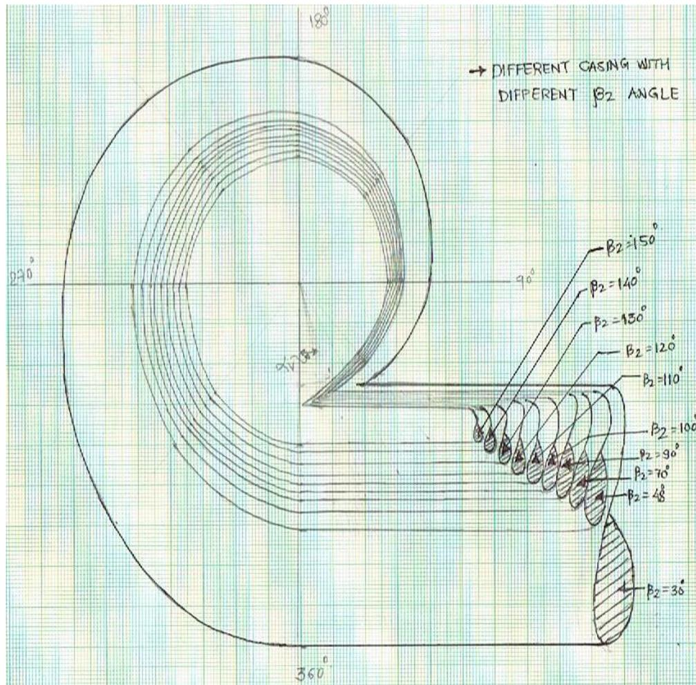
Figure: 3.7 Size of Volute with different outlet angle
