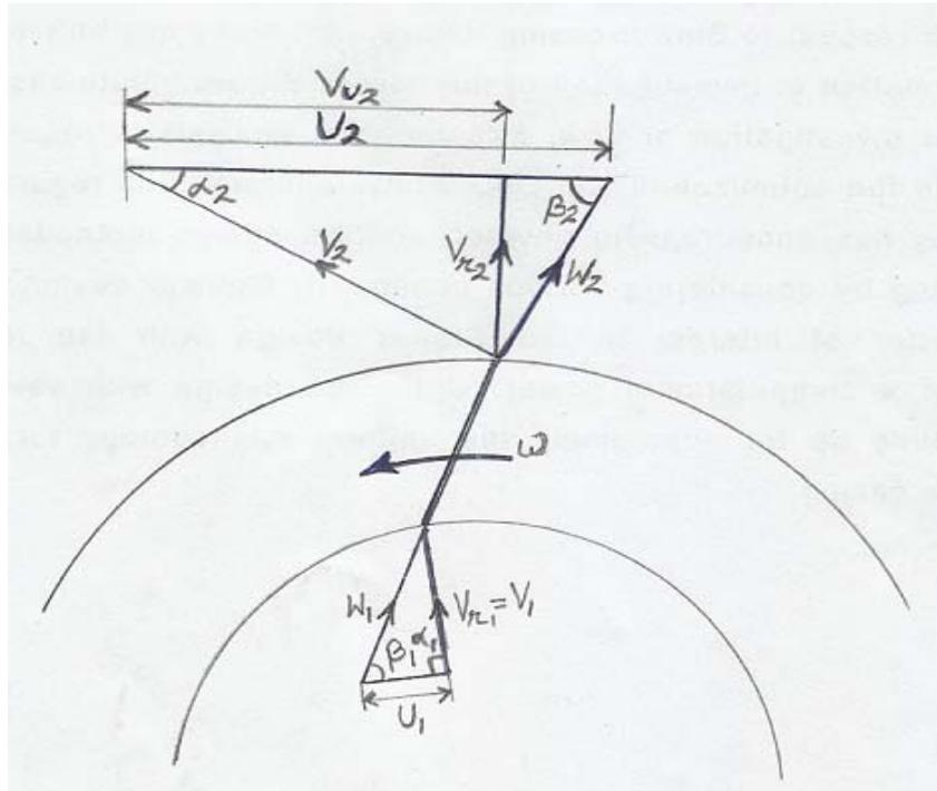
Figure: 3.5 Inlet and Outlet Velocity Diagram for impeller.
