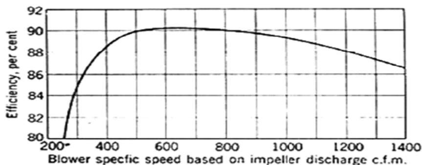
Figure: 3.1 Specific speed versus efficiency.
