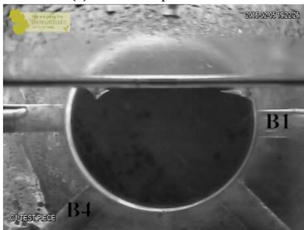
(c) Disappearance of unsteady flow at B1
