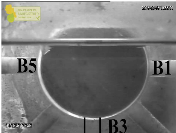
(k) Disappearance of unsteady flow at B5
