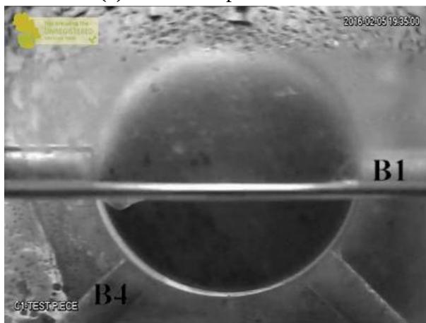
(g) Disappearance of unsteady flow at B4
