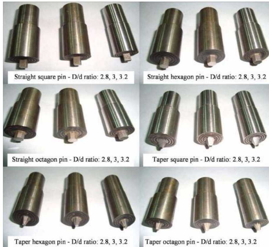
Figure 2.23: Tools with different amount of flat faces [50]
