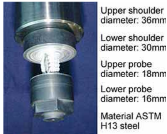
Figure 2.26: BFSW tool used by Threadgill et al. [13] to weld 25 mm thick, AA6082-T6 Aluminium Alloy.
