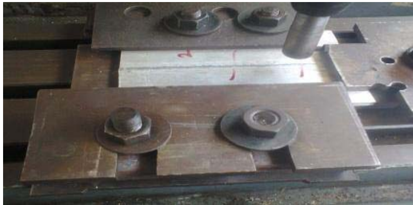
Figure 2.7: Setting the Al plates in Universal Milling Machine [35]
