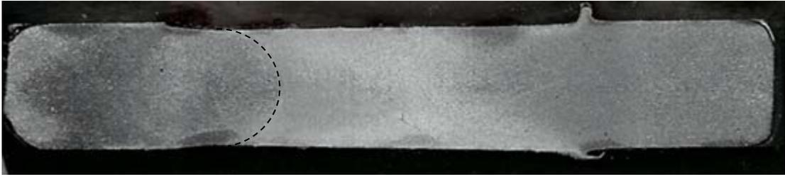
Figure 4.88: Image of sample welded by BFSW at 1000rpm and 24mm/min (as polished)
