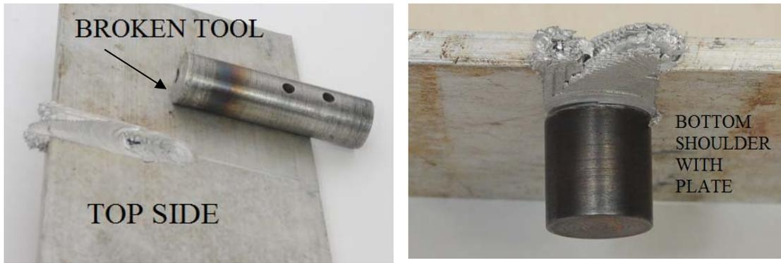
Figure 4.24: Failure of cylindrical bobbin tool during welding
