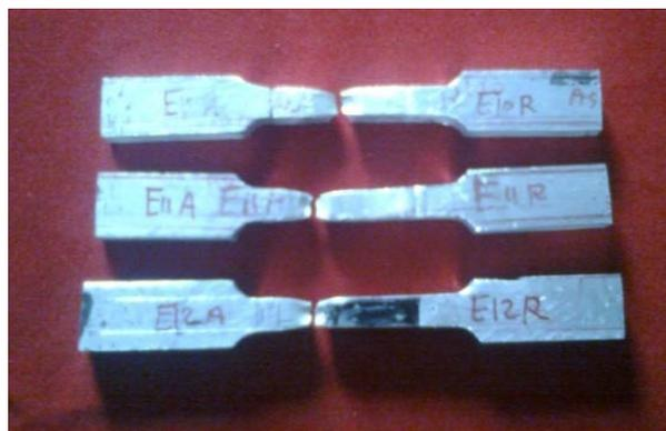
Figure 4.8: The Tensile test specimen after test - welded by square tool pin profile
