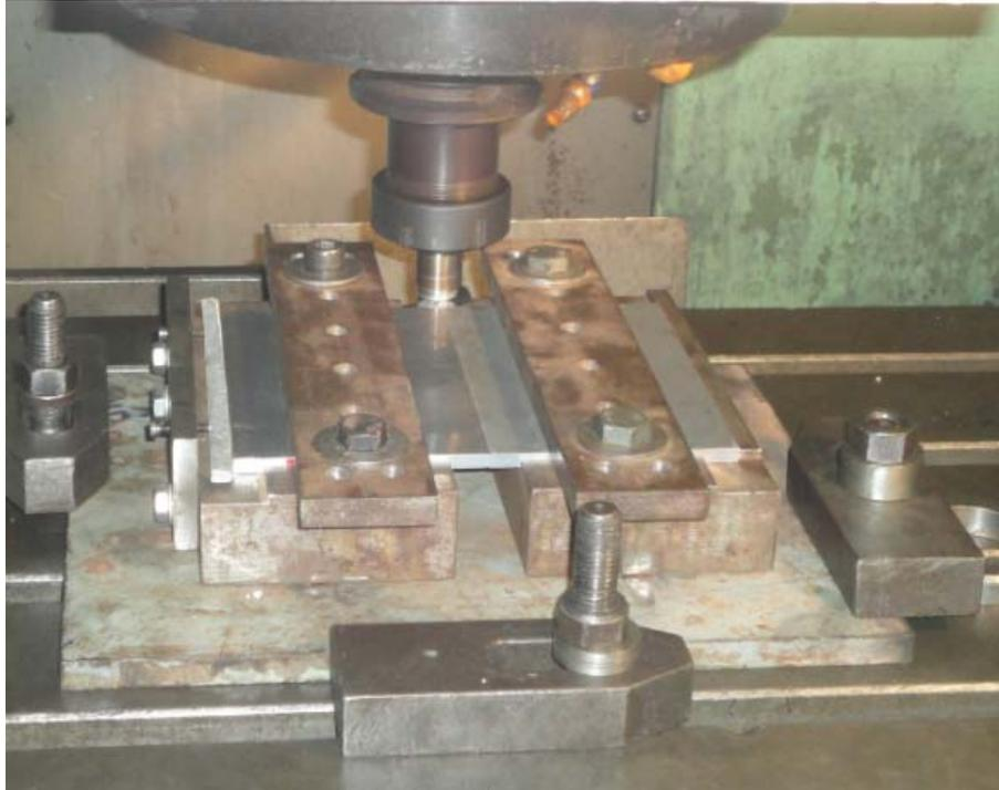
Figure 4.5: Fixture for bobbin friction stir welding (BFSW fixture)
