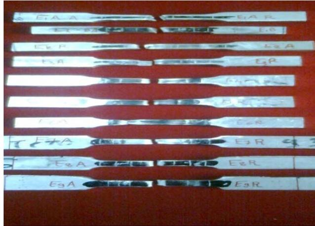
Figure 4.7: The Tensile test specimen after test - welded by hexagonal tool pin profile
