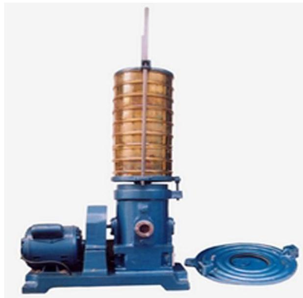
**Fig. 3.1: Vertical Sieve Shaker**
