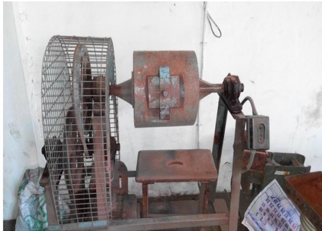
**Fig.3.2: Laboratory Ball Mill**
