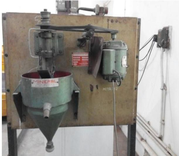
**Fig. 3.6: Laboratory Hydro-cyclone**
