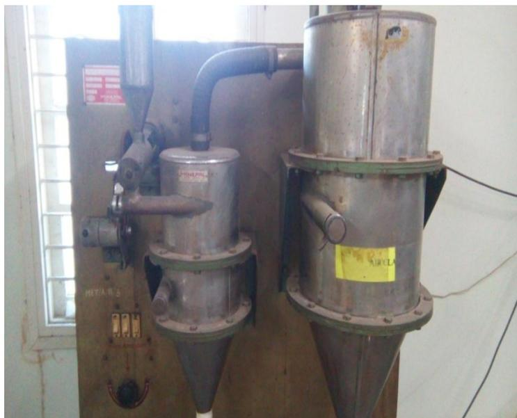
**Fig.3.4: Laboratory Air Classifier**
