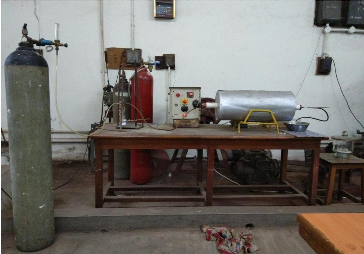
**Fig. 4.16: Experimental set-up for isothermal reduction of composite pellets**
