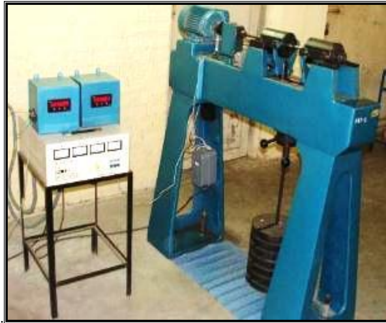
Fig.3.8: Close-up view of fatigue testing machine showing loading system, controller and digital counter
