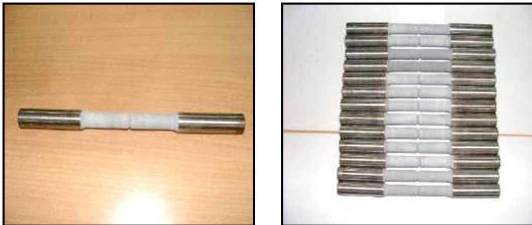
Fig. 3.3: Close-up views of alumina coated specimens produced by thermal spraying
