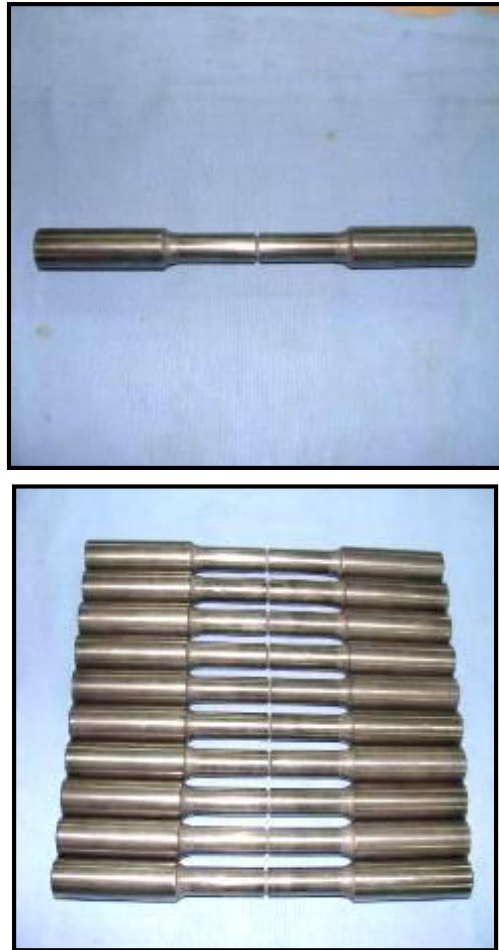
Fig. 3.5: Pictorial view of a plasma nitrided specimens
