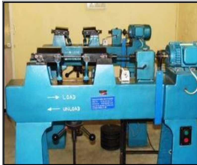
Fig. 3.7: Pictorial view of the rotating bending fatigue machine (Numbers of machines installed : 4)
