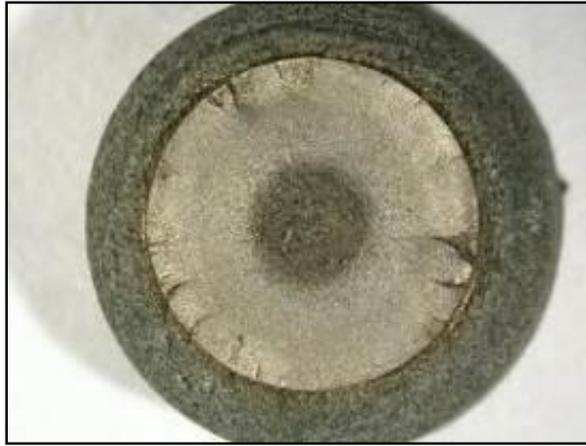
**Fig. 4.42:** Macrofractograph of fatigue tested thermally sprayed specimen demonstrate the multiple origin type of fracture under fatigue.
