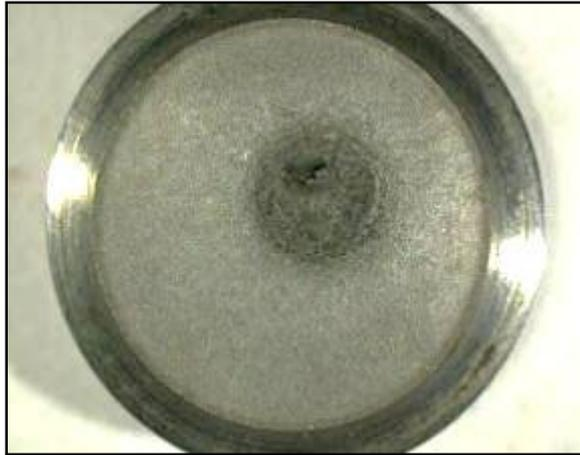
**Fig. 4.46:** Macrofractograph of fatigue tested plasma nitrided specimen with  $< 10 \mu\text{m}$  white layer thickness does not show any peripheral ratchet marks on the fracture surface, presumably indicative of failure of the specimen due to initiation and propagation of a single crack leading to final separation
