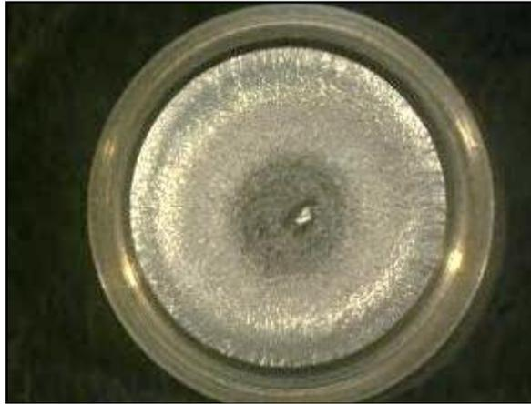
**Fig. 4.44:** Macrofractograph of fatigue tested plasma nitrided specimen with  $> 10 \mu\text{m}$  white layer thickness demonstrate the multiple origin type of fracture under fatigue.
