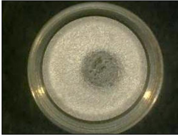
**Fig. 4.48:** Macrofractograph of fatigue tested plasma nitrided specimen without any white layer does not show any peripheral ratchet marks on the fracture surface, presumably indicative of failure of the specimen due to initiation and propagation of a single crack leading to final separation.
