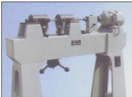
**Fig. 2.12: A pictorial view of a rotating bending type fatigue testing machine [Jinan co. China]**
