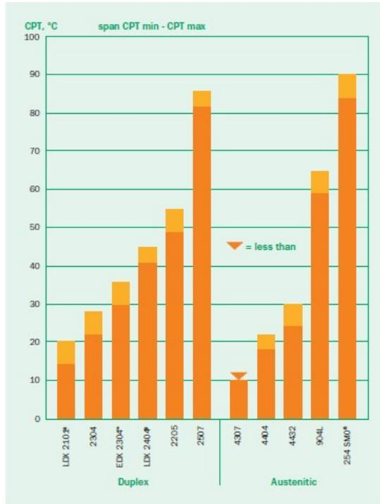
**Fig 2.23 Typical critical pitting corrosion temperatures (CPT) in 1M NaCl measured according to ASTM G 150 using the Avesta Cell. Test surfaces wet ground to P320 mesh. CPT varies with product form and surface finish**
