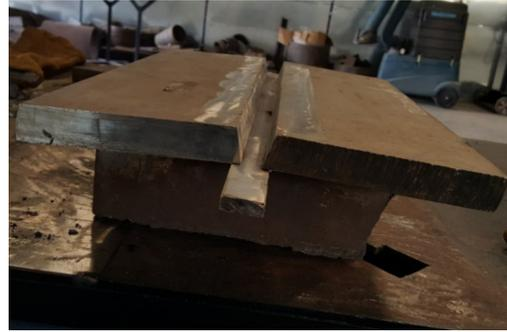
Fig. 3.5 C-Clamp Restraint (Front view)
