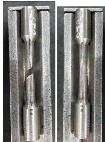
**Fig. 3.20 Fracture within Gauge length at 91740 N**
