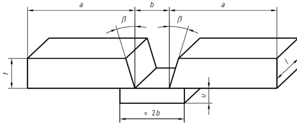
Fig. 3.1 Schematic of All weld metal test coupon preparation set up. Source[77]
