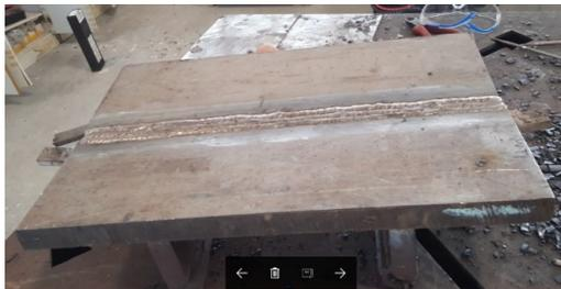
Fig. 3.8 Fill Pass completed
