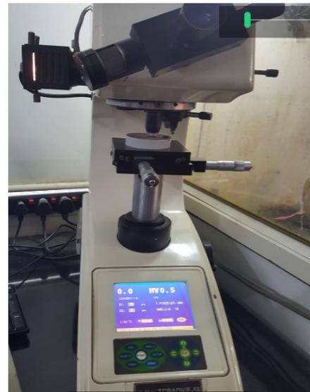
**Fig 3.29 Specimen being measured for micro hardness at different 12 locations with 500 gmf load according to AS PER E-384, EN ISO 9015-1:2011**
