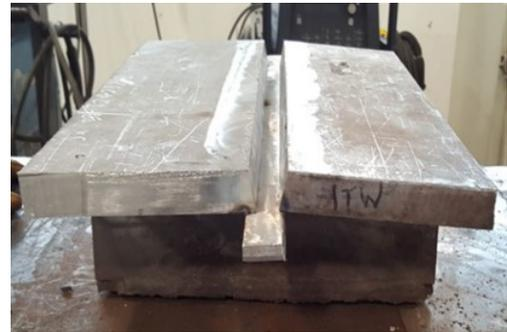
Fig. 3.7 Wire Brush finished test Piece
