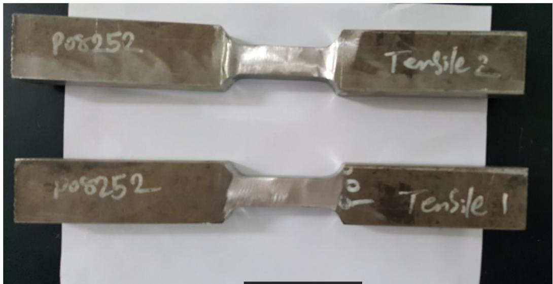
**Fig 3.23. (b) Preparation of Test Specimen for Transverse Tensile Testing as per AWS B4.0 [78]**
