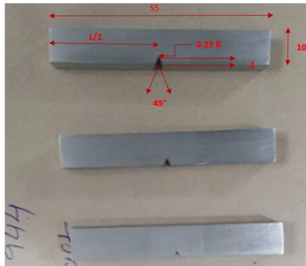
Fig 3.32 One Set (3 specimens) for V Notch Charpy Impact Test as per ASTM A 370-14
