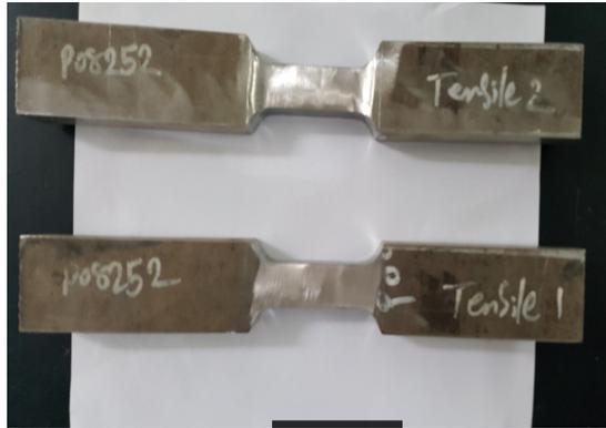
**Fig 3.24 Transverse Tensile Specimen before fracture**
