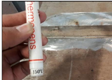
**Fig. 3.12 Application of templic to control less than 150 °C inter pass temperature.**
