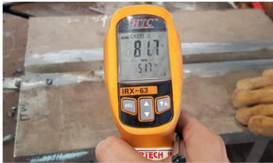
**Fig. 3.11 Application of digital thermometer to control less than 150 °C inter pass temperature.**
