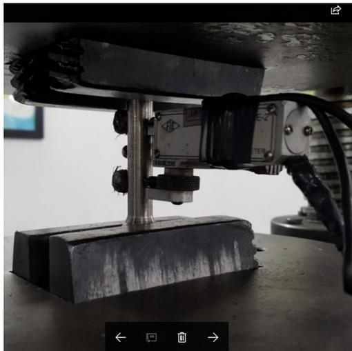
**Fig. 3.19 Specimen under Tensile load of UTM Machine with 40 Ton capacity**
