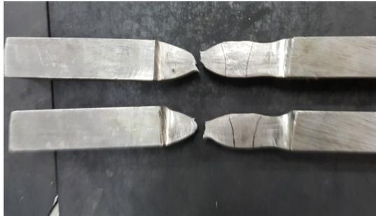
**Fig 3.26 Transverse Tensile Specimen After fracture Dimension**
