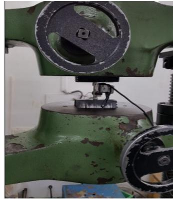
**Fig 3.25 Specimen under Tensile load Press capacity 60 Ton Capacity**
