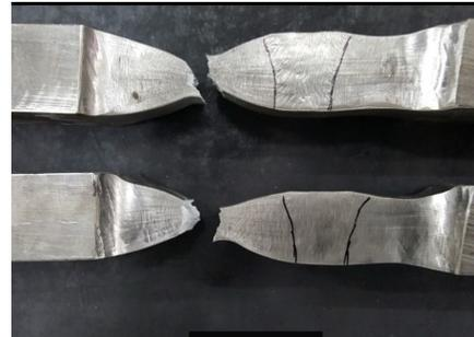
**Fig 3.27 Fractured specimen shows fracture from the P.M.**
