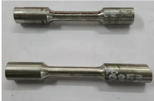
**Fig. 3.17 Prepared specimen for All weld Test**
