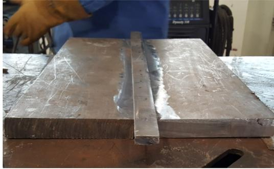
Fig. 3.4 Backing Strip Weld
