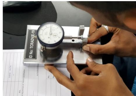
**Fig 3.36 Measurement of Lateral Expansion by dial gauge.**
