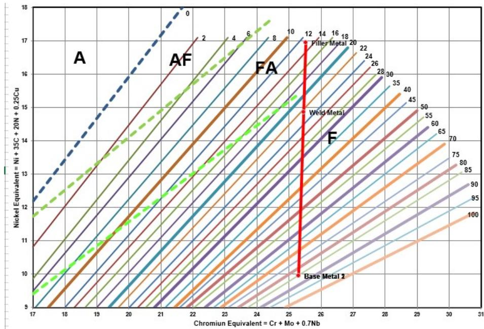
Fig 3.40 WRC -1992 DIAGRAM PREDICTING FN 22
