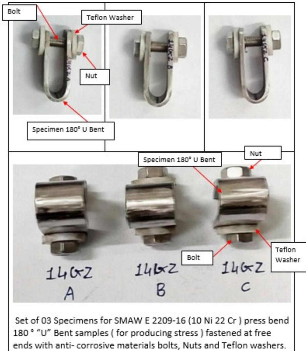
**Fig. 3.42 Set of 03 specimens for SMAW E 2209-16 ( 10 Ni 22 Cr ) press bend 180° "U" bent samples (for producing stress) fastened at free ends with anti-corrosive materials bolts, Nuts and Teflon washers.**
