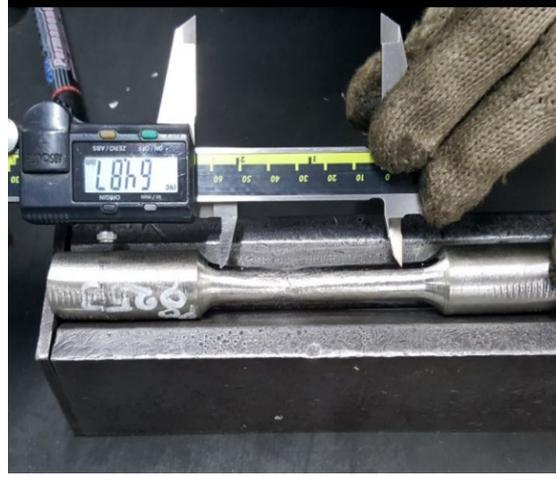
**Fig. 3.22 Final Length Measurement : 64.87 mm**
