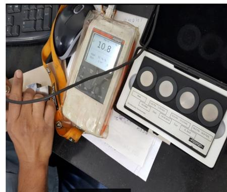
**Fig 3.38 Calibrated Fischer Ferriscope® Germany Make: Fischer 2531**
