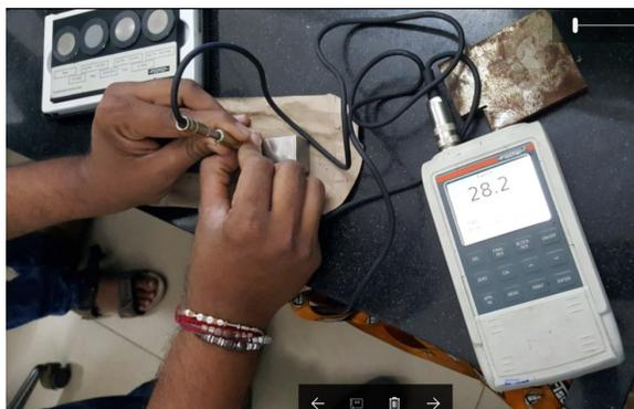
**Fig 3.37 Instrument utilized was Fischer Ferriscope® Germany Make: Fischer 2531**
