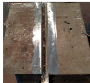
Fig. 3.9 Root pass completed
