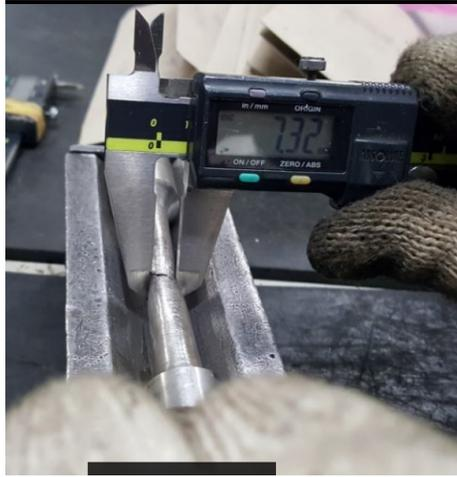
**Fig. 3.21 Final Diameter 7.32 mm measurement.**
