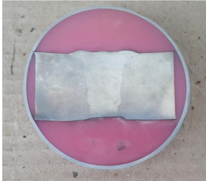
**Fig 3.27 (a) Specimen for Micro hardness measurement**
