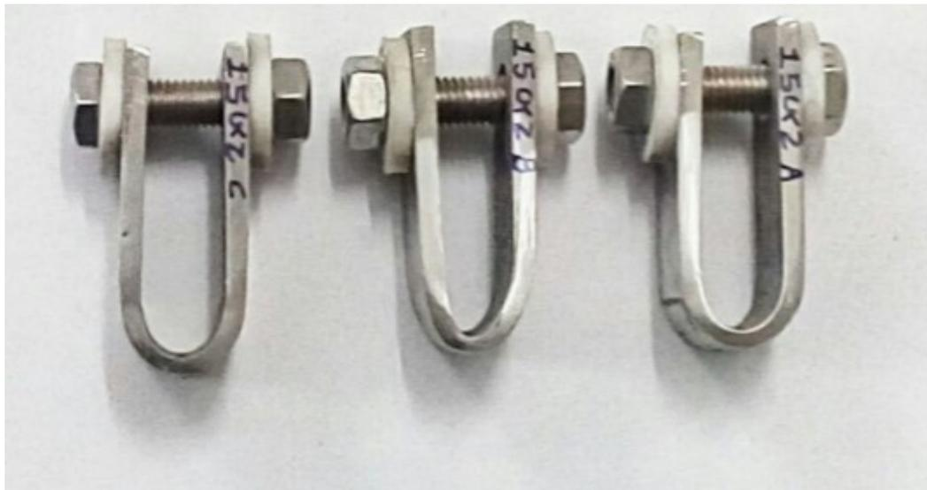
**Fig. 3.43 Set of 03 Specimens for SMAW E 2209-16 (11 Ni 22 Cr ) press bend 180 °
