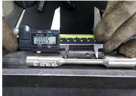
**Fig. 3.18 Initial gauge length measurement ~ 50 mm**
