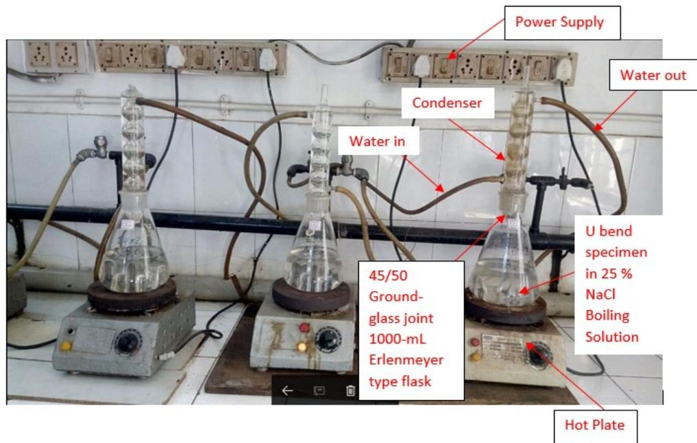
**Fig. 3.45** Set of Specimen (03 Nos. Per Heat) immersed in boiling 25 % NaCl Solution (120-150 °C) in each flask on Hot Plate equipped with Condenser arrangement. Cycle time 1000 Hrs. (ASTM G123 )
