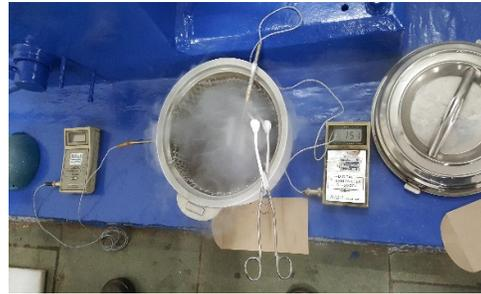
**Fig 3.34 Test temp -46 °C maintained by Liquid N2, Temperatures monitored by thermocouple**
