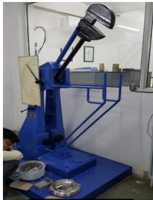
**Fig 3.35 Impact Test Machine Capacity 350 Joule**
