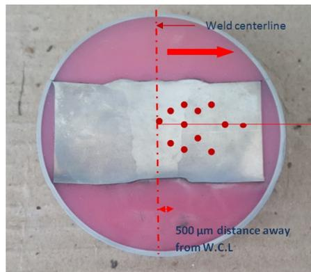
**Fig 3.28 micro hardness at 12 locations away from weld centre line**
