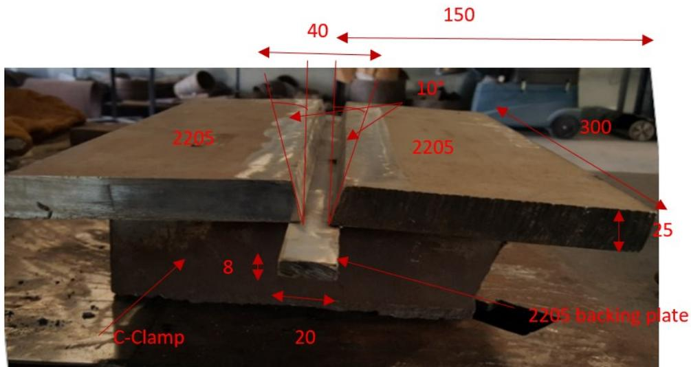
Fig. 3.2 Weld Test Coupon prepared for welding
