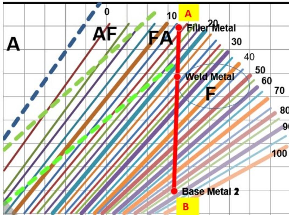
**Fig 3.41 Calculation of Ferrite Number from WRC 1992 diagram Enlarged view indicating approx. FN 22**
