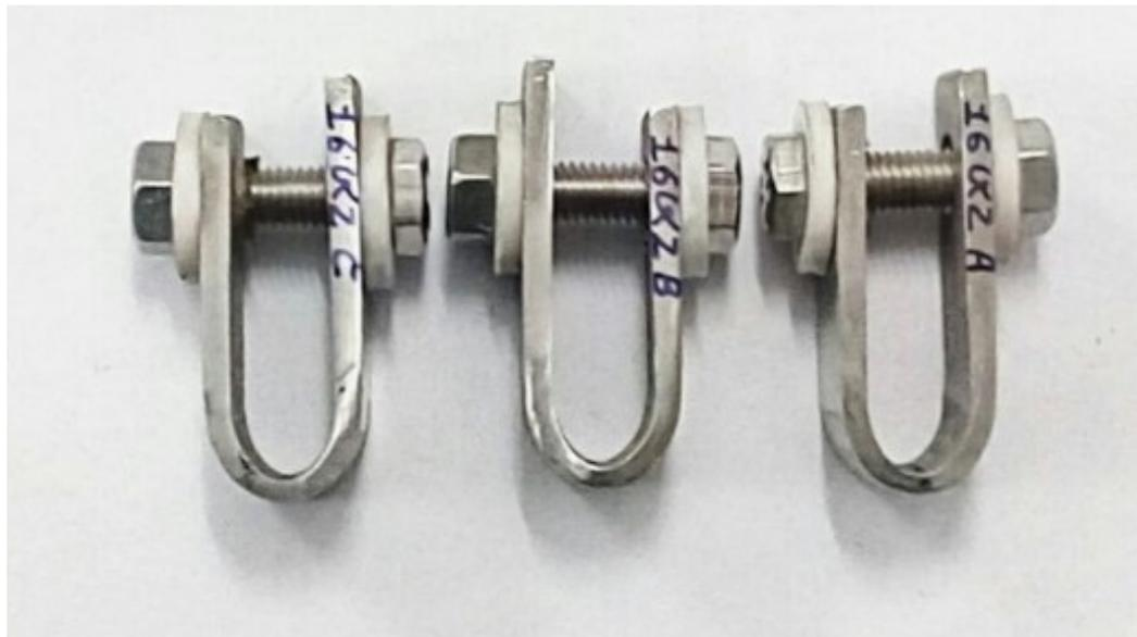
**Fig. 3.44 Set of 03 Specimens for SMAW E 2209-16 (12 Ni 22 Cr ) press bend 180 ° “U” Bent samples ( for producing stress ) fastened at free ends with anti-corrosive materials bolts, Nuts and Teflon washers.**
