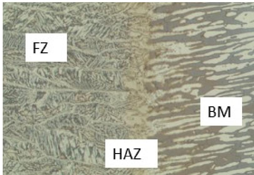
**Fig.5.16 sample id 11 Ni 22 Cr across fusion boundary showing fine grain austenite in fusion zone Weld Micro at 200 X Mag. NaOH etched**
