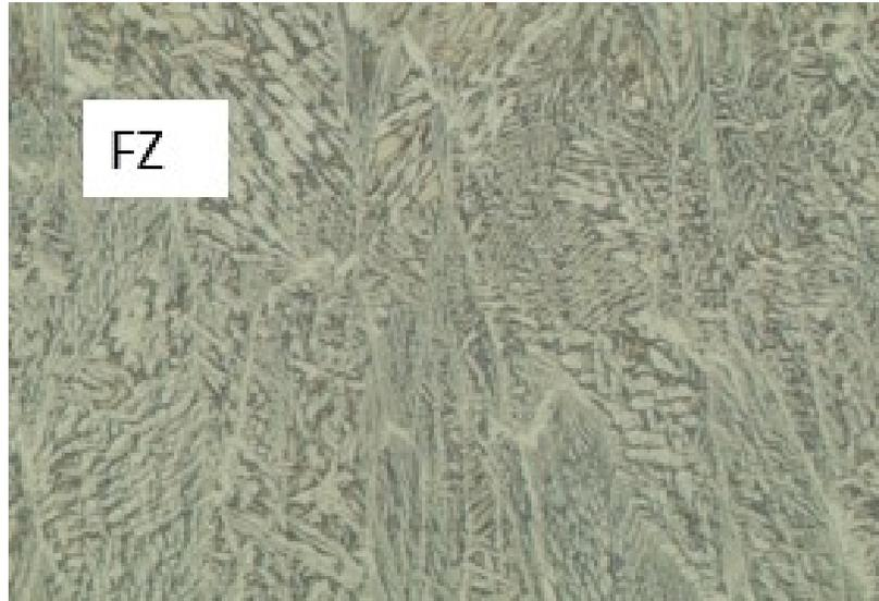
**Fig. 5.15 sample id 11 Ni 22 Cr Micro at 200 x Magnification,NaOH etched light phase austenite (WA) and ferrite (dark phase)**
