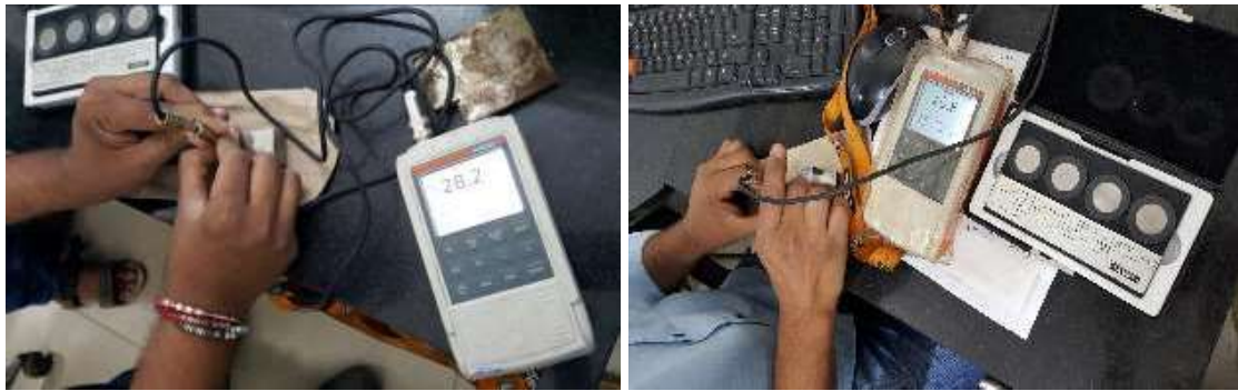
Fig 1 : Calibrated Fisher Feritscope Instrument Model Fischer 2531
