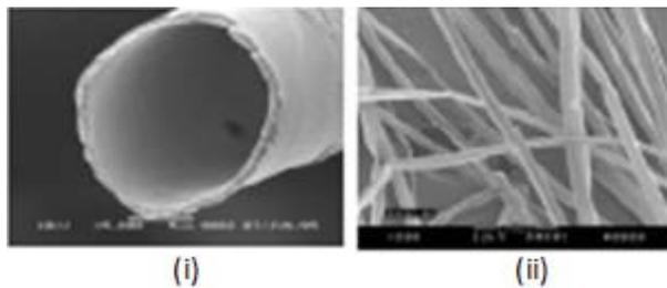
**Figure 3.1:** SEM of kapok fibre. (i) Kapok fibre cross-section (ii) Kapok fibre surface
