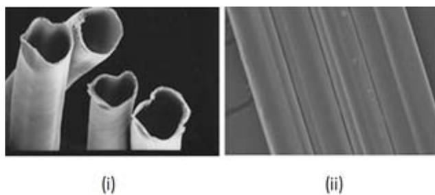
**Figure 3.2:** SEM of milkweed fibre (i) Milkweed fibre cross-section (ii) Milkweed fibre surface
