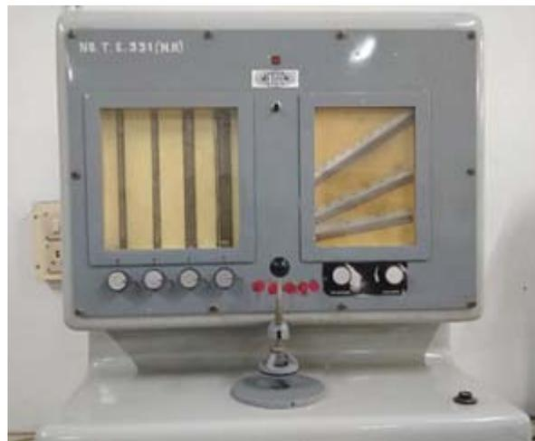
**Figure 3.13:** Air permeability tester
