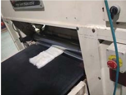
**Figure 3.10:** Image of web feeding in needle punch machine
