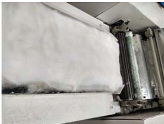
**Figure 3.9:** Image of sandwich web passed through a miniature carding machine
