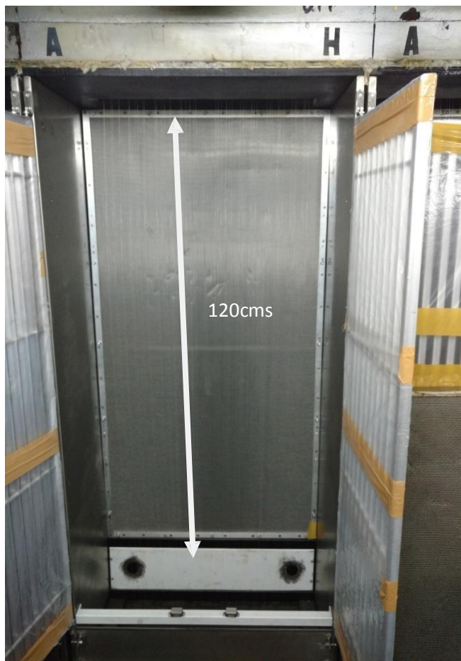
Quench screen length before modification (Length = 120 cm)
