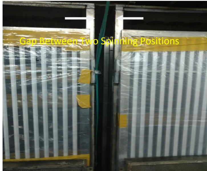
Fig.4.4: Quench chambers of two adjacent positions before increasing width of quench screen
