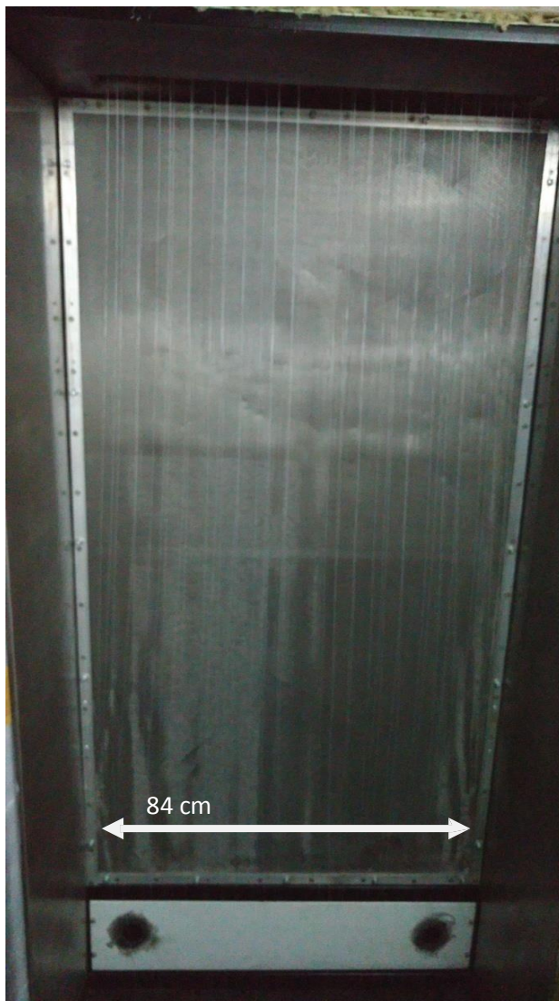
Quench screen before modification (Width = 84 cm)
