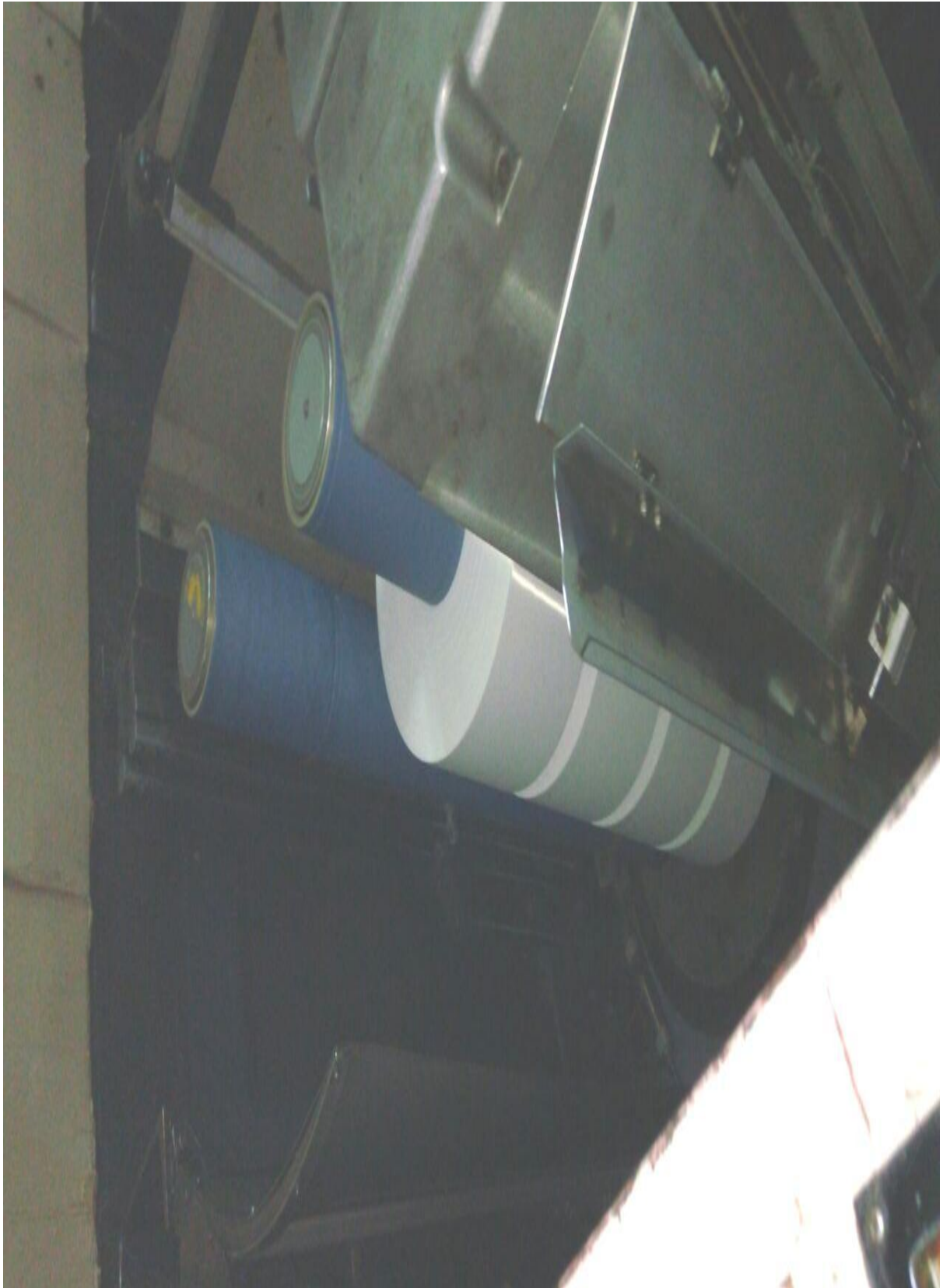
Fig.4.12: Modified take-up with 4 ends winder
