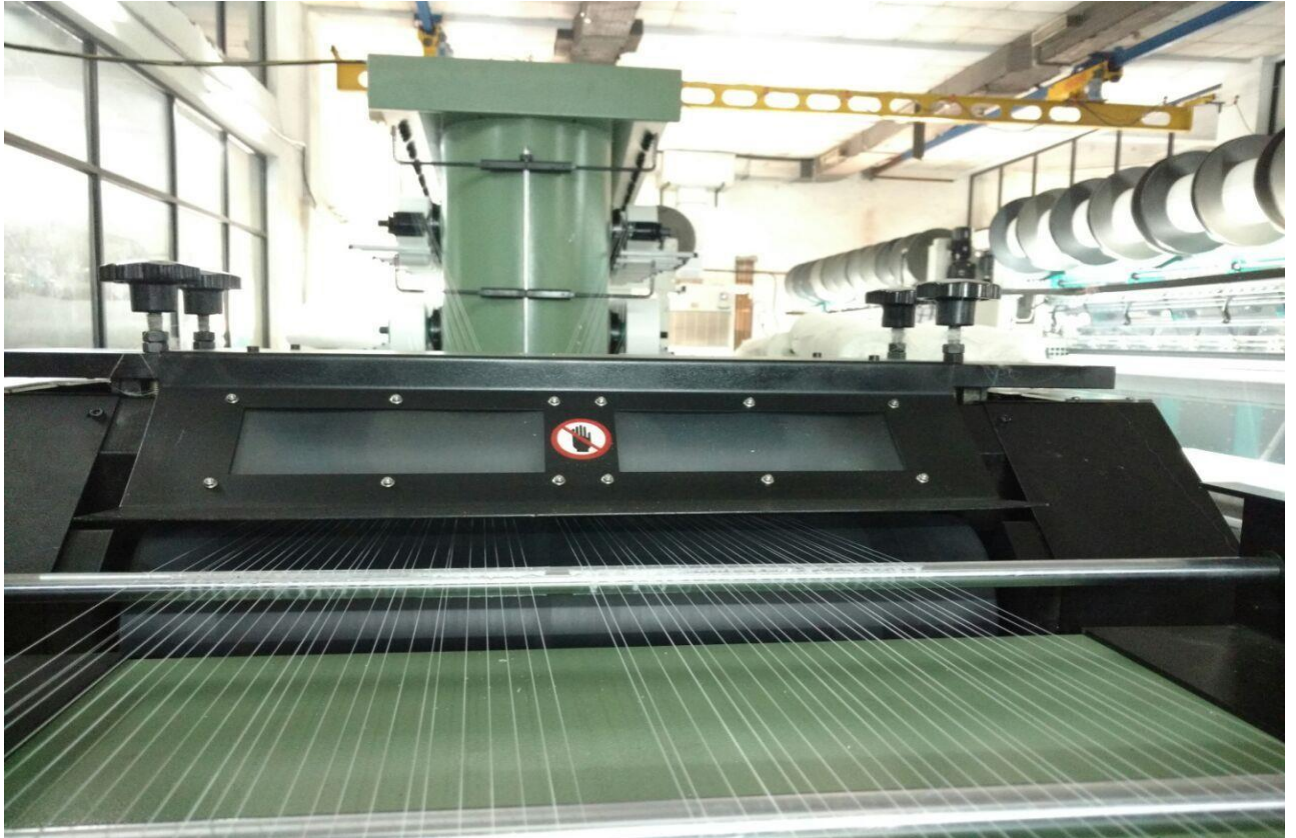
Fig 4.17 Monofilament formation process at warp splitter
