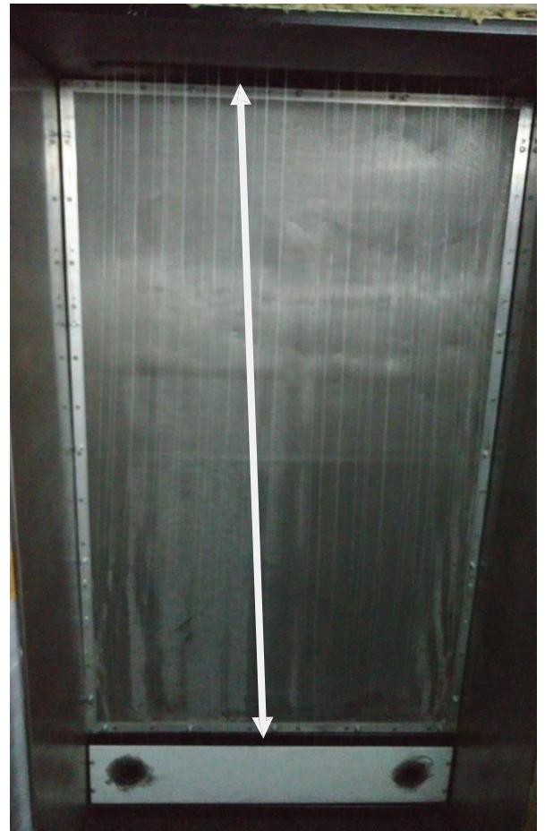
Modified quench screen (Length = 200 cm)
