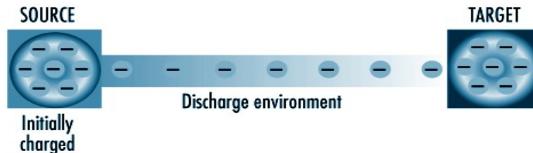
Fig. 2.2 – Schematic of electrostatic discharge problem
