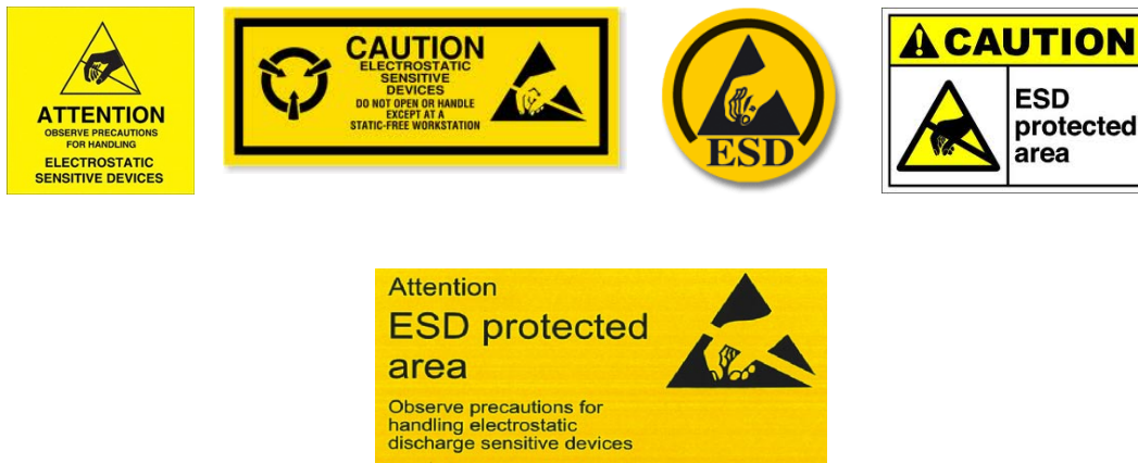
Fig. 2.3 – Examples of ESD indicators/labels
