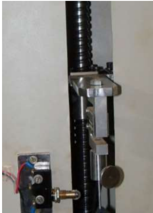
Fig 3.14: Load cell attached to clamp
