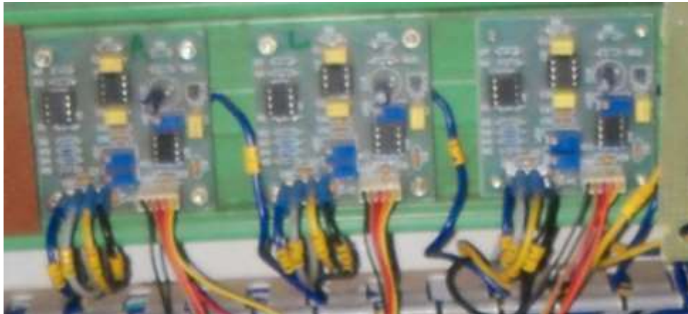
Fig 3.28: Analog to digital card interface with LabJack
