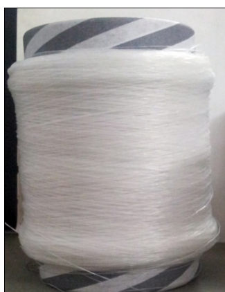
g) Polypropylene and 1.25% SiO 2 filament (NPP6)
