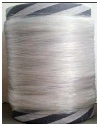
e) Polypropylene and 0.7% SiO 2 filament (NPP4)
