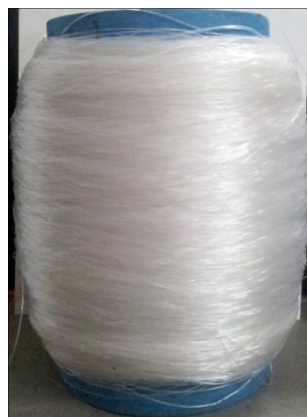
b) Polypropylene and 0.1% SiO 2 filament (NPP1)
