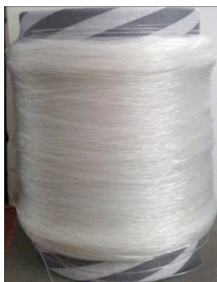
d) Polypropylene and 0.5% SiO 2 filament (NPP3)
