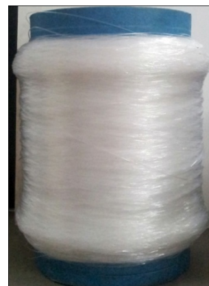
c) Polypropylene and 0.3% SiO 2 filament (NPP2)
