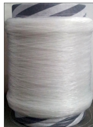
f) Polypropylene and 1.0% SiO 2 filament (NPP5)
