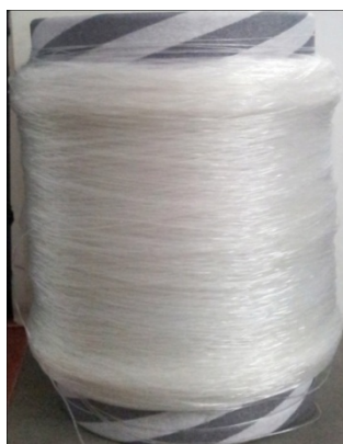
d) Polypropylene and 0.5% SiO 2 filament (NPP3)
