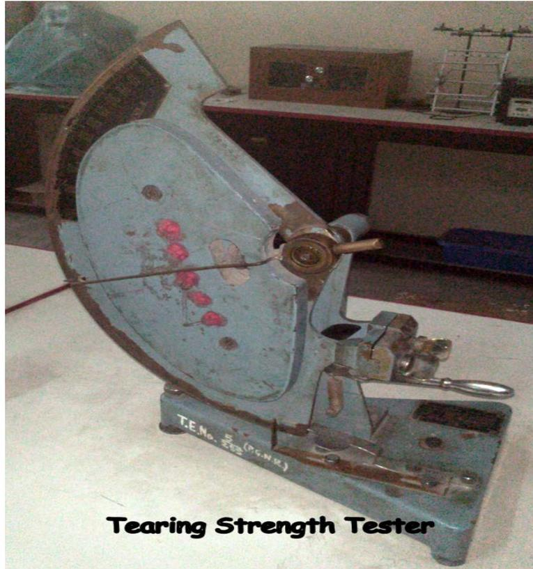
*Figure 3.12 Elmendorf tear strength tester*
