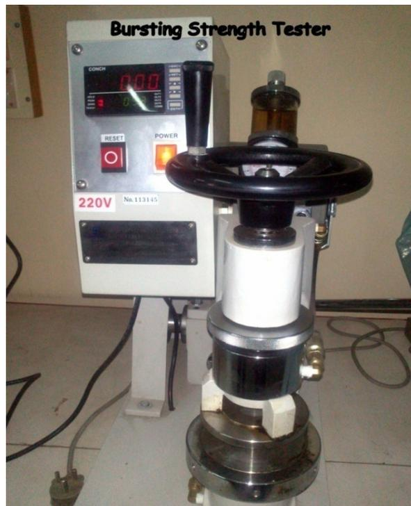
*Figure 3.13 Bursting strength tester*
