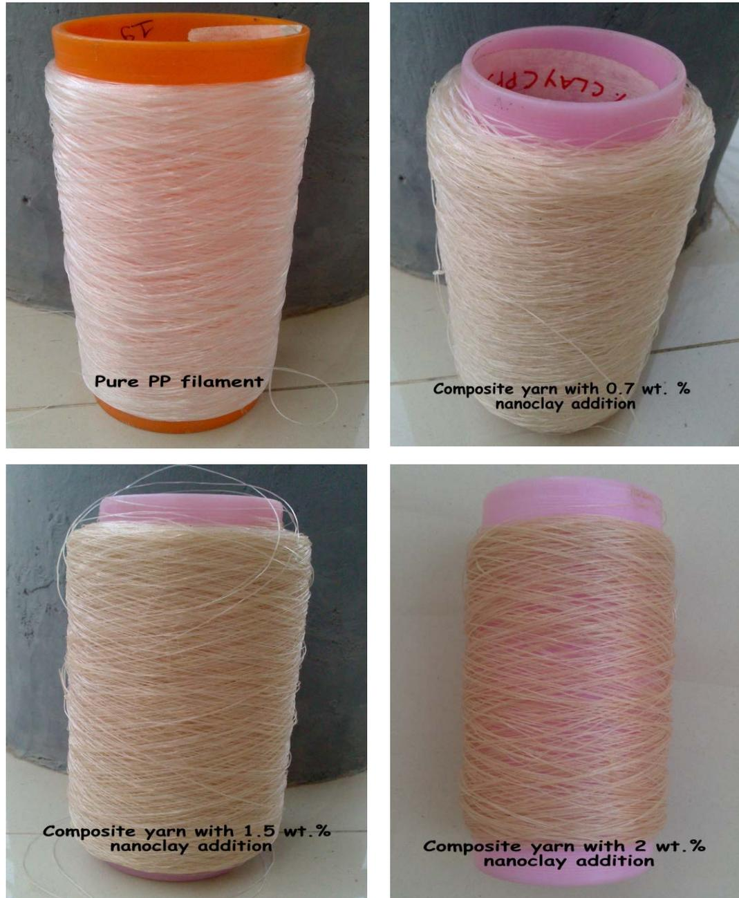
*Figure 4.8 Photographs of pure polypropylene and polypropylene / nanoclay composite filament*
