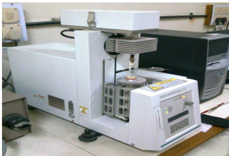
*Figure 3.5 Photograph of Shimadzu TGA-50 thermal analyzer*
