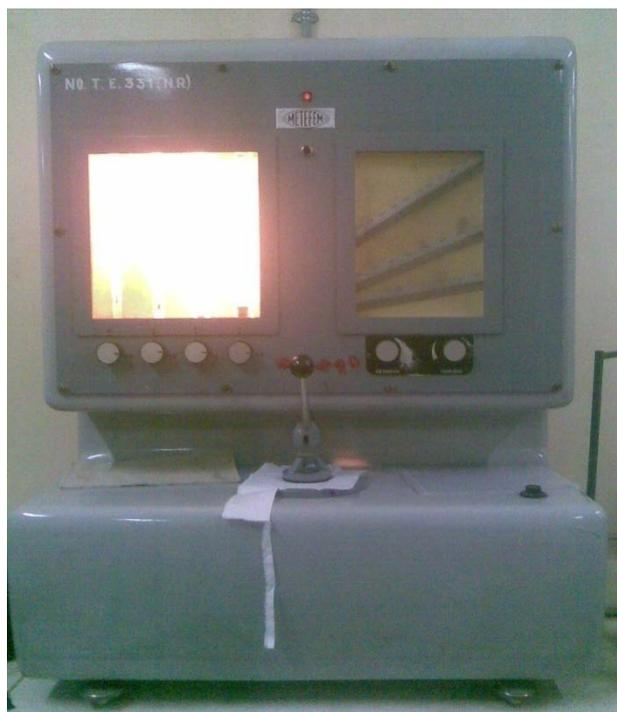
*Figure 3.15 Metefem Air Permeability Tester*
