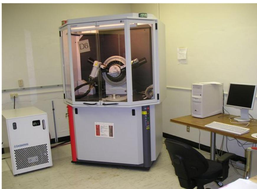
*Figure 3.6 Photograph of Diffractometer D8 advance with CuK  $\alpha$  radiation*
