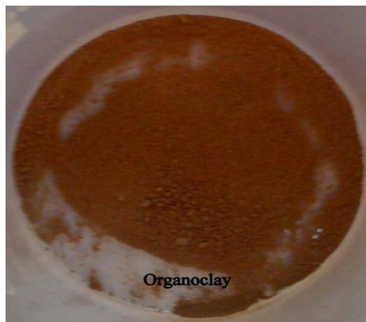
*Figure 4.2 Photograph of Organoclay nano particles prepared from Na-MMT clay using CTAB*
