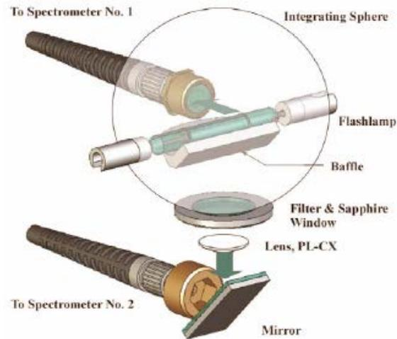
*Figure 2.19 UV-2000F Ultraviolet Transmittance Analyzer*
