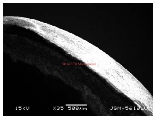
Figure 6 - 4 SEM Image of cross section of exhausted shell after dissolution
