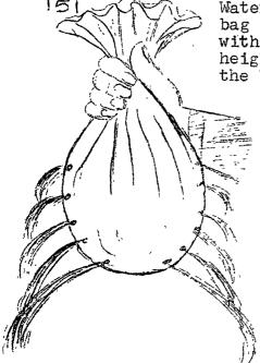
Water is poured into a heavy paper bag. The bag is lifted carefully and four holes are punched with a needle with 1" different at different heights on both sides. Water from the holes near the bottom is seen to gush farther. It shows that
