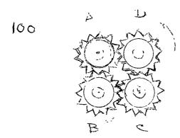
As the wheel 'D' rotates in the direction shown how do the wheels A and B move?
