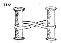
As the second pulley 'B' rotates in clockwise direction the first one
