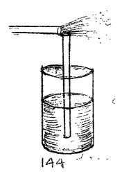
Two soda straws, one placed in water vertically and the other kept horizontally normal to the first one and just above it. Through the straw kept horizontally, air is blown. Water gets sprayed. It denotes that the
