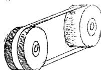
The belt driven mechanism is used because of its
