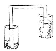
A bent glass tube when placed in the first position shown no water flowed. In the second position water continued to flow in the direction indicated. It is to be concluded that water
