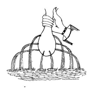
Water is poured into a heavy paper bag. The bag is lifted carefully and four holes are punched with a needle at one inch difference at different heights on both sides as shown. Water from the holes near the bottom is seen to gush farther.
