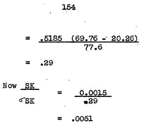
From the table of testing significance, it can be seen that this value is not at all significant. Hence 0.0015 represents no real deviation of the frequency distribution from normality.
