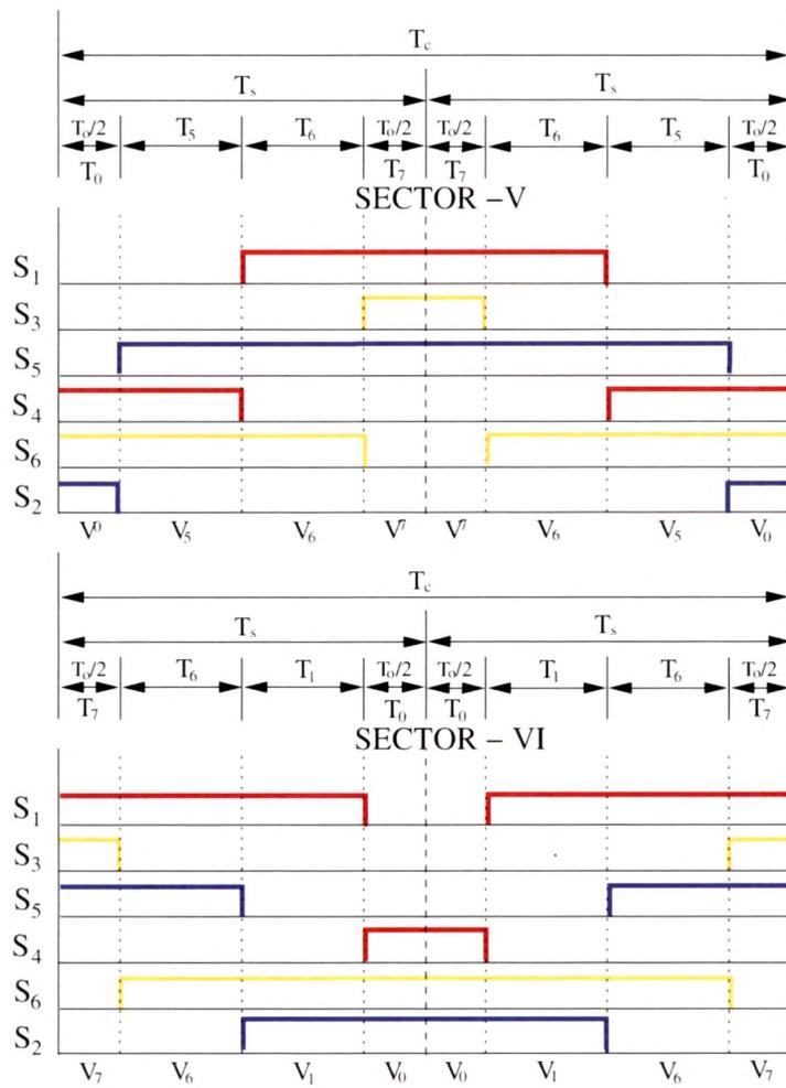
Figure 2.11: Optimal Switching Sequences for Sector V & VI
