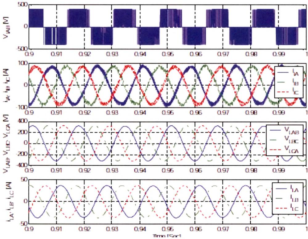
Figure 2.17: Simulation Waveforms. (a) Inverter Output Line to Line Voltage ( $V_{LAB}$ ) (b) Inverter Output Current ( $i_{iA}$ ) (c) Load Line to Line Voltage ( $V_{LAB}$ ) (d) Load Phase Current ( $i_{LA}$ )
