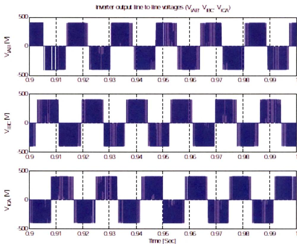
Figure 2.13: Simulation of Inverter Output Line to Line Voltages ( $V_{IAB}, V_{IBC}, V_{ICA}$ )
