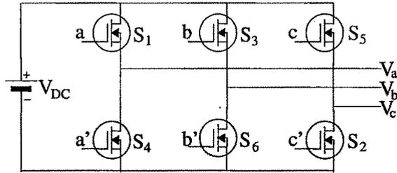
Figure 2.1: 3 Phase PWM Inverter Circuit for IDH
