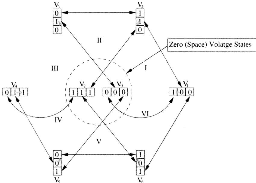
Figure 2.5: Transitions Between Different Switching States
