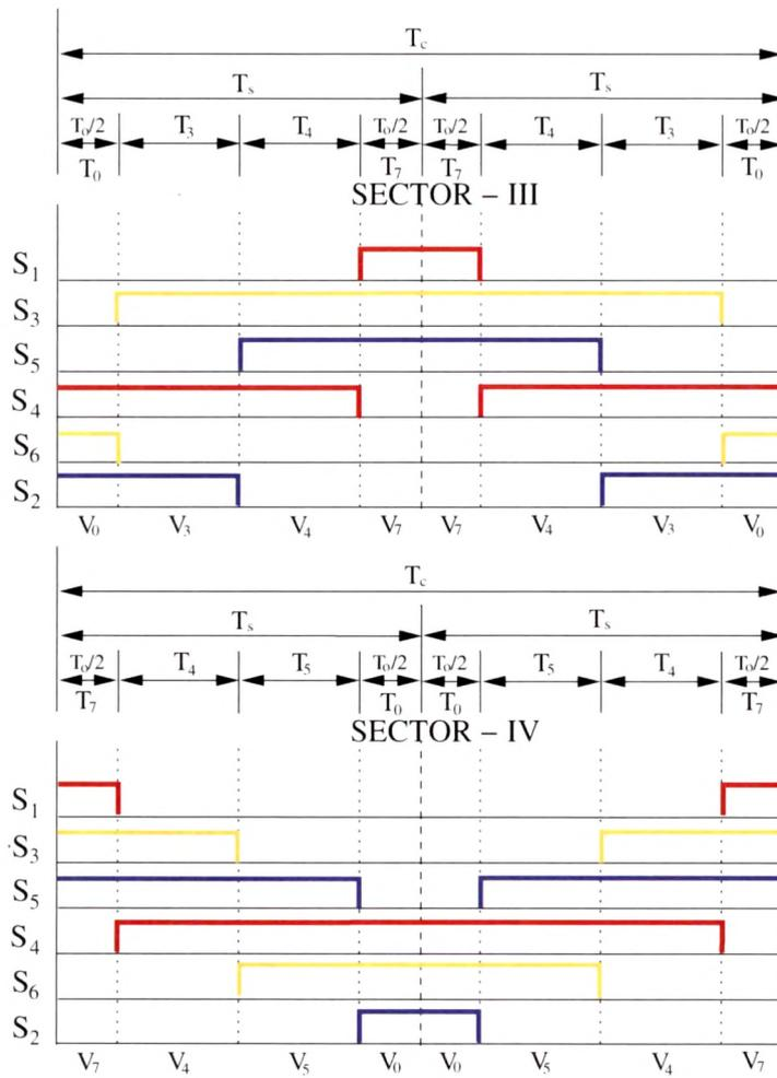
Figure 2.10: Optimal Switching Sequences for Sector III & IV
