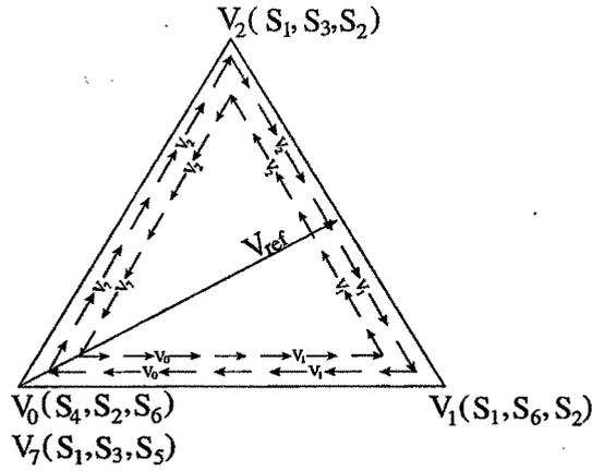
Figure 2.6: Optimal Vector Commutation for Sector I
