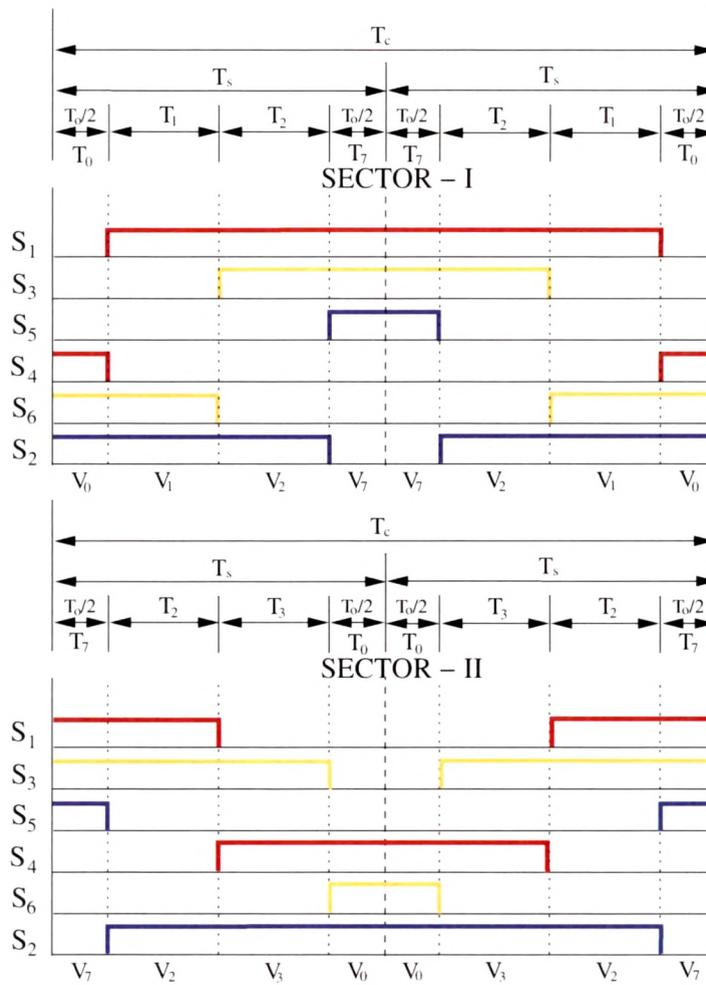
Figure 2.9: Optimal Switching Sequences for Sector I & II
