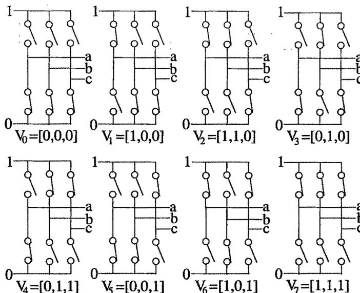
Figure 2.2: Eight Inverter Voltage Vectors
