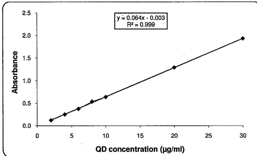
Figure 4.4 Standard curve of QD in Acetonitrile
