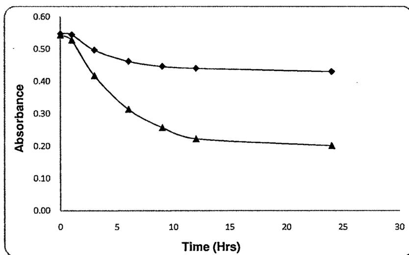
**Figure 4.9 Effect of 0.3mg/ml BSA on stability of QD in pH 7.4 Phosphate buffer**
