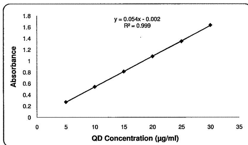
Figure 4.8 Standard curve of QD in pH 7.4 phosphate buffer
