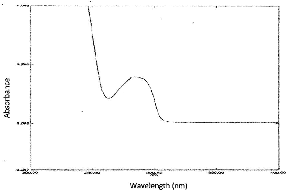
Figure 4.5 Absorptivity Scan of ET in pH 7.4 Phosphate Buffer
