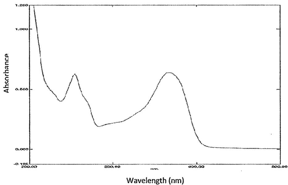
Figure 4.3 Absorptivity Scan of QD in Acetonitrile
