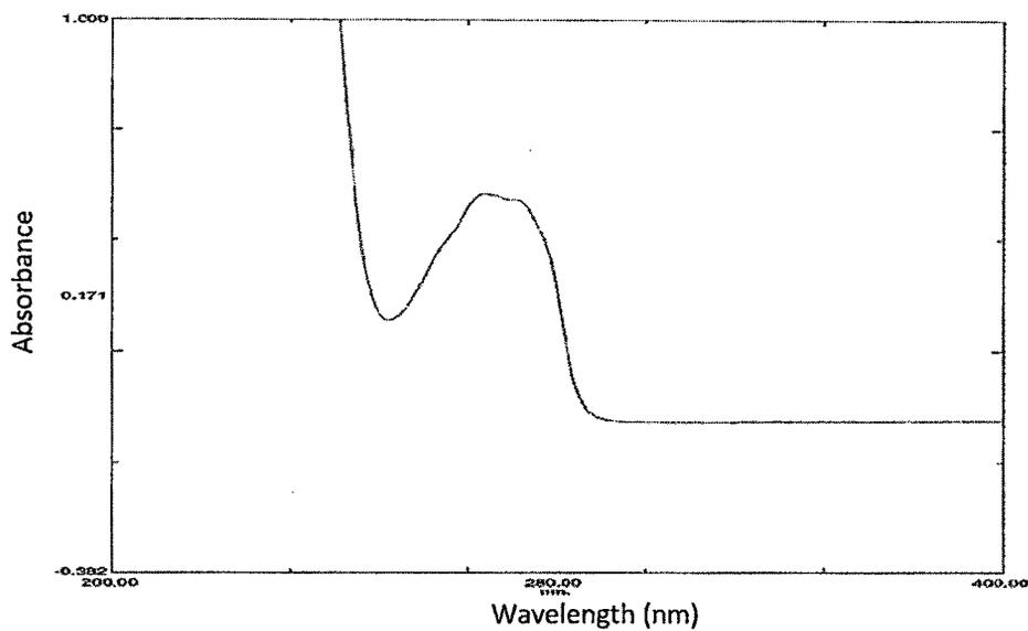
Figure 4.1 Absorptivity Scan of ET in Acetonitrile
