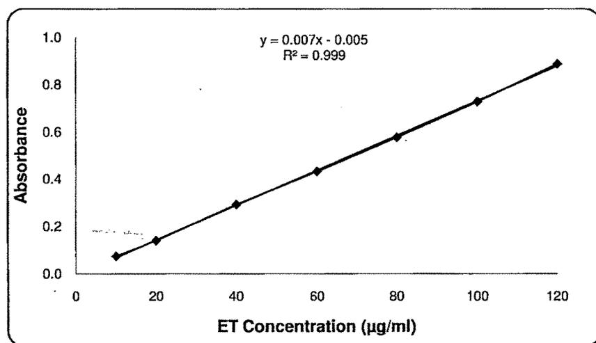
Figure 4.2 Standard curve of ET in Acetonitrile
