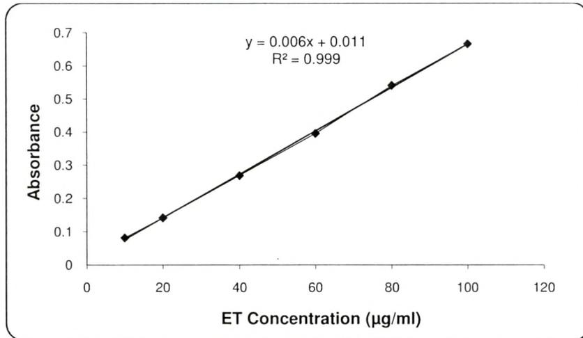
Figure 4.6 Standard curve of ET in pH 7.4 phosphate buffer
