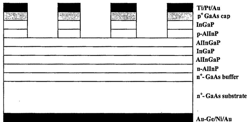
Figure 3.10: Laser diode structure after back contact.
