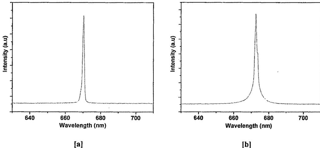
Figure 3.12: Laser diode spectra: [a] sample 2107086 [b] sample 2107088.
