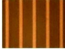
**Figure 3.7: Photograph of metal contacts on laser structure after lifting off.**
