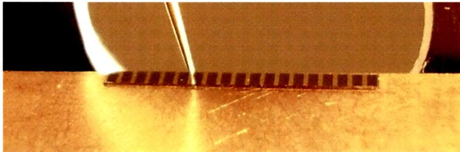
**Figure 3.3: A laser diode bar probed for characterization.**
