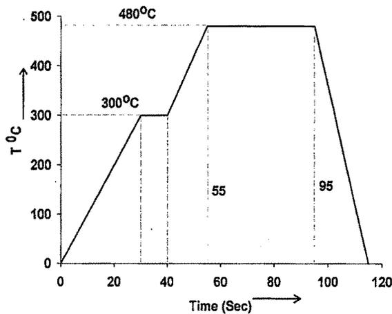
Figure 3.9: Temperature-time graph of RTA process.
