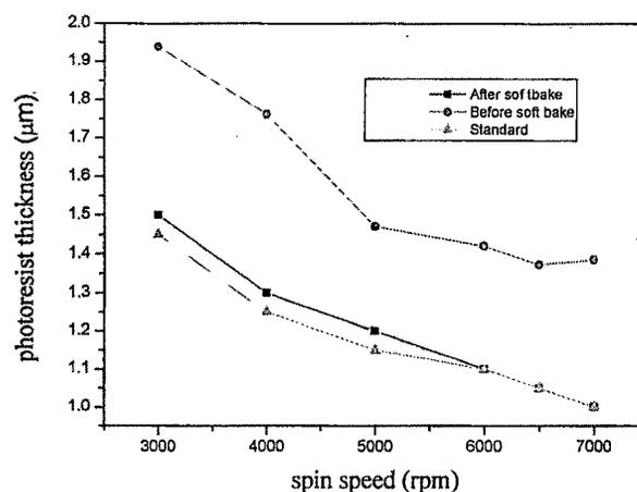
**Figure 3.5: Spin speed- thickness curves for S1813 photoresist :before softbake, after softbake and standard (from the catalogue).**
