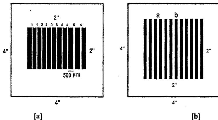
**Figure 3.6: Mask used in photolithography for laser diode stripe pattern; [a] variable-stripe width: No. 1 = 30  $\mu\text{m}$ , 2 = 50  $\mu\text{m}$ , 3 = 80  $\mu\text{m}$ , 4 = 100  $\mu\text{m}$ , and 5 = 200  $\mu\text{m}$ , [b] constant stripe-width.**
