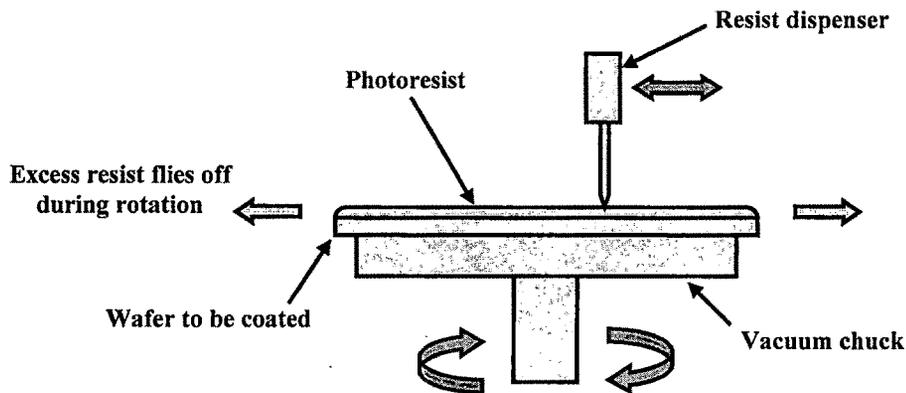
**Figure 3.4: Photoresist spin coating.**
