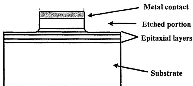
**Figure 3.2:** Schematic cross-section of index-guided mesa isolated stripe geometry laser diode.
