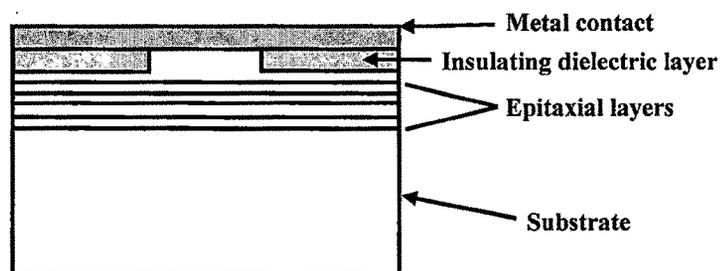
Figure 3.1: Schematic cross-section of gain-guided stripe geometry laser diode by dielectric insulation.
