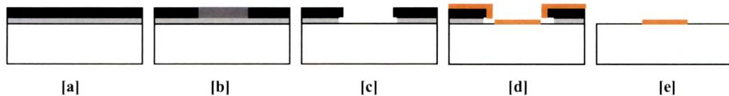
**Figure 3.8: Lift-off technique: (a) overlying layer of OiR 960 and underlying resist layer modified with chlorobenzene (b) area of OiR 960 resist exposed to UV (c) developed resist (d) following metal deposition (e) following lift-off and clean.**
