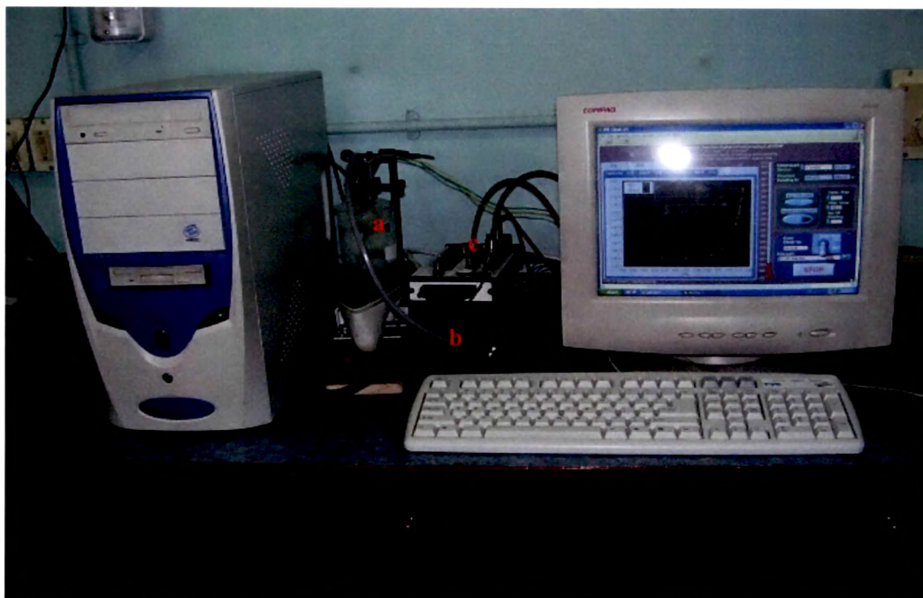
Figure 5.13: A DAQ system developed at our laboratory for semiconductor junction characterization.
