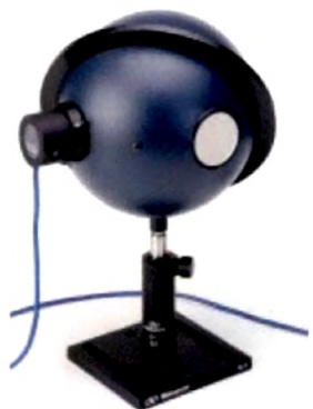
Figure 5.7: Photograph of integrating sphere with photodetector.
