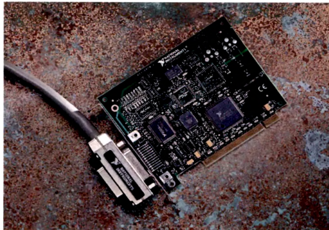
Figure 5.15: National Instruments' PCI-GPIB board with GPIB cable.
