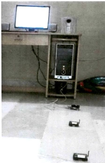
Figure 8.18(b): MICAz Nodes & Gateway Setup
