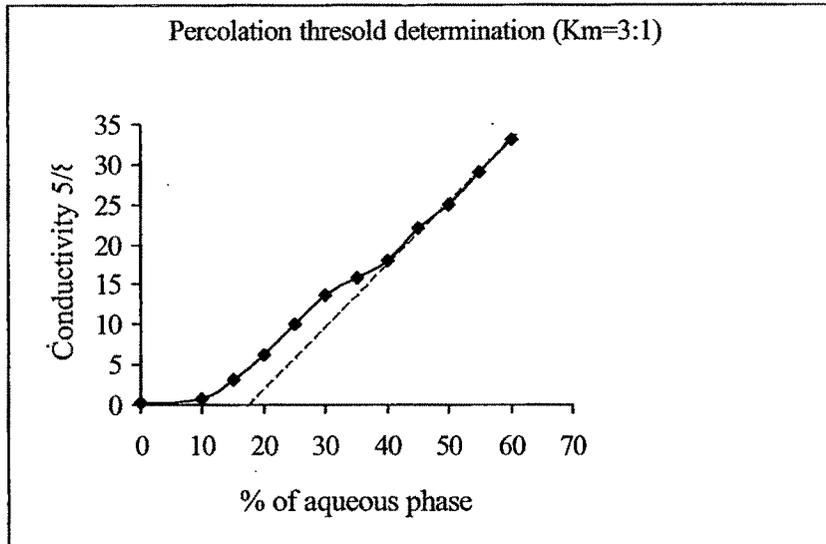
Figure 5.4: Percolation threshold determination of system A (ST/COST ratio=3:1)
