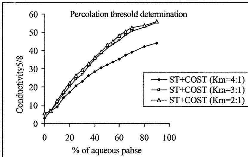
Figure 5.8: Percolation threshold determination of system C at different Km
