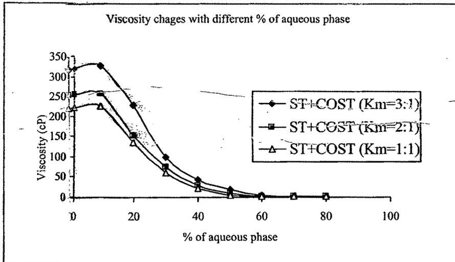
Figure 5.14: Viscosity changes with increasing water content at different surfactant to cosurfactant ratio ( $K_m$ ) (system D)
