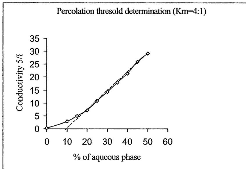
Figure 5.3: Percolation threshold determination of system A (ST/COST ratio=4:1)
