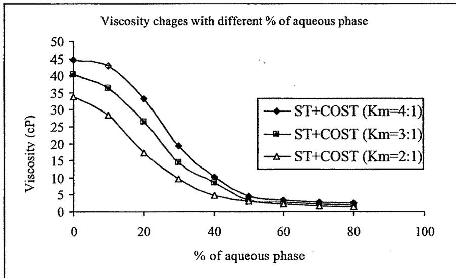
Figure 5.13: Viscosity changes with increasing water content at different surfactant to cosurfactant ratio ( $K_m$ ) (system C)
