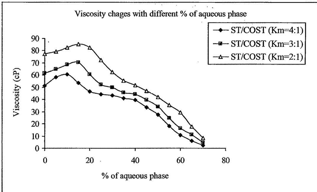
Figure 5.11: Viscosity changes with increasing water content at different surfactant to cosurfactant ratio (Km) (system A)
