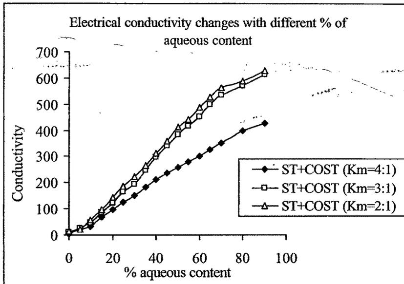
Figure 5.7: Electrical conductivity as a function of water content (System C)
