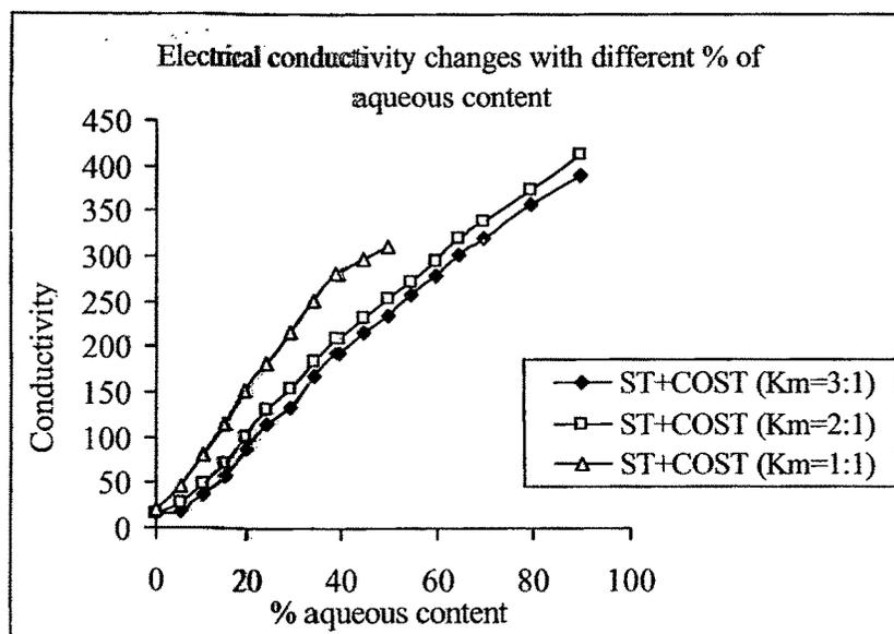
Figure 5.9: Electrical conductivity as a function of water content (System D)
