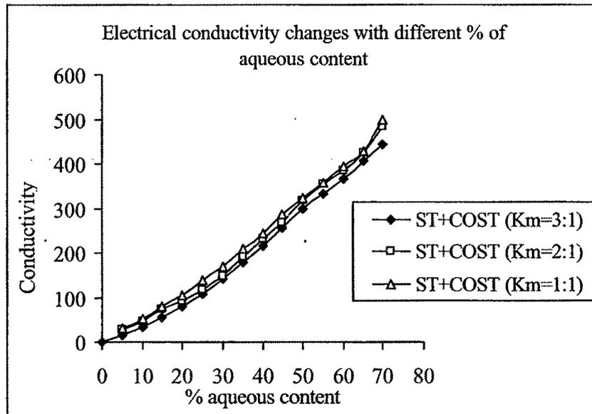
Figure 5.2: Electrical conductivity as a function of water content (System B)
