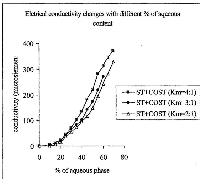
Figure 5.1: Electrical conductivity as a function of water content (System A)
