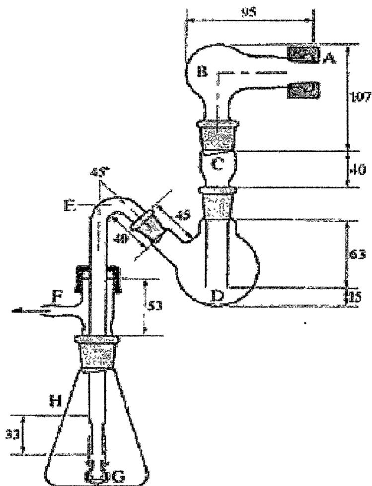
**Figure 5.7 Schematic of the apparatus showing the standard glass twin stage impinger.**
