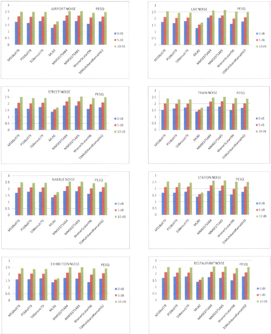
Fig. 4.10 PESQ comparison of STSA algorithms over NOIZEUS database
