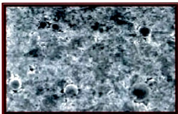
**Fig. 3.1.13 : Scanning electron microphotograph of membrane containing 12% w/w of HPMC K4M (3000 X)**
