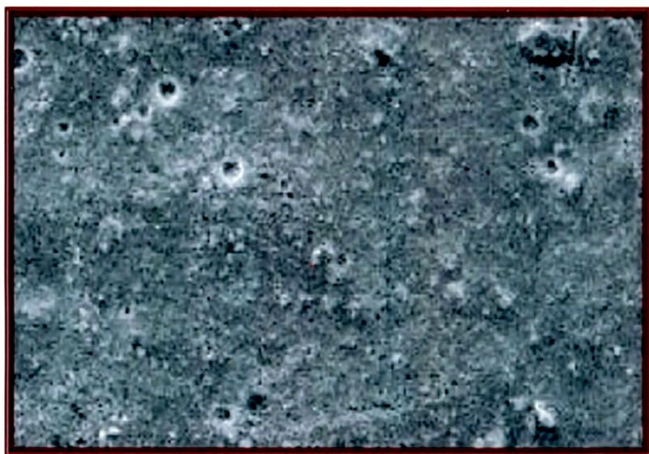
**Fig. 3.1.9 : Scanning electron microphotograph of membrane containing 6% w/w of HPMC K100LV (3000 X)**
