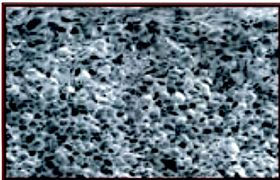
**Fig. 3.1.11 : Scanning electron microphotograph of membrane containing 6% w/w of HPMC K15M (3000 X)**
