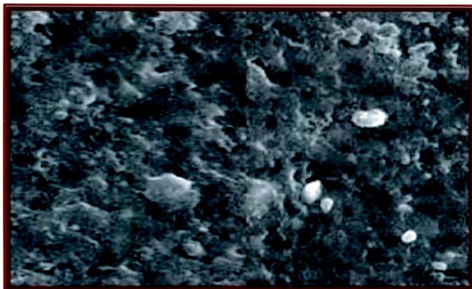
**Fig. 3.2.14 : Scanning electron microphotograph of membrane containing 25% w/w PEG-400 (3000 X)**
