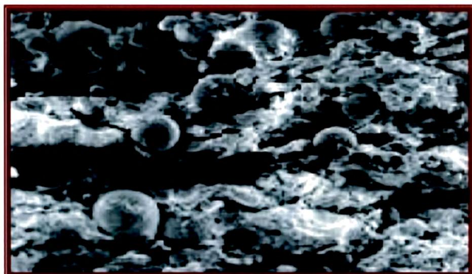
**Fig. 3.3.15 : Scanning electron microphotograph of membrane containing 15% w/w of HPMC (3000 X)**
