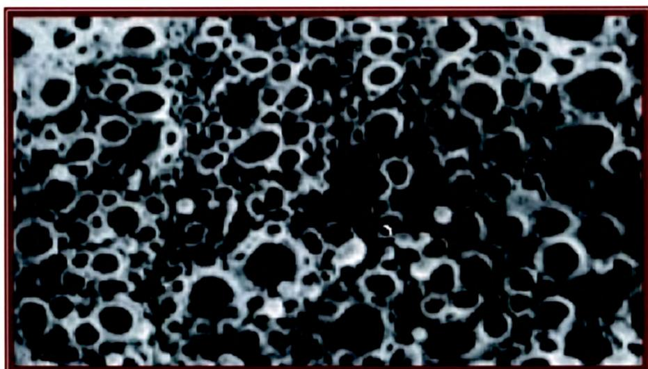
**Fig. 3.3.14 : Scanning electron microphotograph of membrane containing 20% w/w of sorbitol (3000 X)**
