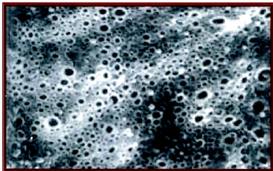
**Fig. 3.3.13 : Scanning electron microphotograph of membrane containing 15% w/w of sorbitol (3000 X)**
