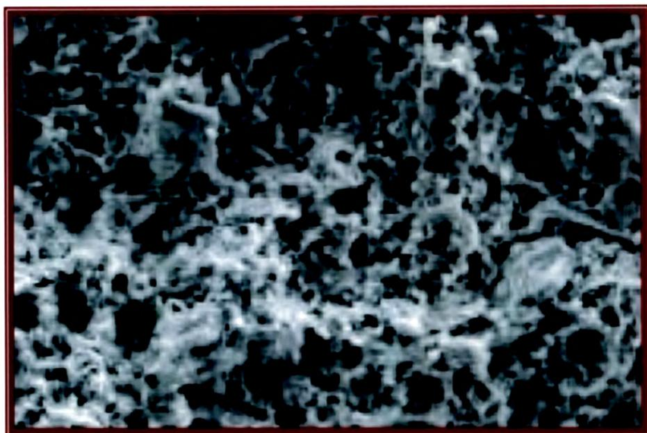
**Fig. 3.3.16 : Scanning electron microphotograph of membrane containing 15% w/w of PEG-6000 (3000 X)**
