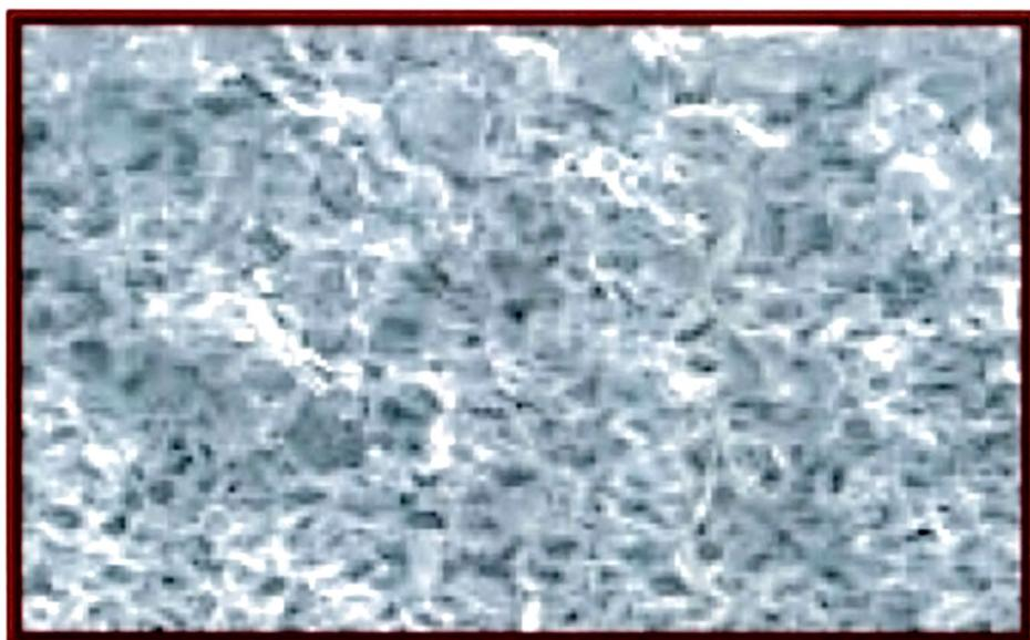
**Fig. 3.1.10 : Scanning electron microphotograph of membrane containing 6% w/w of HPMC K4M (3000 X)**
