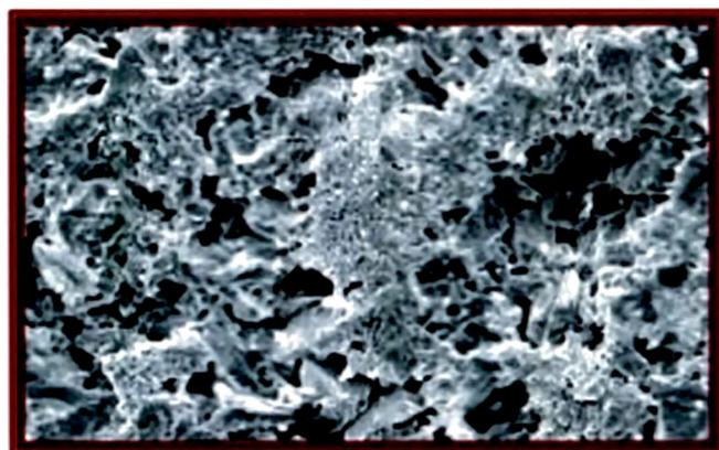
**Fig. 3.1.14 : Scanning electron microphotograph of membrane containing 3.5% w/w each of HPMC K100LV and HPMC K4M (3000 X)**
