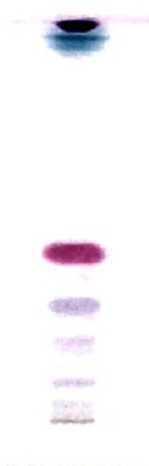
Figure 4.8. Detection of terpenoids in TRFPE on TLC using anisaldehyde sulfuric acid reagent.
