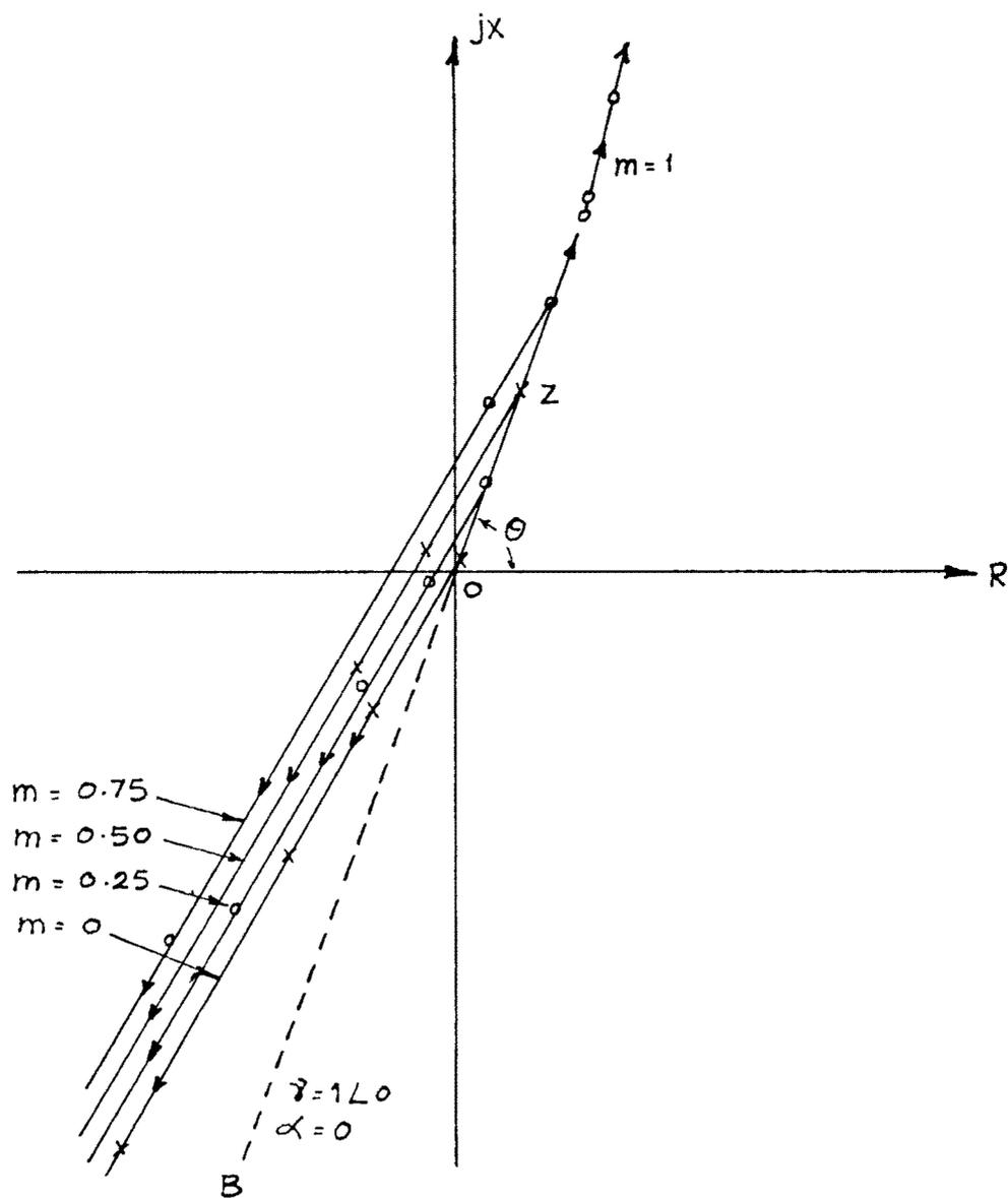
FIG. 9.4 IMPEDANCE LOCI WITH  $\gamma = 0.95 \angle -10^\circ$ ;  $\alpha = 0$
