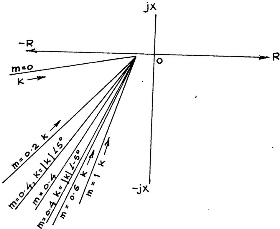
FIG. 9-16 INTERNAL FAULTS ON IMPEDANCE PLANE
