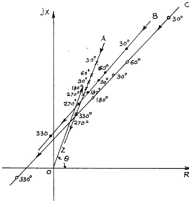
FIG.9-6 POWER SWING LOCI FOR VARIOUS VALUES OF  $\gamma$
