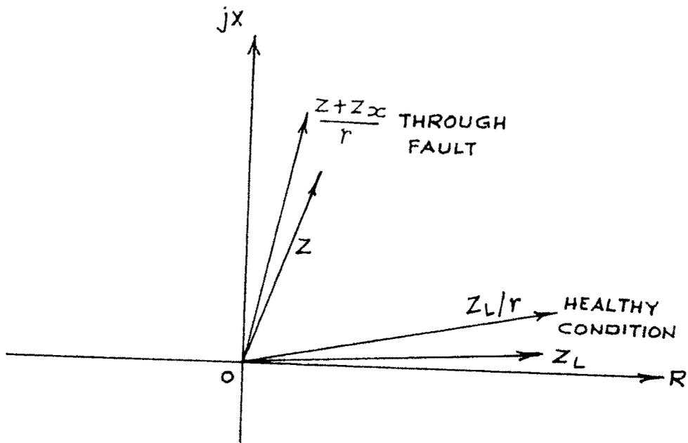
FIG. 9-17 THROUGH FAULT AND HEALTHY CONDITION
