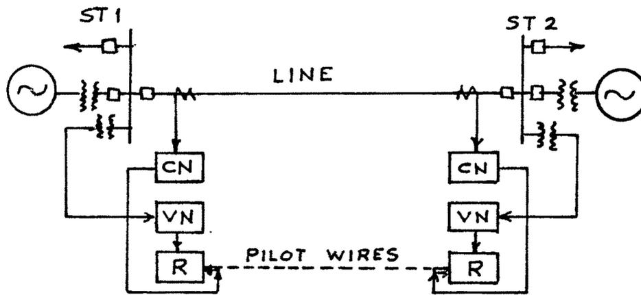
FIG. 9-15 SCHEME OF PROTECTION
