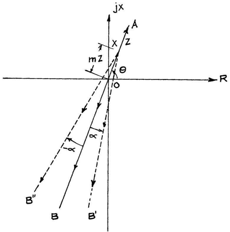
FIG. 9.2 IMPEDANCE LOCI WITH  $k = k_1 \angle \alpha$ ;  $\beta = 1 \angle 0$
