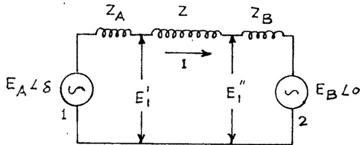
FIG.9-5 A TWO-MACHINE SYSTEM
