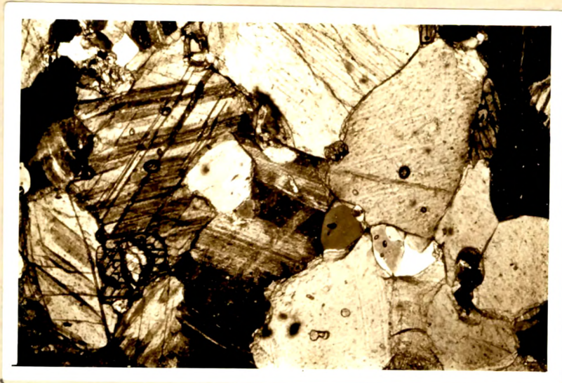
Plate 8.2: Photomicrograph showing granoblastic texture in Marble. (Crossed Nicols, X50)
